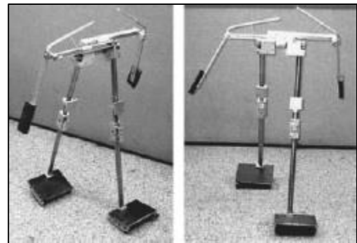
Figure 2-4. Kneed PDW with arms. The arms swung in unison with the contralateral thigh (Collins et al., 2001).
