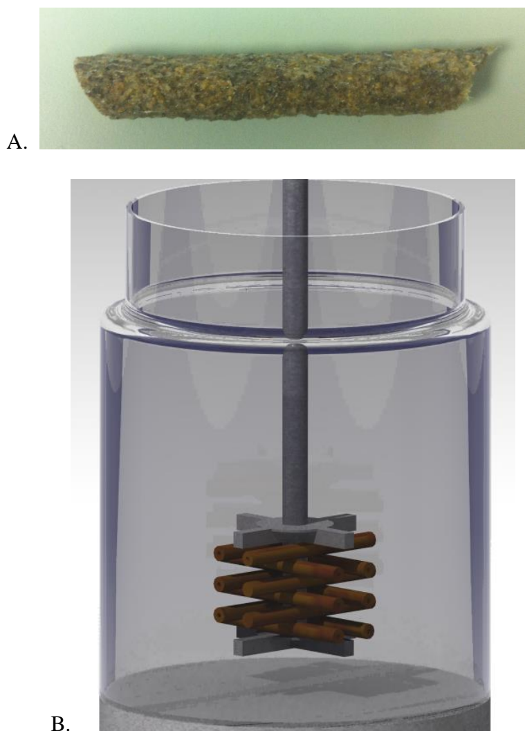
Figure 6.1 Plastic composite support (A), Biofilm reactor set up with plastic composite support (B).
