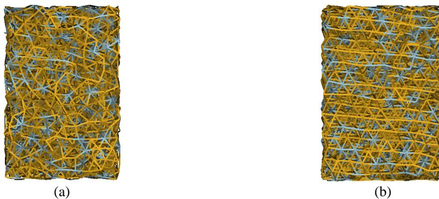
Figure 4-16. Molten Fe matrix ( $28.4 \times 28.4 \times 28.4 \text{ \AA}$ ) structure configuration snapshots before (1701K (a)) and after (1325K (b)) solidification (Fe – orange, Al – grey).
