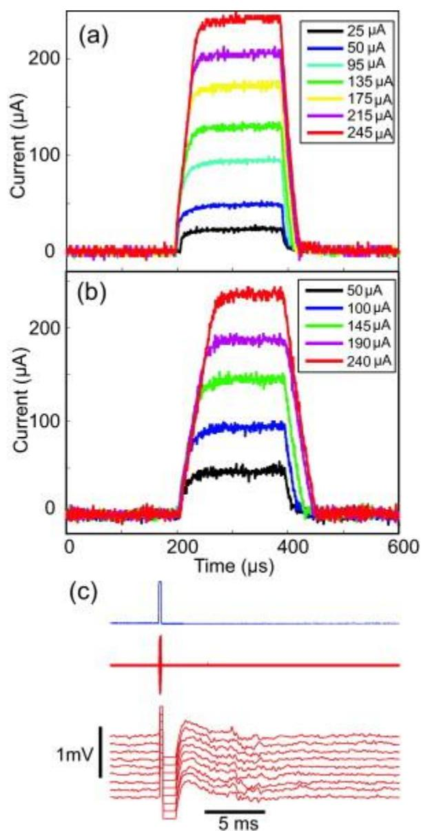
Figure 5-3. Tuning the stimulating current in the current source mode of the device.
