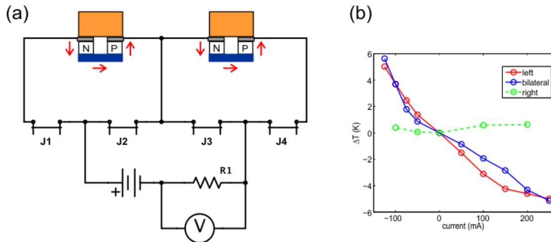
Figure 4-1. Unilateral cooling device
