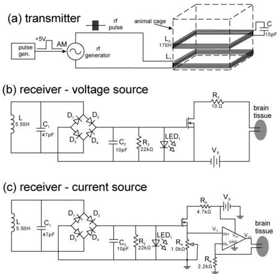
Figure 5-1. Schematic of the wireless stimulation system.
