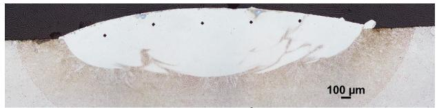
Figure 10 – Single track deposit of SS 431 at 1.0 cm<sup>3</sup>/min powder flow rate and 2 kW laser power.
