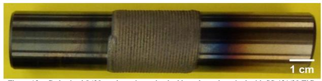
Figure 12 – Carburized 8620 steel specimen that had been laser deposited with SS 431/20 TiC.
