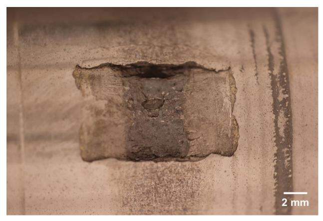
Figure 58 - RCF test results showing surface pitting on the SS 431/20 TiC specimen.
