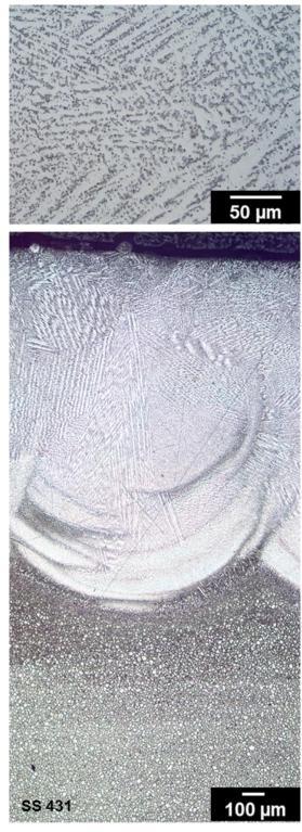
Figure 42 – Microstructures of SS 431 deposited on Inconel 718<sup>®</sup> shaft.
