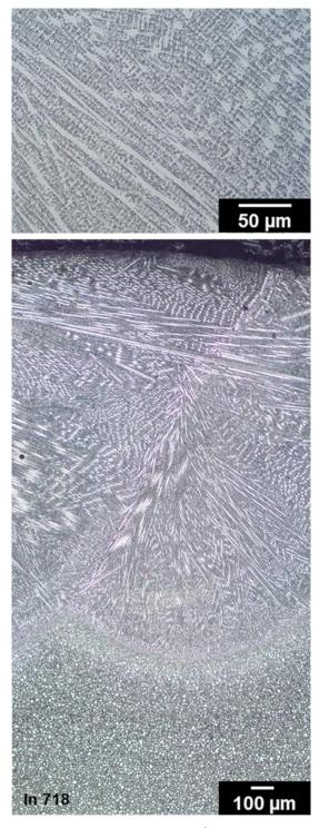
Figure 41 - Microstructures of Inconel  $718^{\text{@}}$  deposited on Inconel  $718^{\text{@}}$  shaft.
