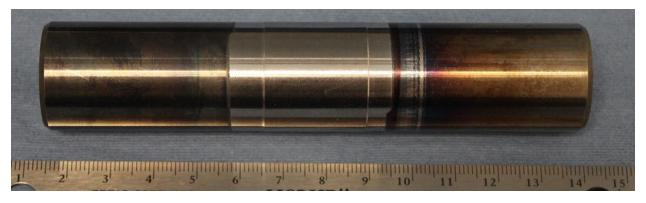
Figure 14 – The RCF test specimen with laser deposited SS 431/20 TiC (scale in cm).
