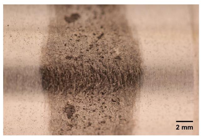
Figure 56 - RCF test results showing scuffing surface on the SS 431/20 TiC.
