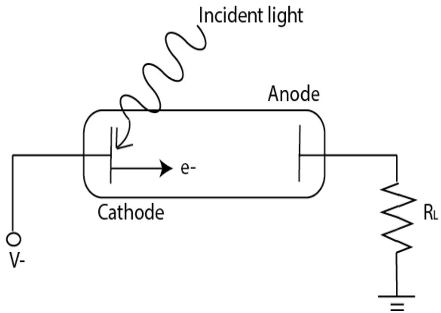
Fig. 2-2. Photo emissive detector.
