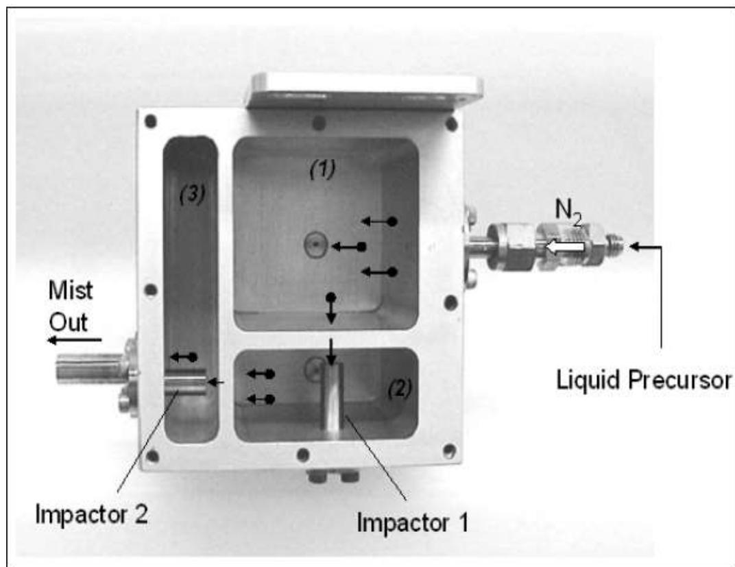
Fig. 2-12. Internal structure of atomizer [26].
