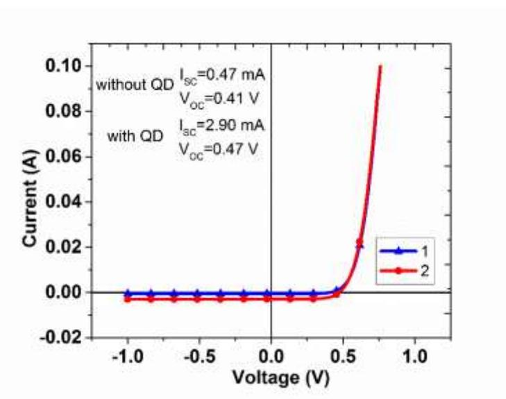
Fig. 5-5. (a) Plot of dark (1) and light (2,3) current-voltage characteristics of the photodiode at 405 nm before (2) and after 40 nm thick layer of QD (3) on log scale. (b) Same plot on linear scale showing current-voltage characteristics of photodiode before (1) and after 40 nm thick layer of QD (2).
