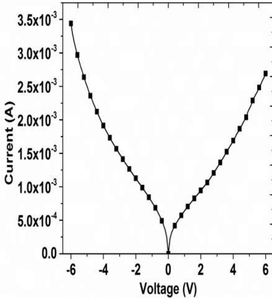
Fig. 5-2. Current-voltage characteristics of T21&T22 on back side of wafer.
