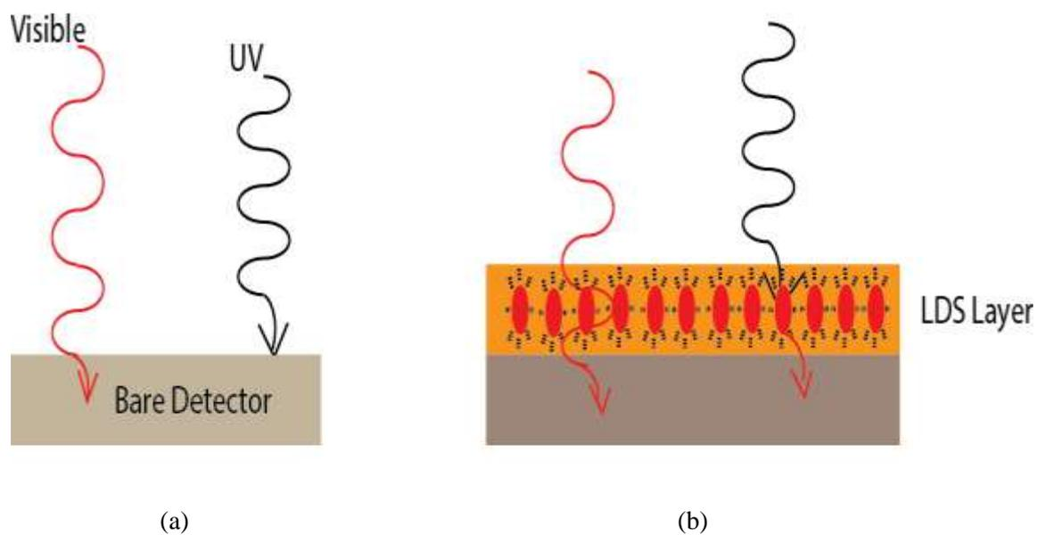
Fig. 2-6. Sketch of quantum dot sensitized UV detector. (a) Visible light (red curved line) is collected in the active region, UV light (black curved line) is collected near the surface of the bare detector. (b) UV light is absorbed by red quantum dots and re-emitted in the visible region.
