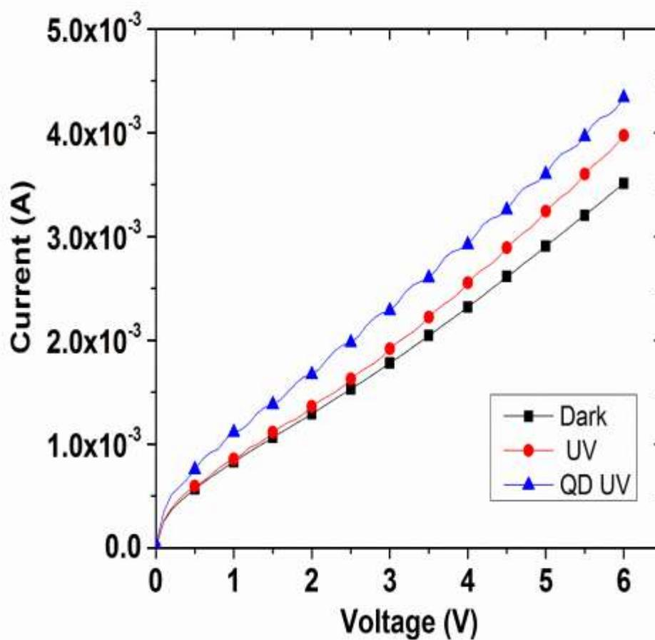
Fig. 5-3. Current-voltage characteristics of T21&T22 under dark and UV light.
