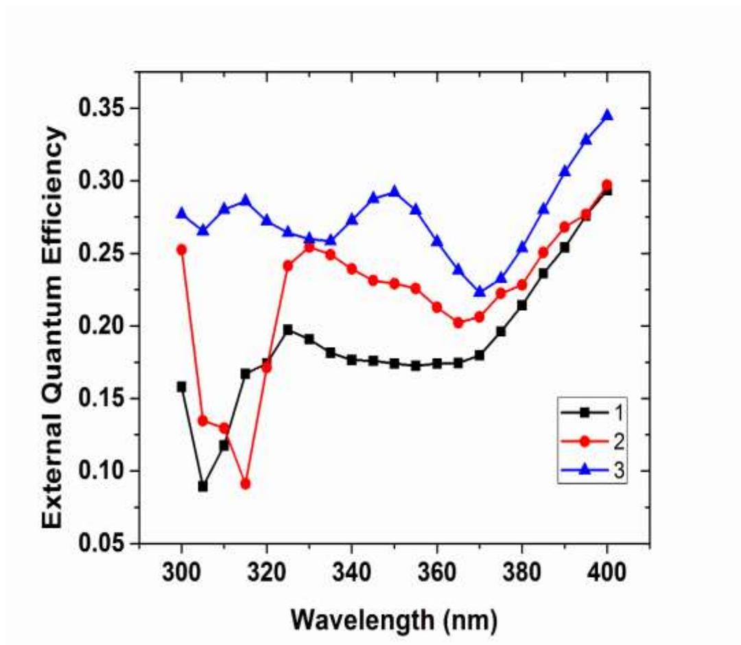
Fig. 5-6. EQE of silicon planar photodiode before (1) and after (2,3) CdSe/ZnS quantum dots- 20 nm deposition (2), 40 nm deposition (3).
