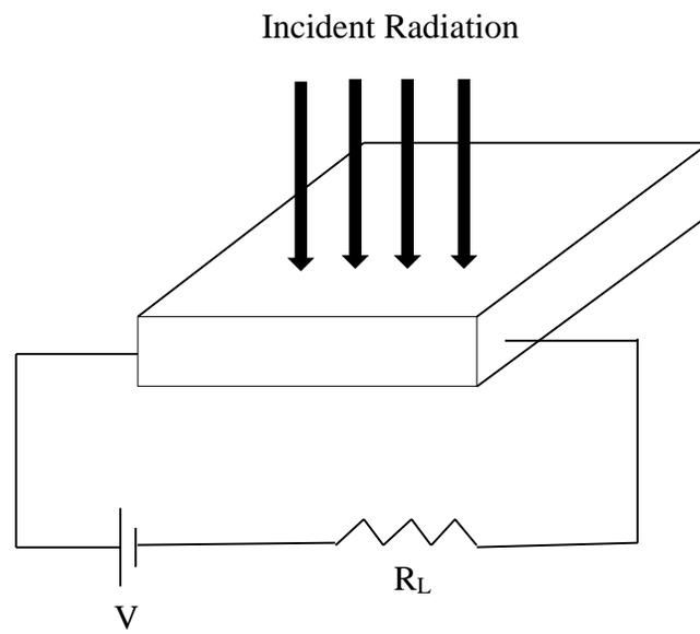
Fig. 2-3. Illustration showing photo conductive detector.
