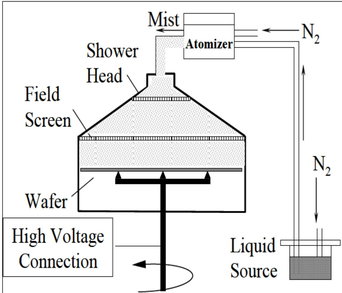
Fig. 2-11. Schematic of mist deposition system [30].
