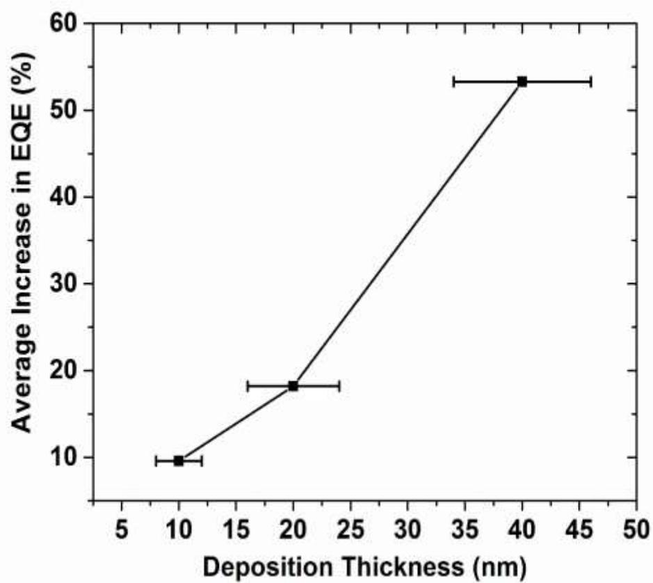
Fig. 5-7. Average increase in EQE with deposition thickness.
