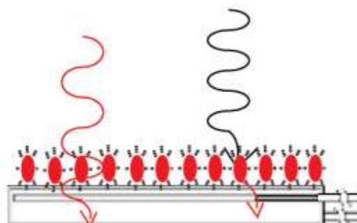
Fig. 4-2. Sketch of quantum dot sensitized UV detector. (a) Silicon planar photodiode from Silonex Inc. used in this study. (b) Visible light (red curved line) is collected in the active region, UV light (black curved line) is collected near the surface of the bare detector. (c) UV light is absorbed by red quantum dots and re-emitted in the visible region.
