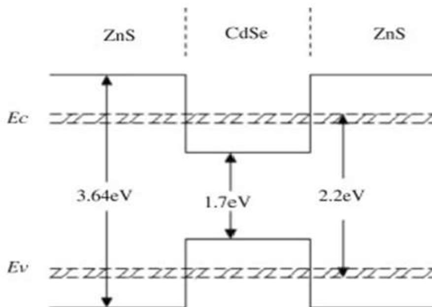
Fig. 2-7. (a) Illustration of CdSe core and CdSe/ZnS core-shell quantum dot. (b) Band diagram of CdSe/ZnS core-shell quantum dot [22].
