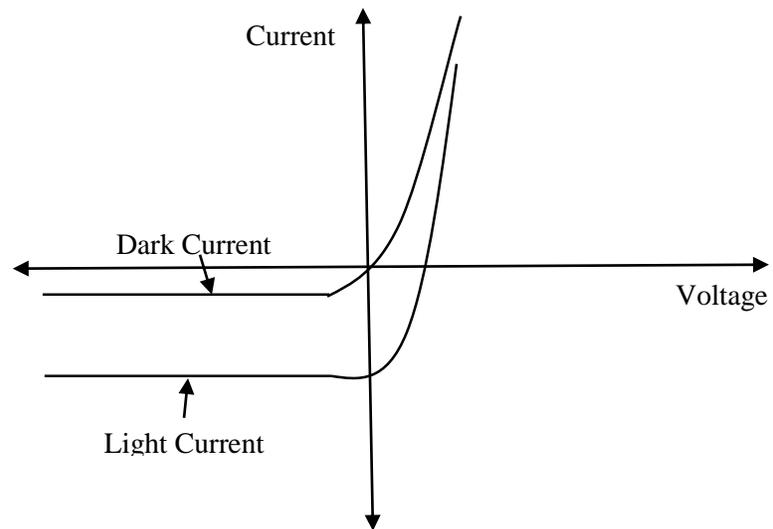
Fig. 2-5. (a) Equivalent circuit of an illuminated photodiode. (b) Current-voltage characteristics of an illuminated and non-illuminated photodiode.
