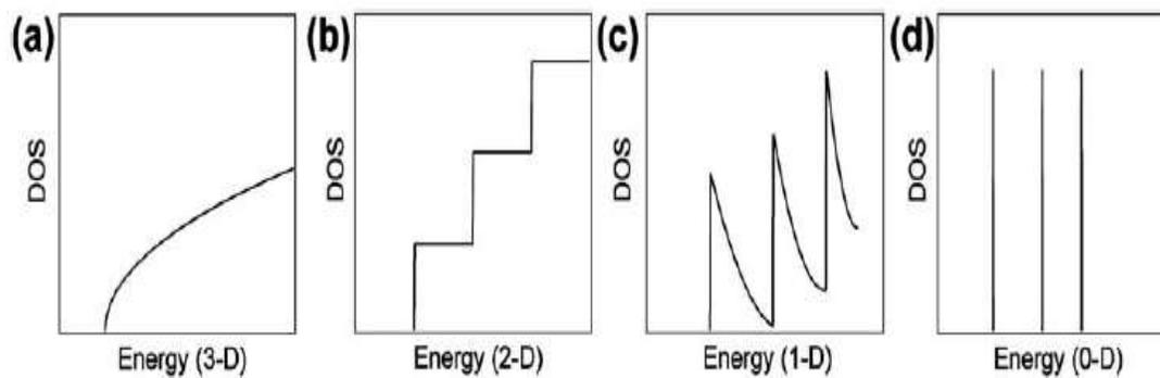
Fig. 2-8 Schematic illustration of the density of states as a function of energy for: (a) a bulk material (3-D), (b) a quantum well (2-D), (c) a quantum wire (1-D), (d) a quantum dot (0D) [23].
