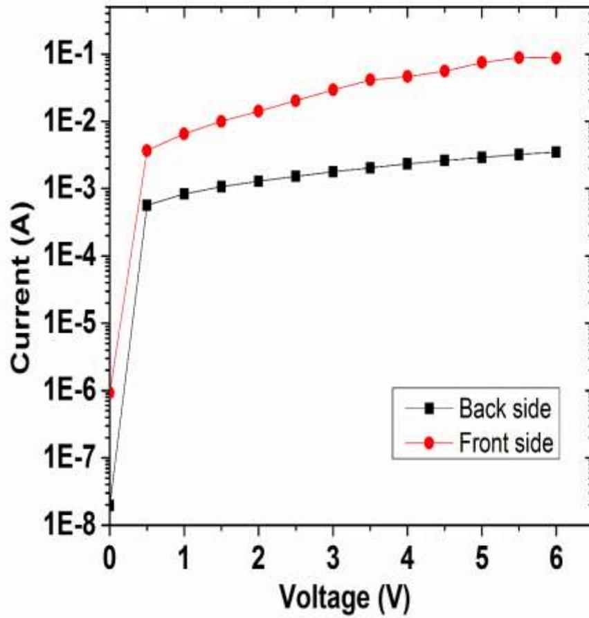
Fig. 5-4. Current-voltage comparison of front and back side of silicon wafer.
