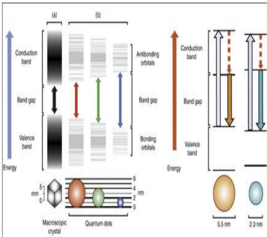
Fig. 2-9. Illustration showing variation of band gap with size [27].
