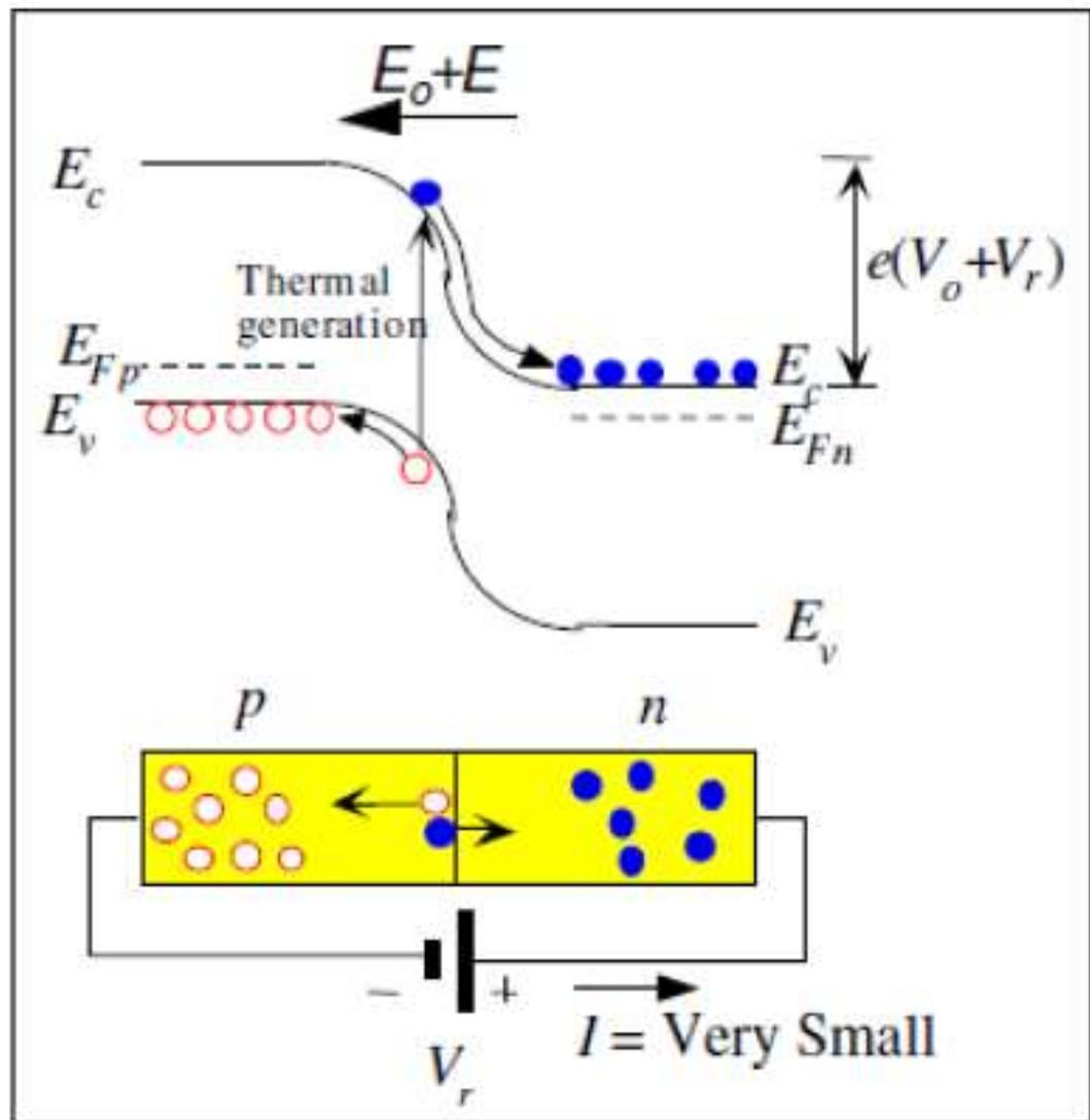
Fig. 2-4. Band diagram of a p-n homo junction photo diode, and its operation [14].
