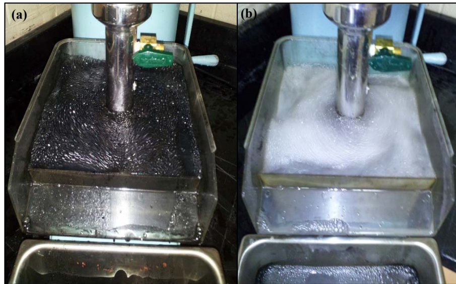
Figure 6.2. Ultimate recovery flotation before (a) and after (b) froth scraping
