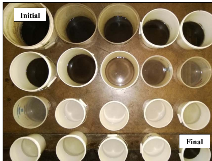
Figure 7.2. Filtrate opacity with cycle progression (final bucket represents air blow liquid)
