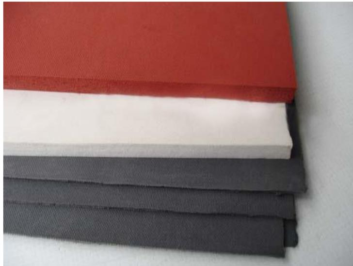
Figure 3-7. Closed-cell silicone foam [35]
