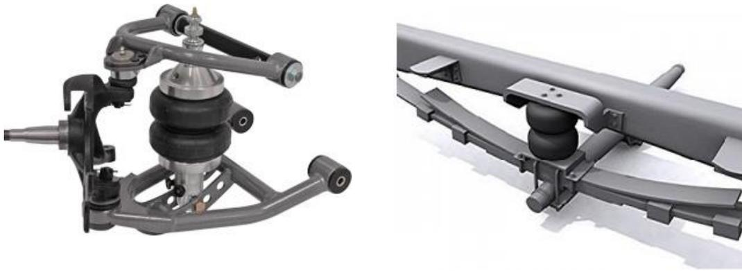
Figure 1-6. Pneumatic isolator vehicle suspension systems [15, 16]
