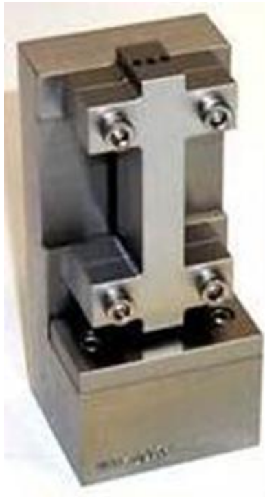
Figure 2-2: SACMA SRM 1R-94 end-loaded compression test fixture [26]
