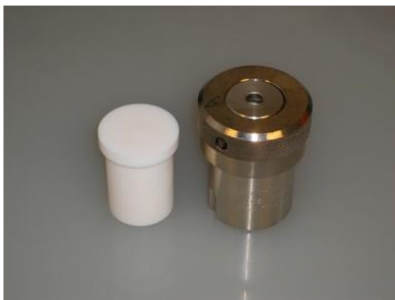
Figure 1-9 Hydrothermal/solvothermal methods are conducted in ovens. A Teflon reactor which contains precursor solution and substrates is sealed in a metal bomb.
