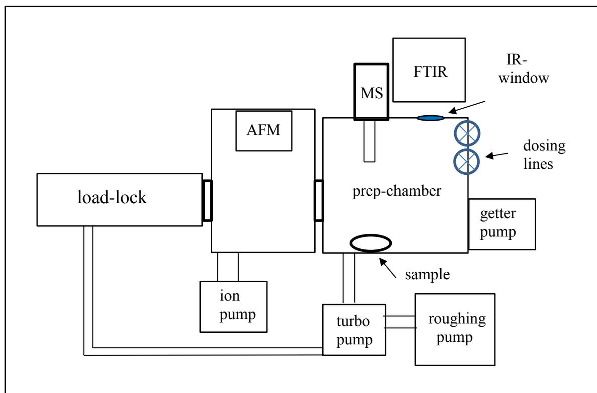
**Figure 7.** Schematic of the Ultra High Vacuum instrument.
