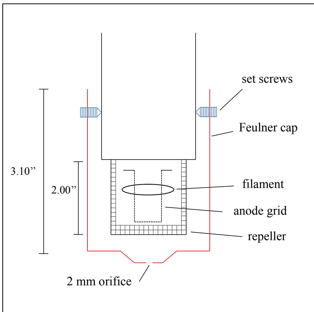
**Figure 9.** The schematic of the Feulner cap which houses the filament of the mass spectrometer. The 2 mm orifice of the cap is placed close to the sample for the detection of desorbing molecules.
