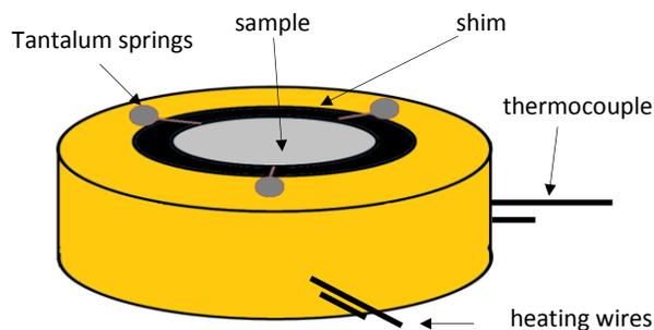
**Figure 8.** Schematic of the sample mount.
