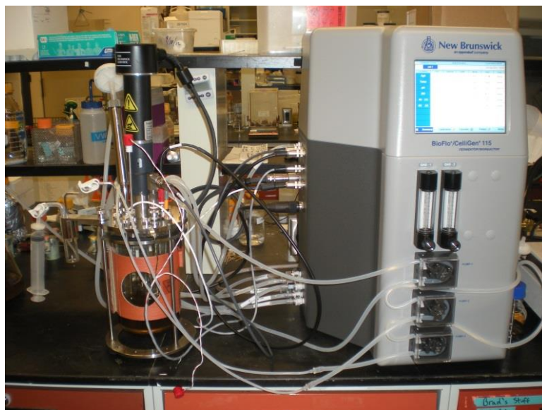
Figure 2-3: The automated control unit on the right regulates all of the operating conditions set in the reactor on the left.
