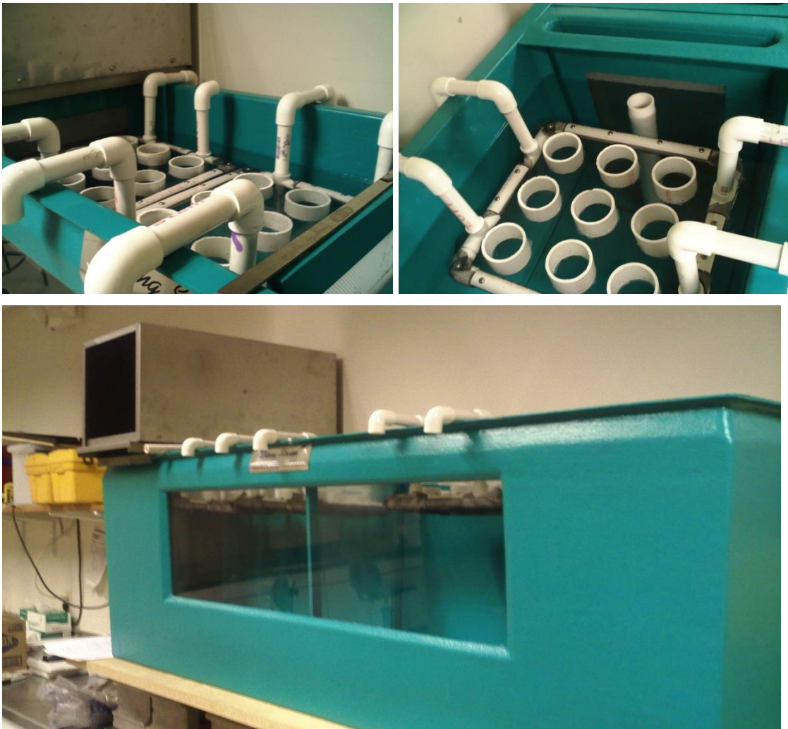
Figure B-1: Egg Trays in Living Streams. In 2010, egg trays were partially submerged in the tank, as shown above. The cups were not fully submerged to prevent fry from escaping their cup.
