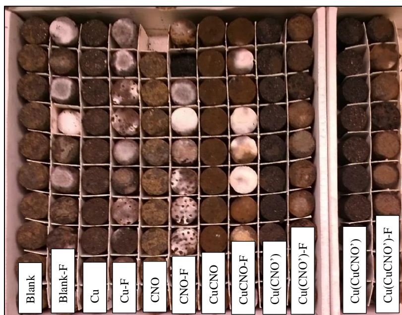
Figure 4-10. Lab-scale briquettes following 21 day incubation at 30 °C and 100% humidity reveals fungal growth on all briquettes with (A) minimal growth on some and (B) extensive growth on others. Fungicides were applied internally to briquette batches unless otherwise noted. Cu=Copper; CNO=Clarified Neem Oil; CNO'=External CNO Fungicide; F=Fungus applied.
