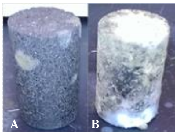
Figure 4-11. Lab-scale briquettes following 21 day incubation at 30 °C and 100% humidity reveals significant difference in the amount of fungal growth observed: (A) minimal growth on some non-inoculated bricks (B) extensive growth on some inoculated bricks.
