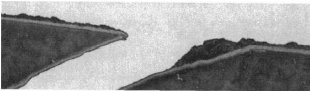
**Figure 2-1. A micrograph of a blocked film cooling hole [6].**
