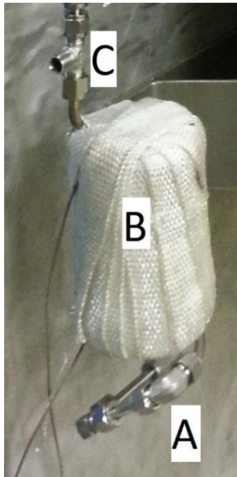
Figure 2.6: The first revision of the steam generation system showing the water inlet (A), heated coil (B), and thermocouple port and steam outlet (C)
