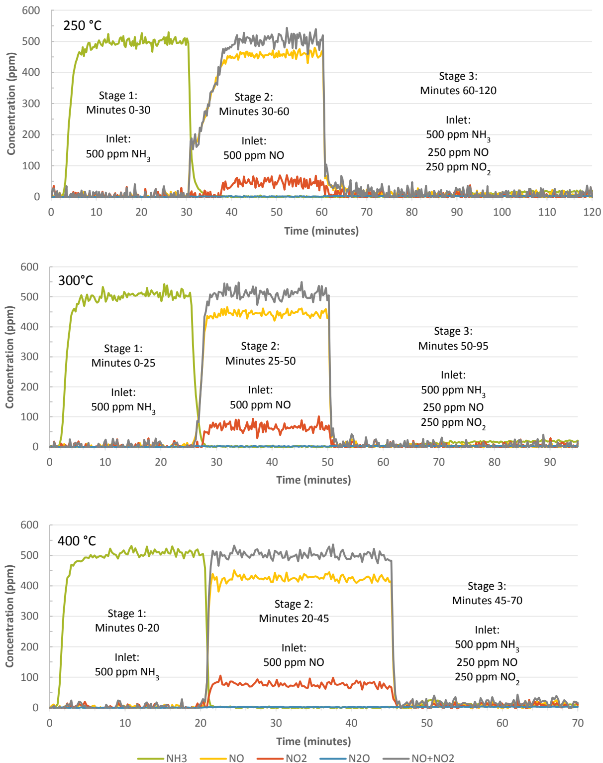
Figure 4.1: Performance of the new catalyst monolith at 250, 300, and 400 °C.
