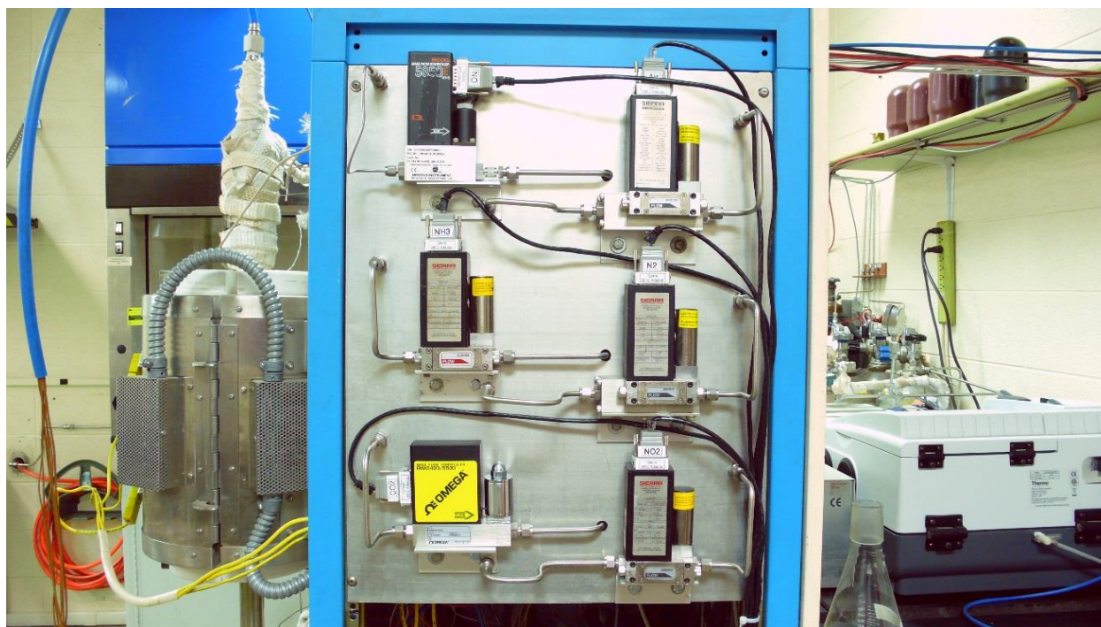
Figure 2.3: The mass flow controller system showing the six primary MFCs. Not shown are a MFC controlling the flow rate of the nitrogen carrier gas for steam and a MFC controlling the nitrogen purge for the FT-IR spectrometer.
