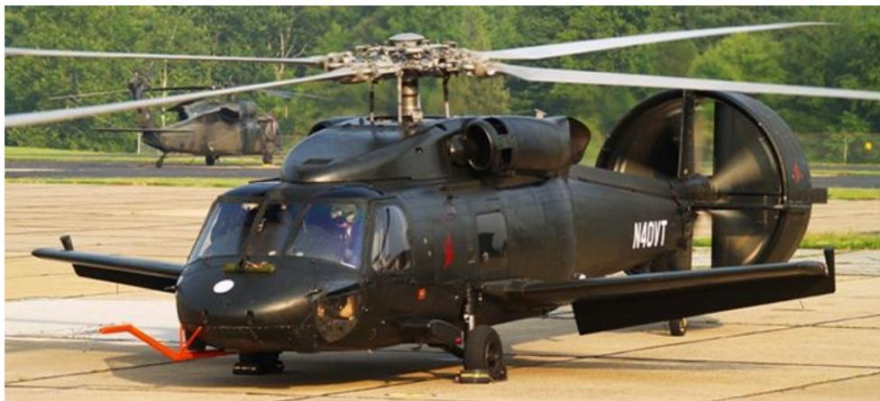
Figure 2-4: Piasecki X-49A SpeedHawk VTDP Technology Demonstrator
