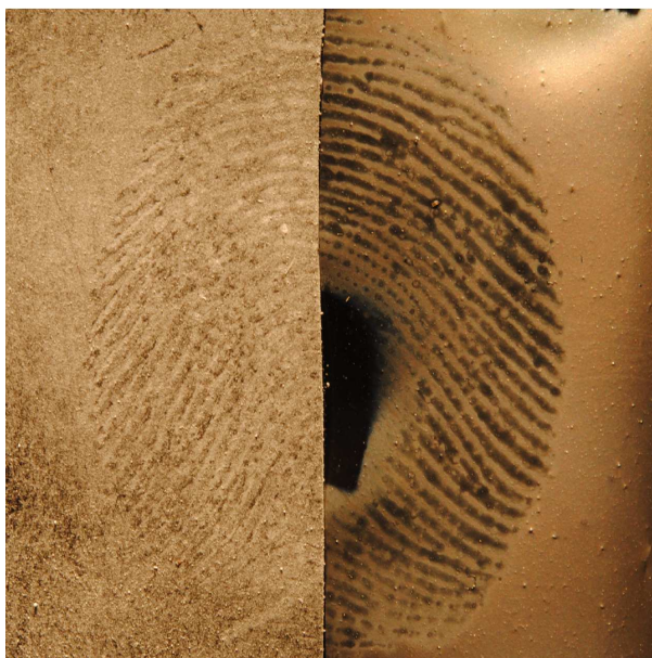
Figure 3.10: Fingerprint on a black garbage bag (soft plastic) developed either (left) by the use of white magnetic powder or (right) by the deposition of a 100-nm-thick CTF of nickel. Level three detail is clearly seen in the CTF-developed fingerprint. [Courtesy of Sarah Muhlberger]
