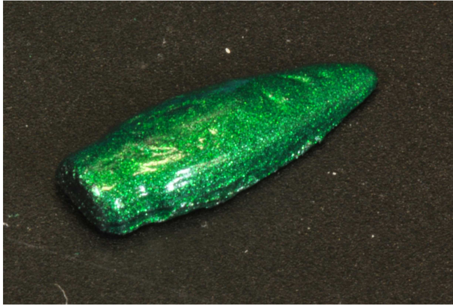
Figure 2.13: The unpainted decoy after being smoothed with acetone and then painted with metallic emerald paint.
