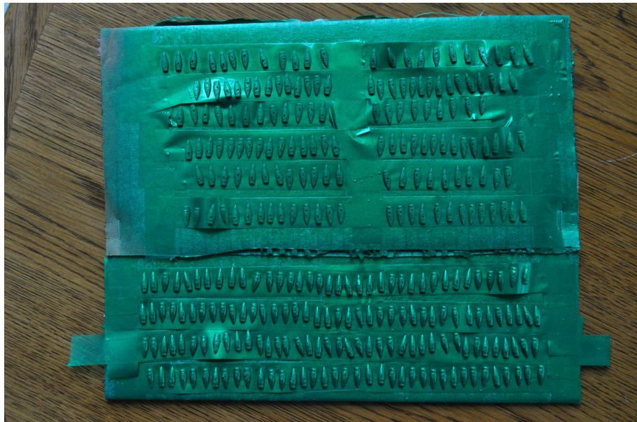
Figure 2.13: The unpainted decoy after being smoothed with acetone and then painted with metallic emerald paint.
