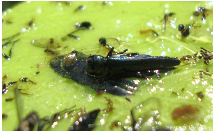
Figure 2.8: Photograph of a test trap with an Agrilus male stuck to a visual decoy, thereby demonstrating that the visual decoys produced by us can initiate pouncing behavior. Field tests were conducted in Hungary. [Courtesy of Dr. Thomas Baker and Dr. Michael Domingue]
