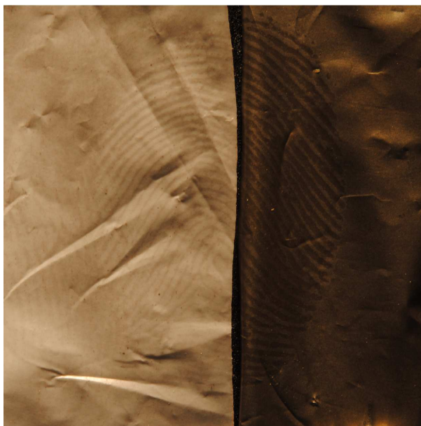
Figure 3.11: Fingerprint on a clear sandwich bag (soft plastic) developed either (left) by the use of cyanoacrylate fuming or (right) by the deposition of a 50-nm-thick CTF of gold. Level three detail is clearly seen in the CTF-developed fingerprint. [Courtesy of Sarah Muhlberger]
