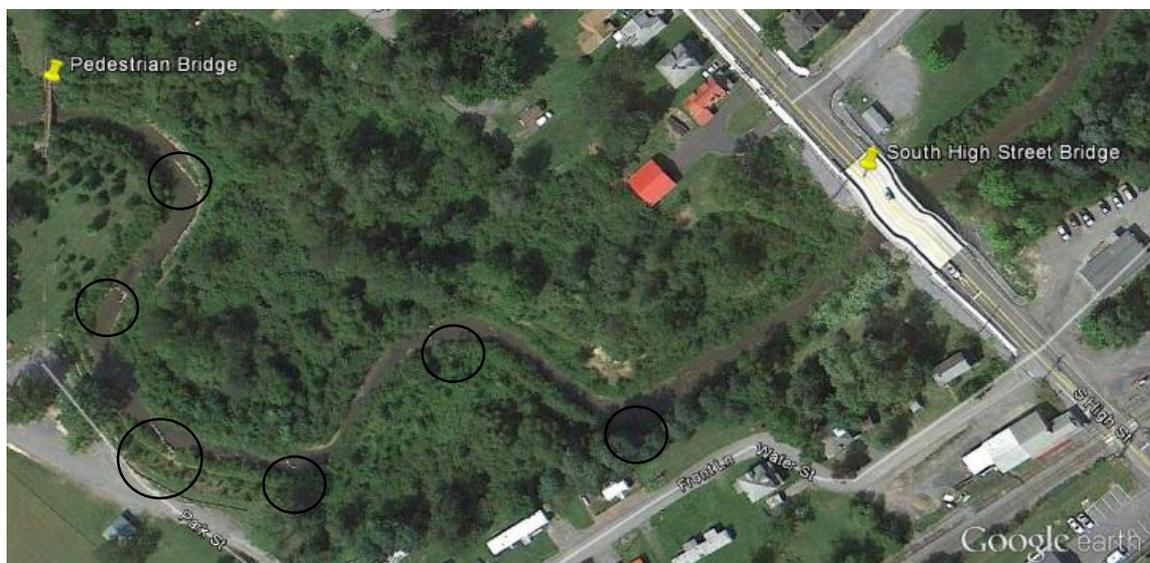
Figure 4-6: Aerial view of Bald Eagle Creek project reach evaluated in this case study (Google earth, 2012b). The black circles indicate the location of the J-Hook structures. Flow proceeds from the pedestrian bridge (west) toward the South Higher Street Bridge (east).
