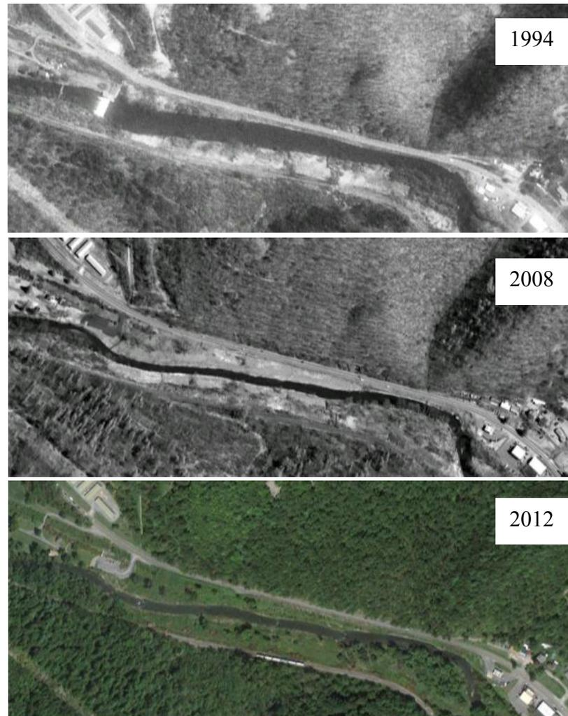
Figure 4-16: Historic photographs of the McCoy Linn Dam (top), the post-dam removal but pre-modified channel (middle), and the modified channel. Images from Google earth (2012c, 2008, 1994).
