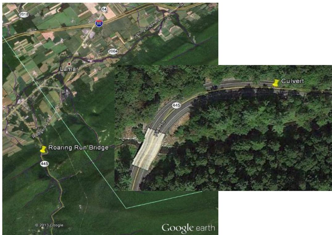
Figure 4-1: PA State Route 445 over Roaring Run. Aerial Photograph of Roaring Run at bridge crossing and culvert location in abandoned channel. Images from Google earth (2012a). Flow direction is east, left to right in the above images.
