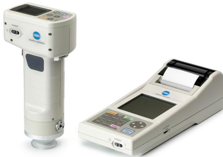
Figure 4.3. Minolta Chromo Meter CR 200 (Minolta Inc., Ramsey, NJ).
