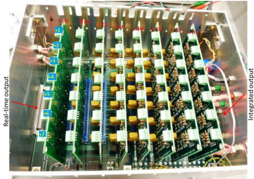
Channel/board mapping to PCI-6071E connector pin-out (use this to program in any order for data acquisition)
