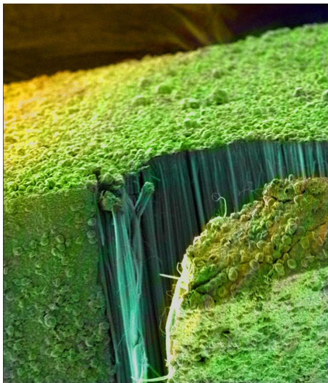
Figure 2.3: SEM image of PEDOT-ACNT forest morphology (colorized with Adobe photoshop)
