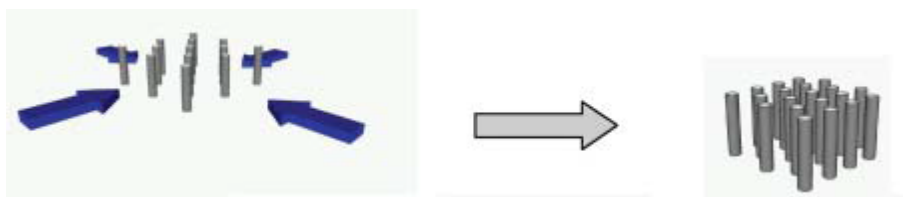
Figure 2.4: Biaxial mechanical densification of ACNT arrays [13]
