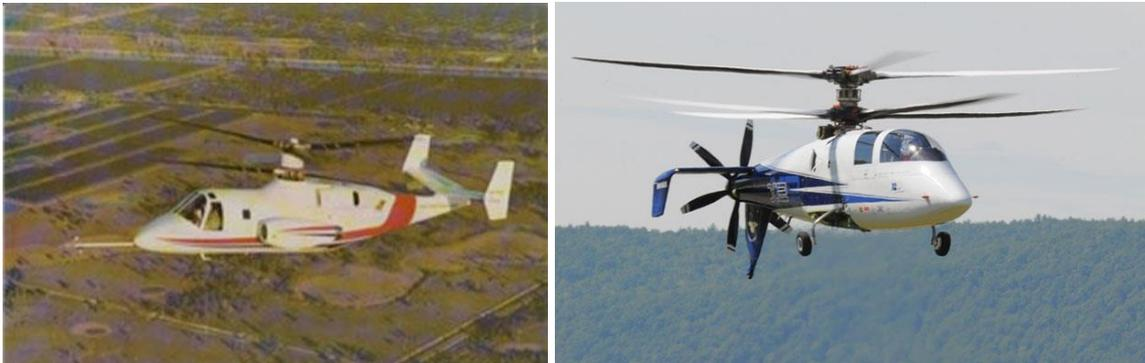
Figure 1-3. Advancing Blade Concept Examples (Left: Technology Demonstrator XH-59A, Right: Sikorsky X-2)
