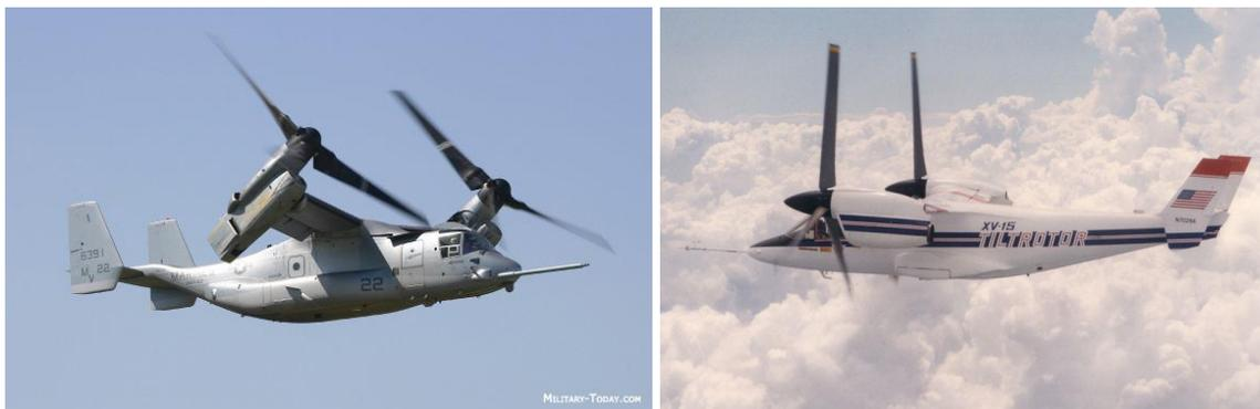
Figure 1-4. Tiltrotor helicopter (Left: Bell-Boeing V-22 Osprey, Right: Bell XV-15)
