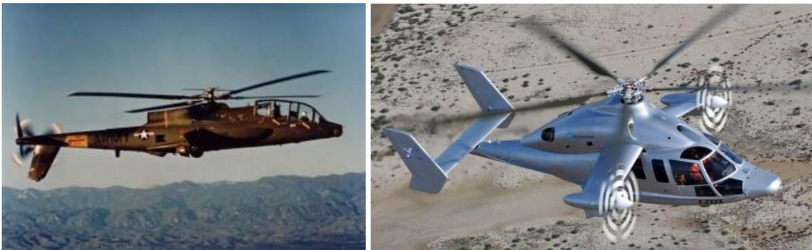
Figure 1-2. Compound helicopter examples (Left: Lockheed AH-56 Cheyenne, Right: Eurocopter X3).
