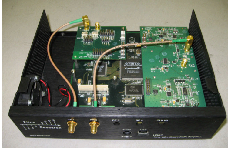
Figure 2.5: The Ettus Research USRP1 device, fitted with a BasicRX daughterboard (left side) and an RFX-400 daughterboard (right side).
