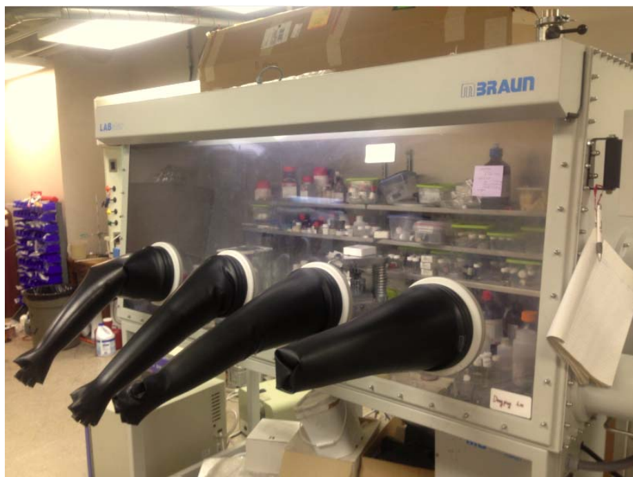
Figure 2-2. Glove box for assembling 2016 type coin cell
