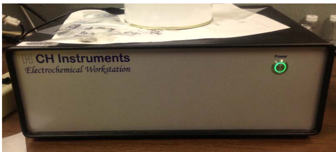
Figure 2-4. CHI electrochemical workstation used for cyclic voltammetry test.
