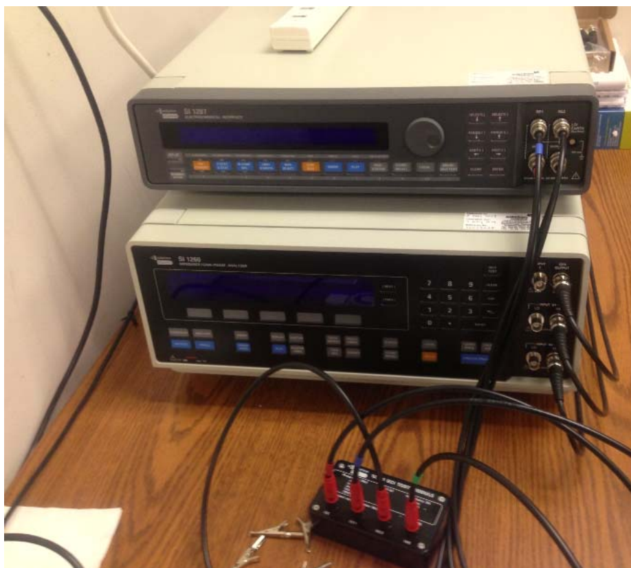
Figure 2-5. Solartron AC impedance tester
