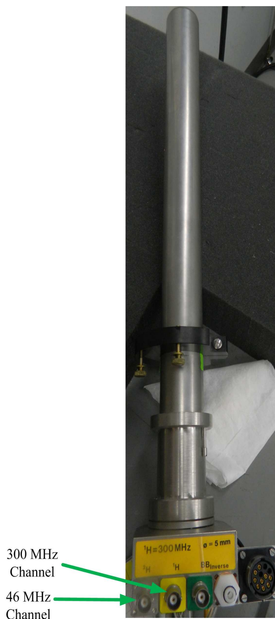
Figure 3.9. Photograph of the Bruker probe used for NMR measurements.
