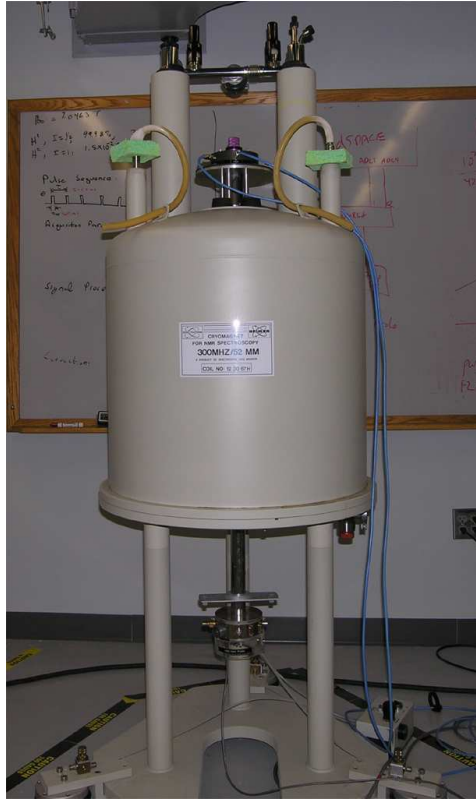
Figure 1.1. Photograph of the 7.1 T superconducting magnet used to develop and test feedback compensators for reducing field fluctuations.
