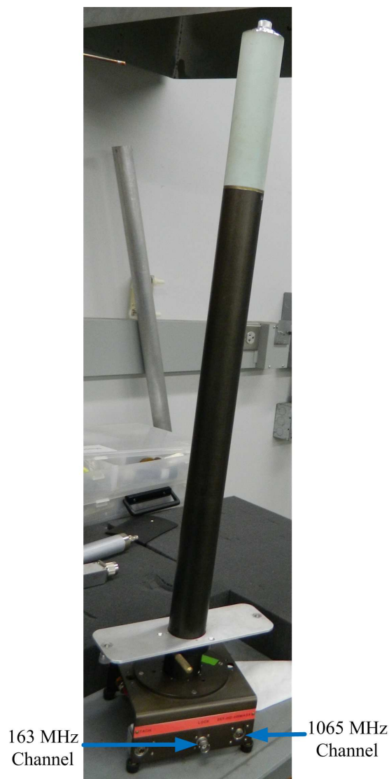
Figure 3.8. Photograph of the HR-MAS probe used for NMR measurements.
