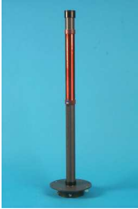
Figure 2.3. Drive coil assembly, including disturbance and correction coils.
