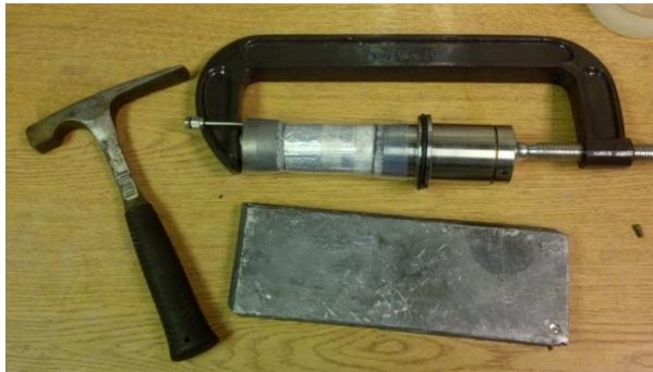
Figure 3-3. Manual stimulation using pick hammer with sample confined in a C- clamp
