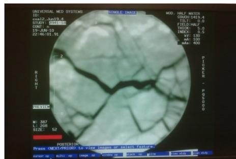
Figure 3-2. X-ray CT image of sample at a particular location in the sample in the axial direction
