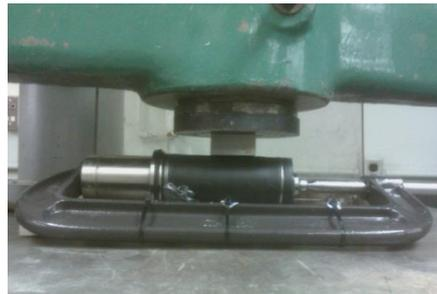
Figure 3-1. Compressive loading on the sample in a Brazilian tensile strength testing machine
