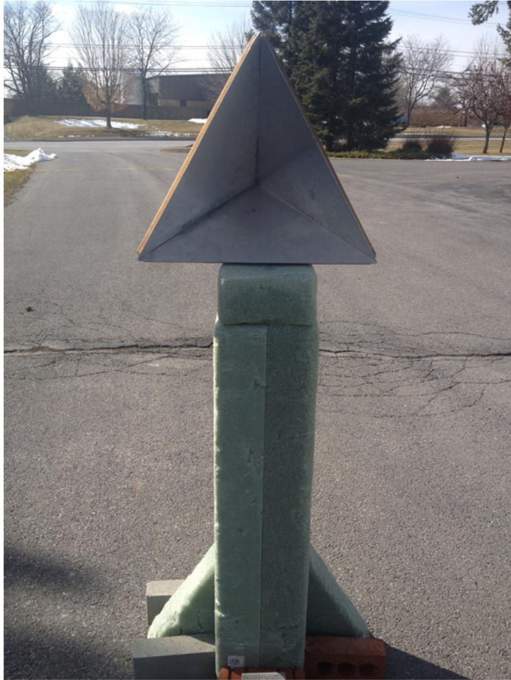
Figure 2.11: Close-up photograph of the corner reflector target.
