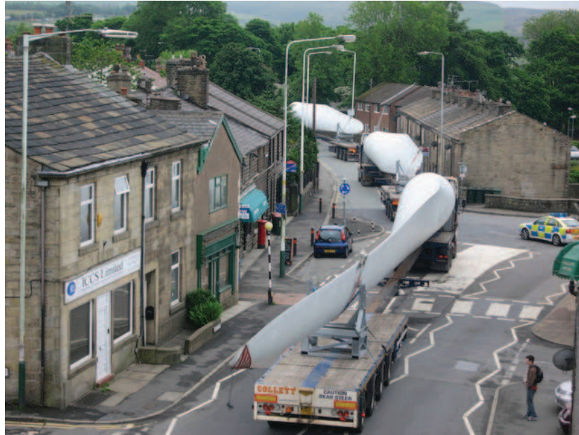
Figure 3: TRANSPORTATION OF WIND TURBINE BLADES
