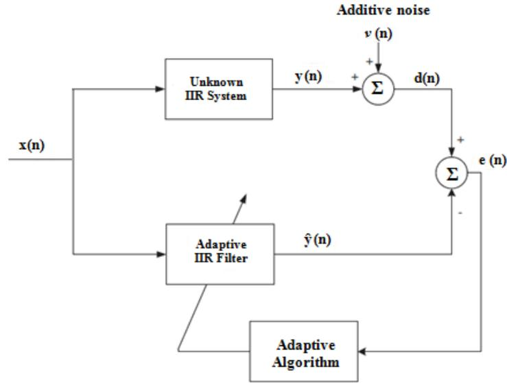
Figure 1-1 IIR System Identification Block Diagram
