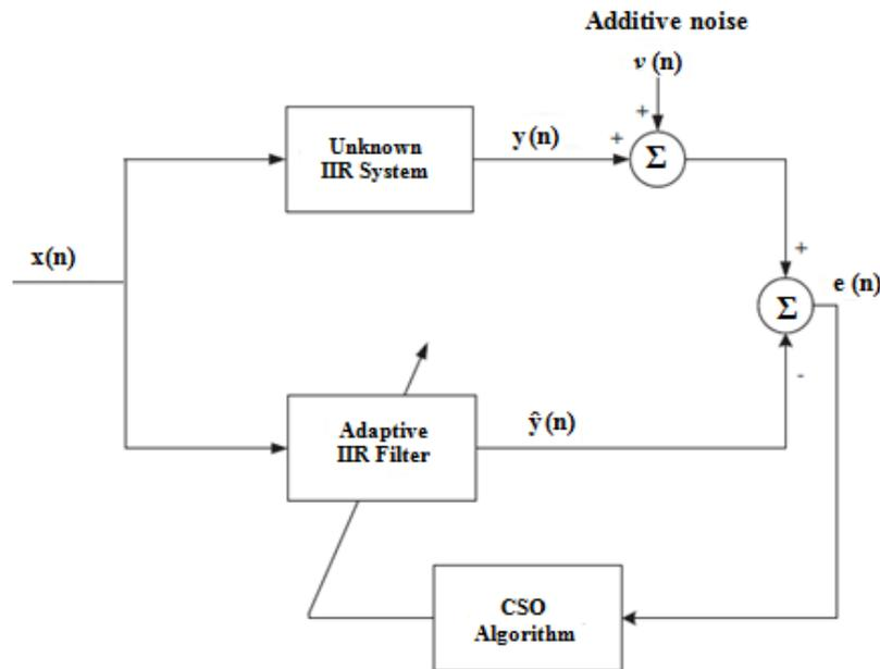
Figure 2-3 Block Diagram of CSO based IIR System Identification
