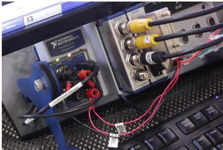
Figure A.2: Close-up of NI data acquisition assembly. Note: Chassis PFI0 outputs trigger and chassis PFI1 outputs pulsetrain (dictates sampling rate), both of which are collected by NI-9411. The NI-9411 also receives differentially encoded digital data from the rotary encoder ( D_{DC} ). Channels 0/1/2 on the NI-9215 receive -10 to +10V analog signals carrying data regarding F_p/F_q/D_{AC} , respectively.
