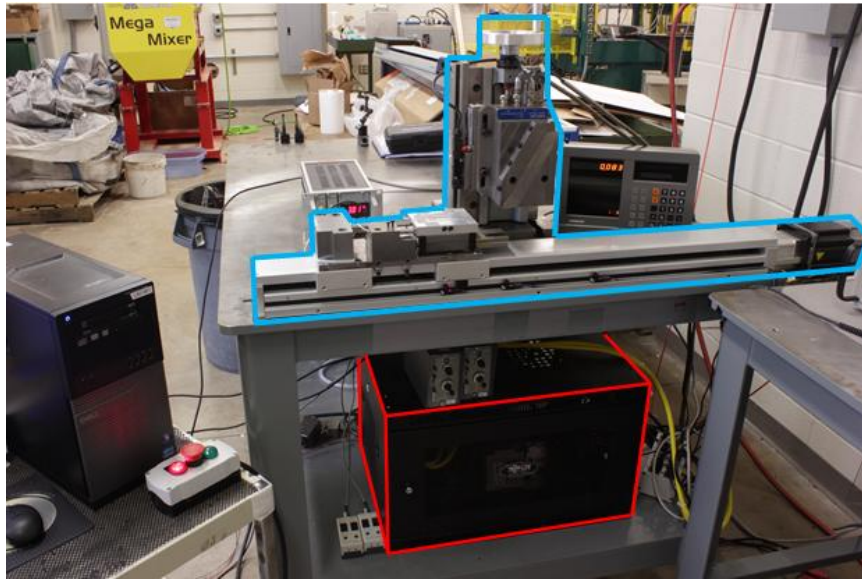
Figure A.3: Table holding planer assembly mechanical components (outlined in blue, top) and controller housing (outlined in red, bottom)
