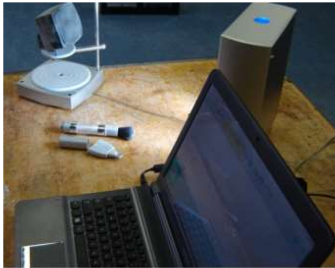
Figure 3-2: Setup of 3D scanner capturing the digital representation of a physical artifact (speaker system) [56].
