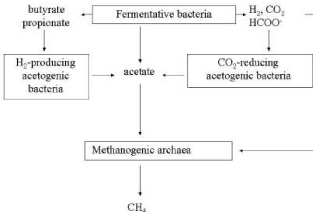
Figure 1-2: Four interacting metabolic groups of anaerobic microorganisms involved in the complete decomposition of organic matter.
