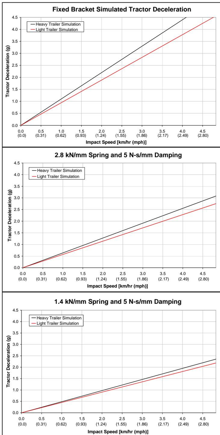
**Figure 4.8: Coupling tractor decelerations**
