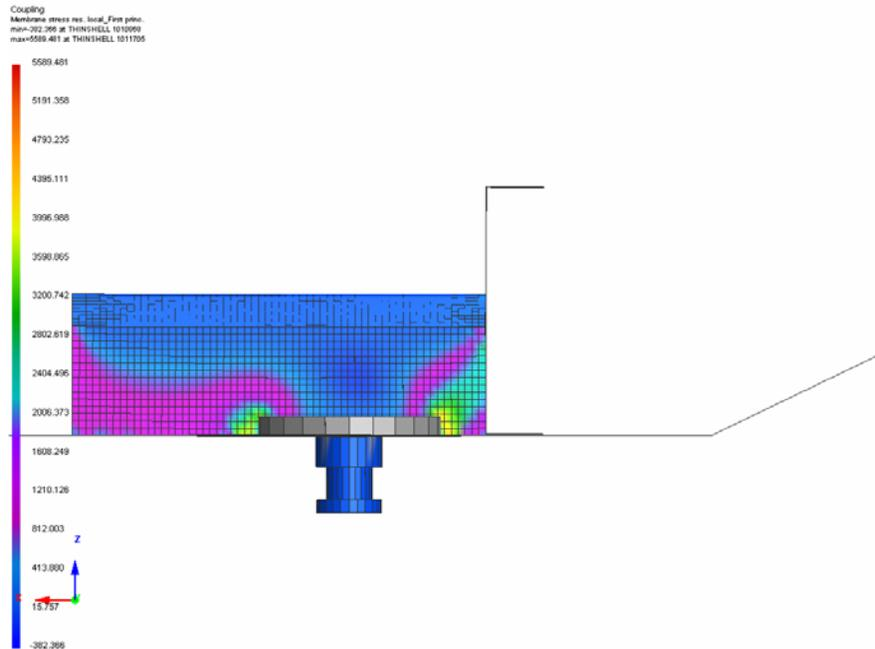
**Figure 5.14: Side view of Von Mises stress plot from the downward load “E”**
