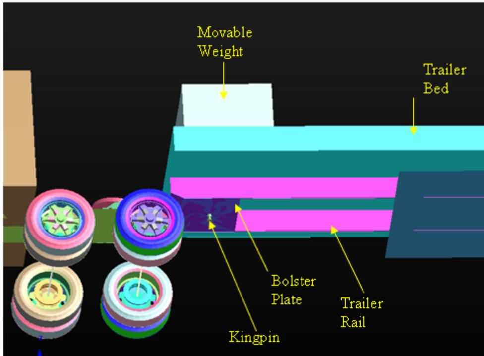
**Figure 2.13: Bottom view of Mack Trucks' trailer model**
