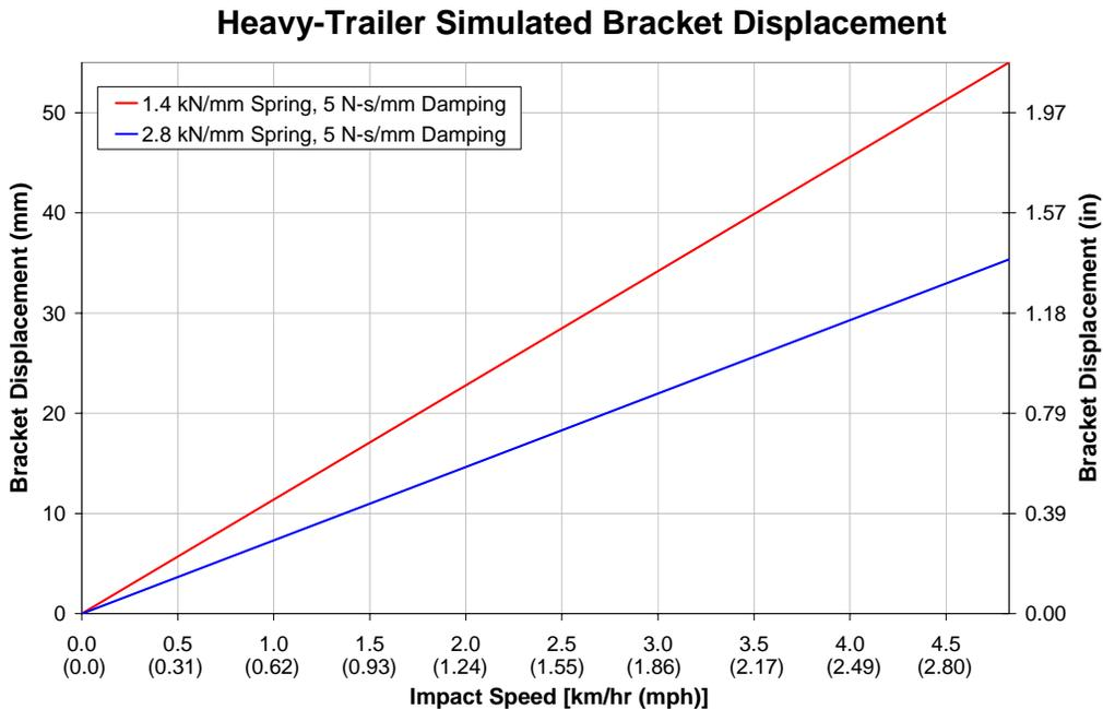
**Figure 4.9: Bracket displacement during heavyweight semitrailer coupling**
