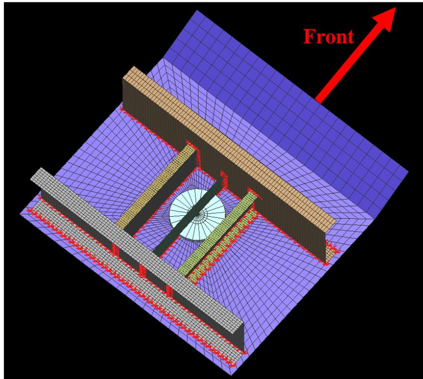
**Figure 5.5: Isometric top view of kingpin supporting structure with weld points**
