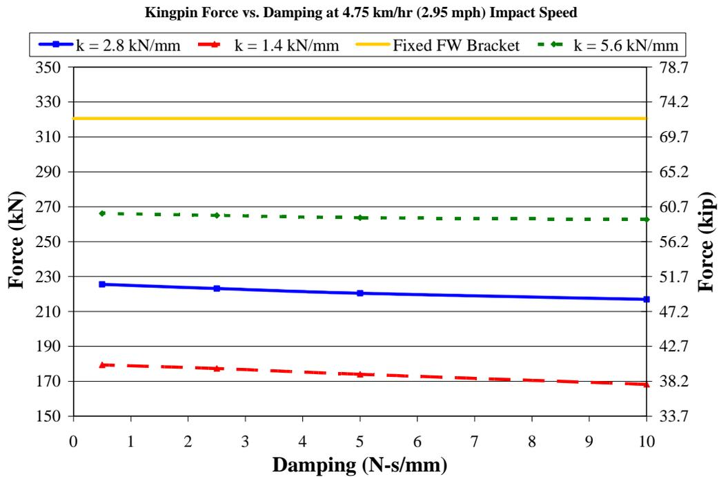
**Figure 3.7: Kingpin impact force of selected damping system parameters**
