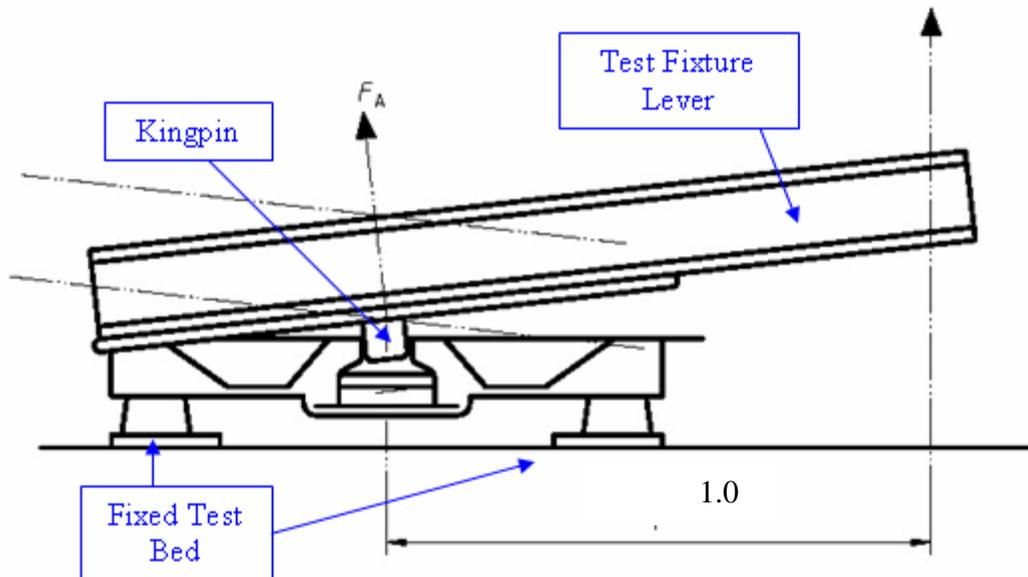
**Figure 1.7: Lifting test on fifthwheel couplings from ISO 8717 [3]**
