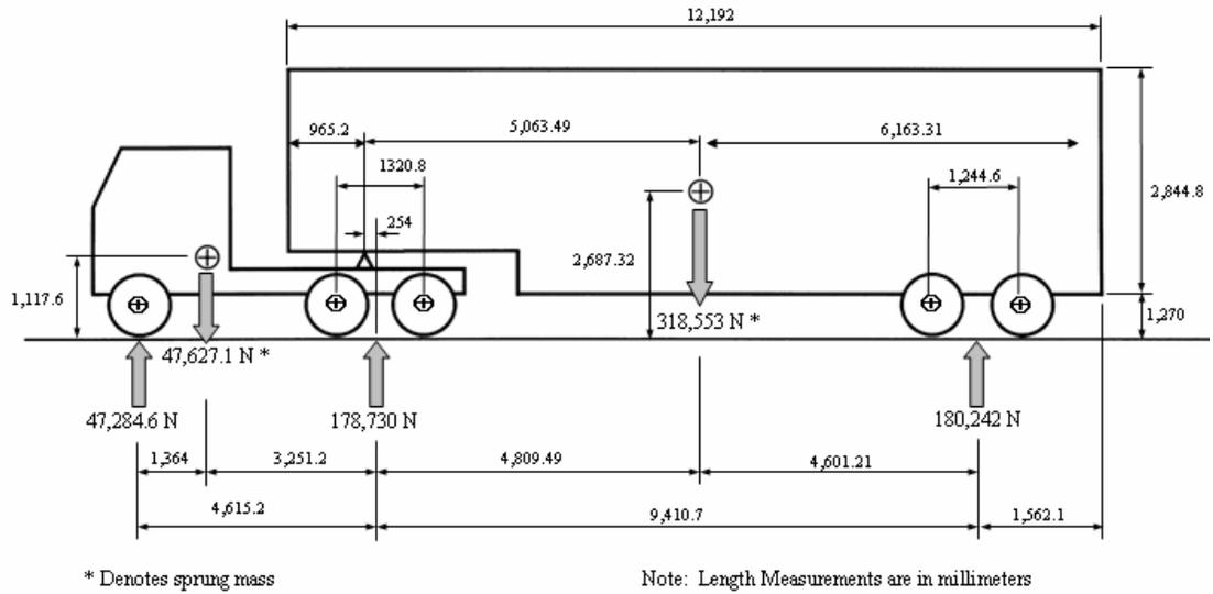
**Figure 1.1: Selected Tractor-Semitrailer (SI Units)**
