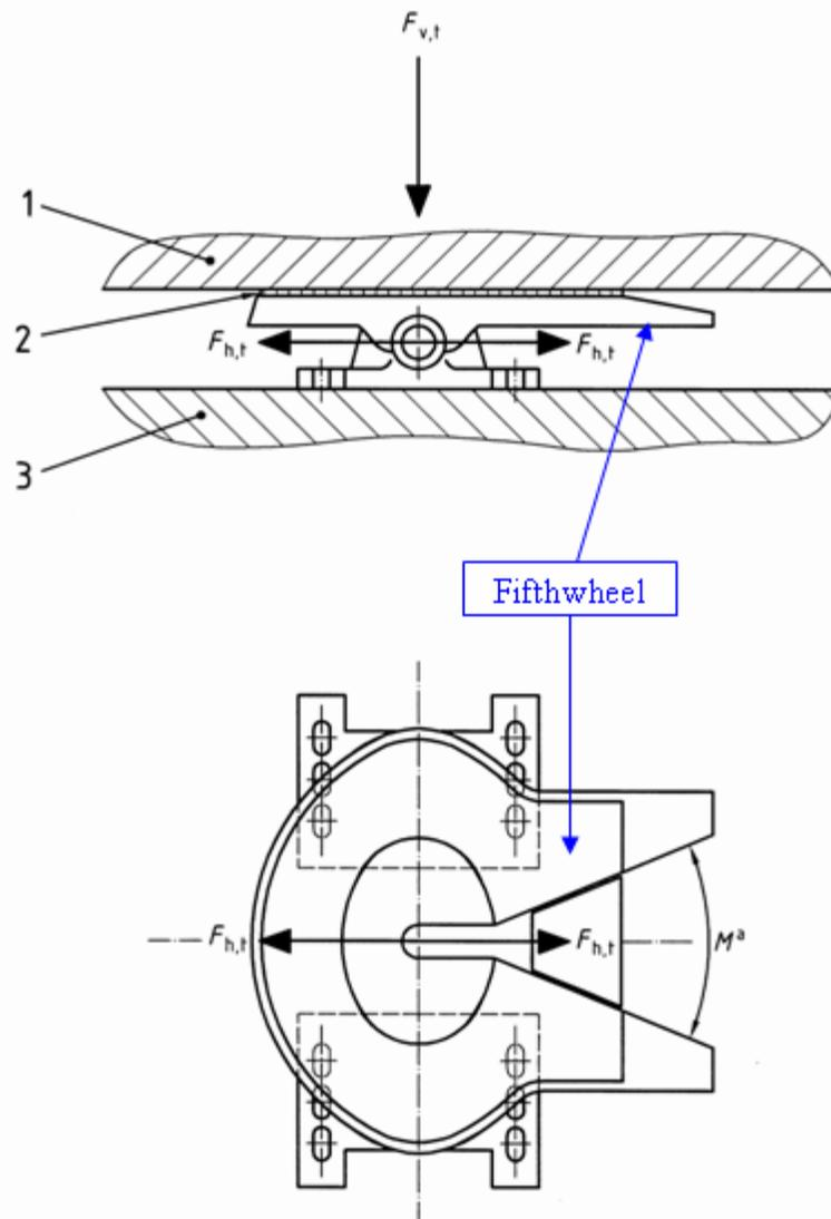
1: Counter-plate, 2: Polyamide foil, 3: Test bed
