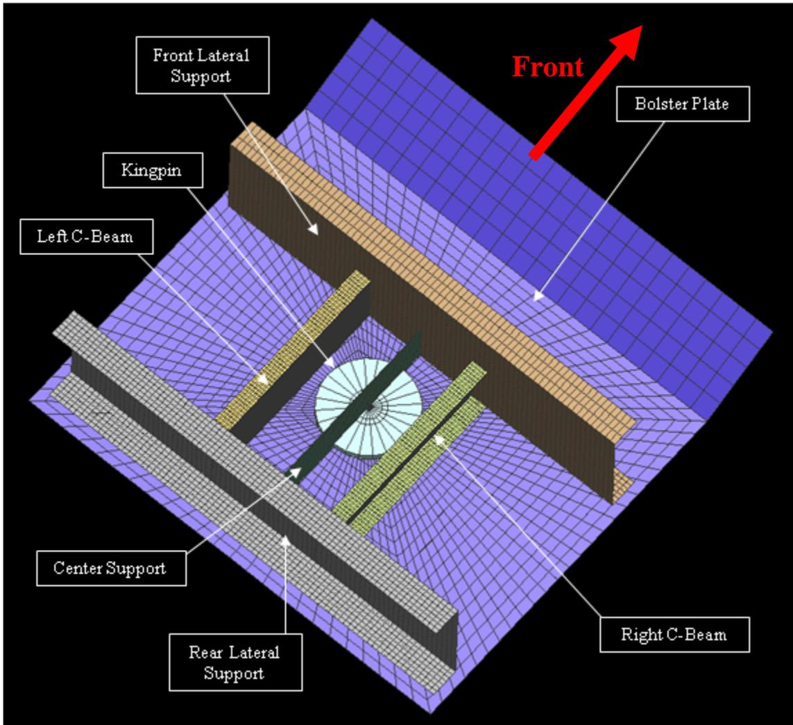
**Figure 5.4: Labeled isometric top view of the kingpin and support structure**
