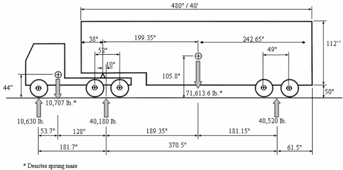
**Figure 1.2: Selected Tractor-Semitrailer (British Units)**
