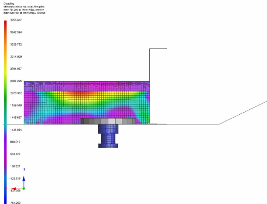
Figure 5.16: Side view of Von Mises stress plot from the upward load “E”
