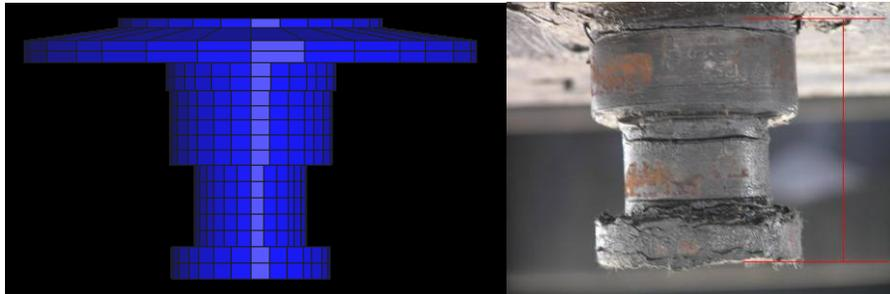
**Figure 2.1: Kingpin finite element model and photo**
