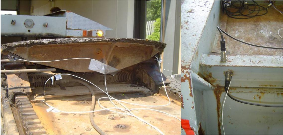
**Figure 3.1: Vertical and longitudinal accelerometers on the ARL tractor (left) and semitrailer (right)**
