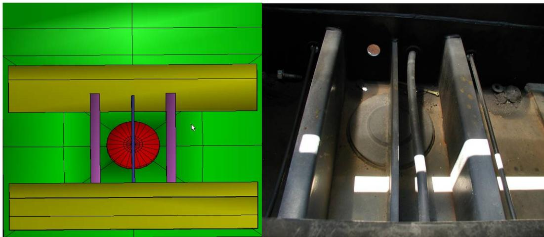
**Figure 2.10: FEA kingpin support structure model and actual support structure**
