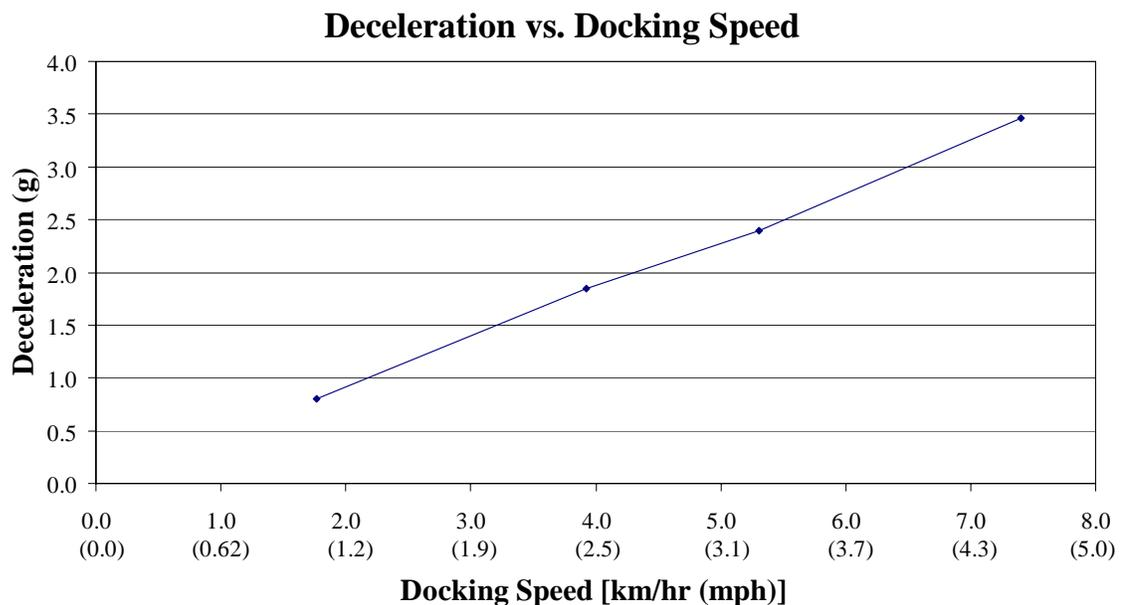
**Figure 1.15: Tractor Deceleration vs. Docking Speed [1]**
