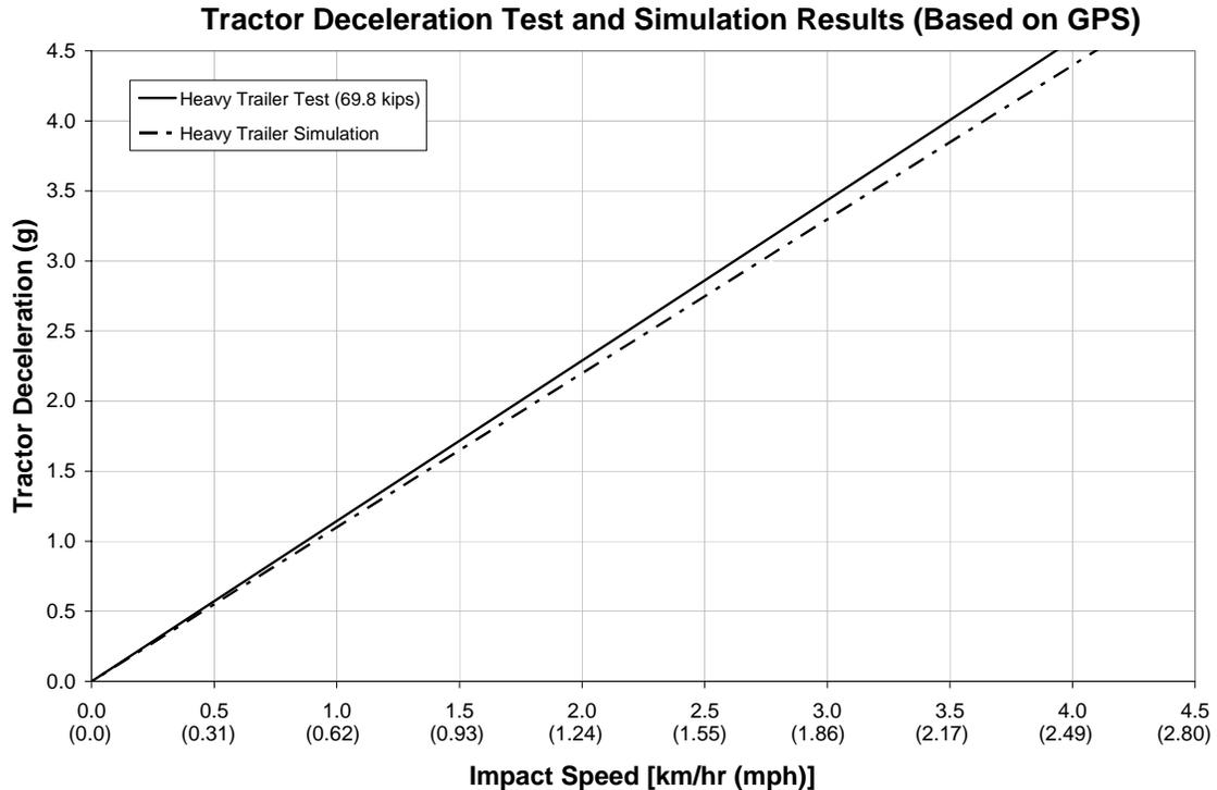
**Figure 4.5: Mack Trucks simulated and measured tractor deceleration vs. impact speed (GPS)**
