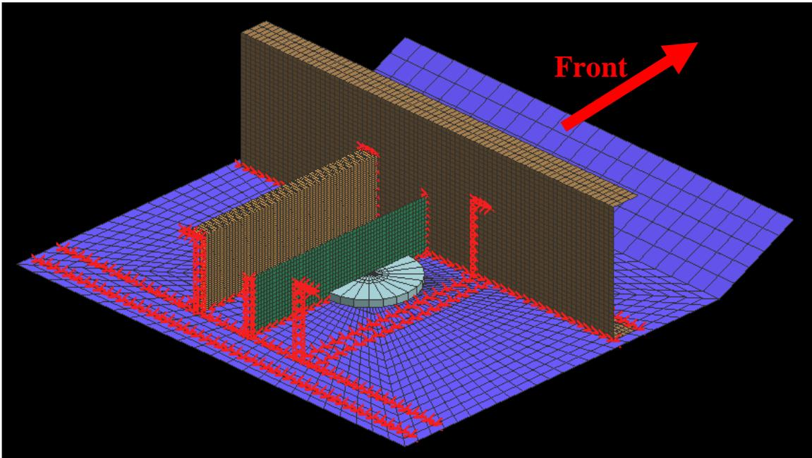
**Figure 5.6: Cut-away view of the kingpin support structure and weld points**
