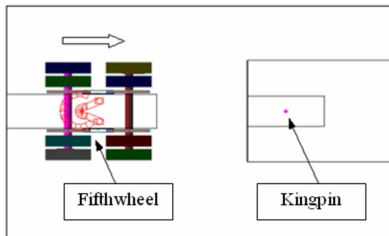
**Figure 1.11: Coupling Model**
