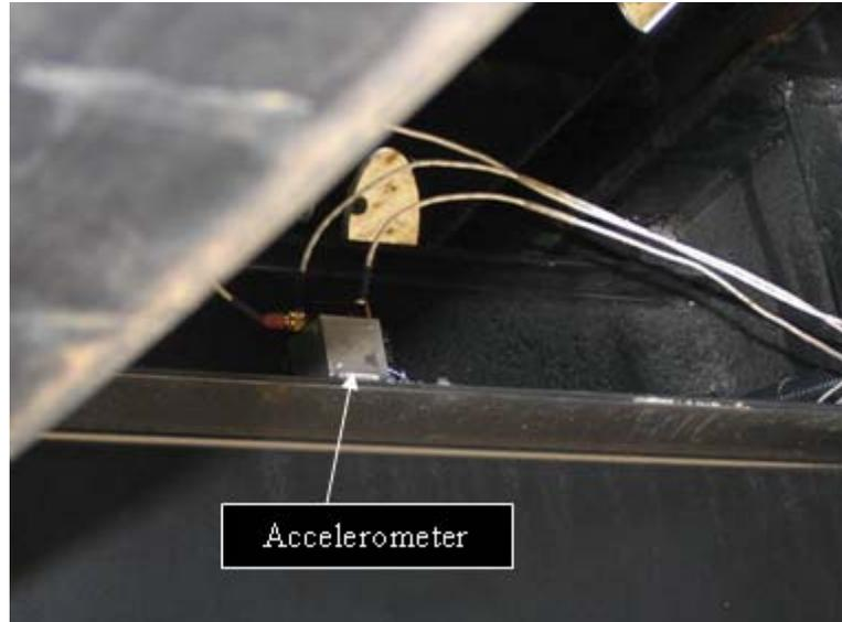
**Figure 4.2: Trailer accelerometer on Mack Trucks' instrumented Fontaine trailer**
