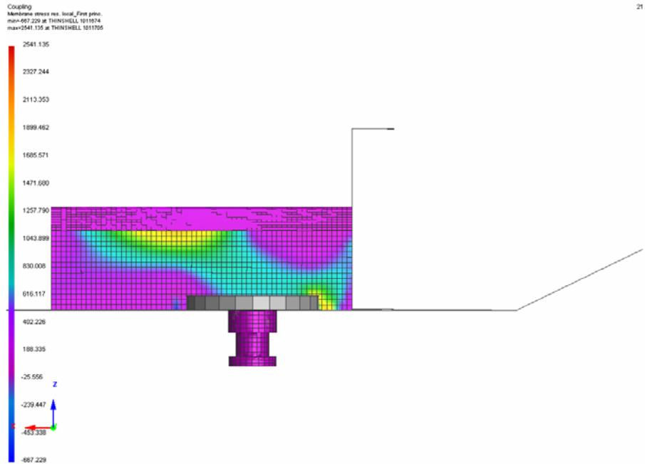
Figure 5.12: Side view of corrected SAE J133 load “A” Von Mises stress plot
