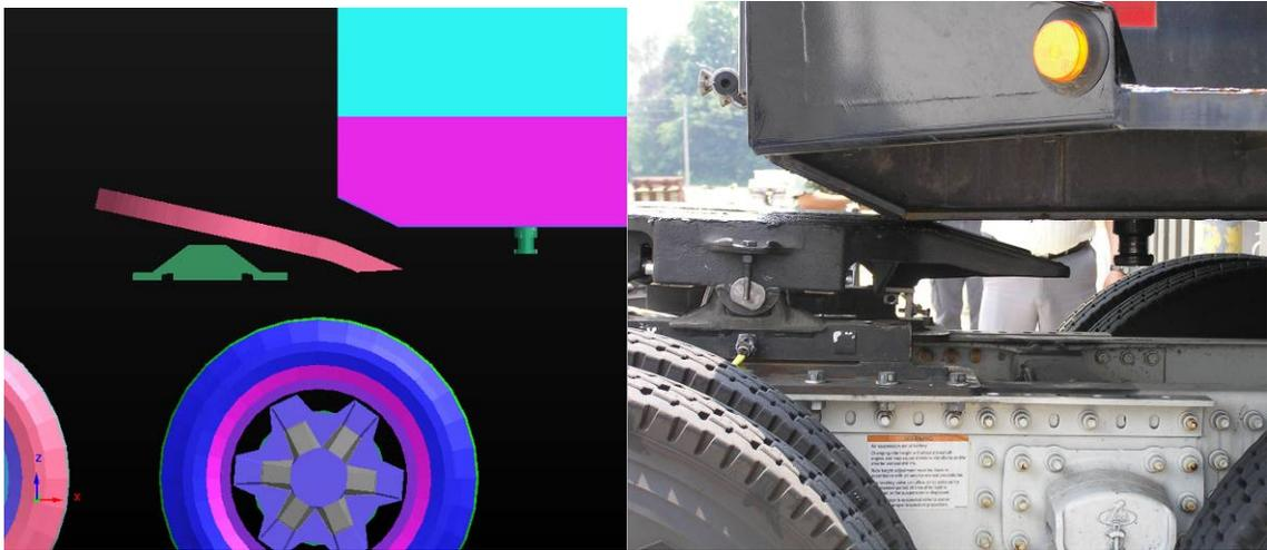
**Figure 2.12: Actual and simulated fifthwheel and kingpin near coupling position**
