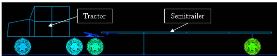
**Figure 2.4: ARL tractor-flatbed semitrailer FEA model**
