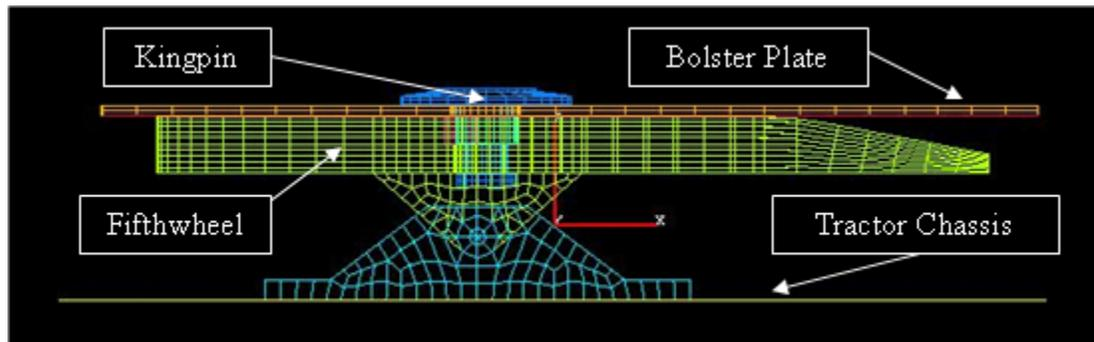
**Figure 2.3: FEA model of the coupled fifthwheel and kingpin**
