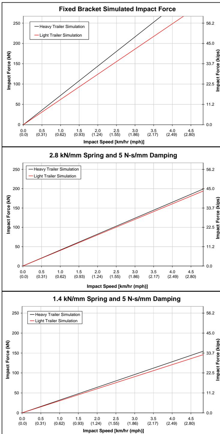
Figure 4.7: Coupling impact forces
