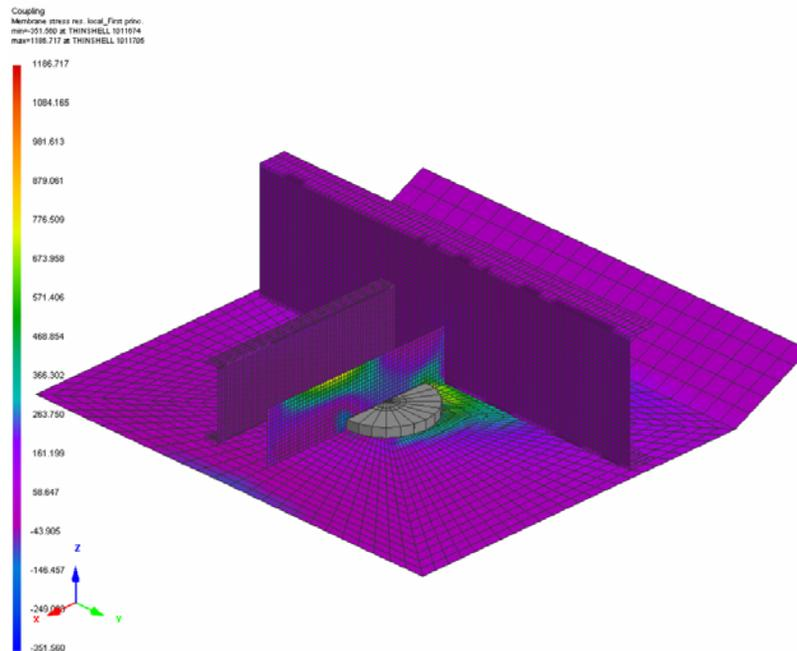
**Figure 5.9: Isometric view of current SAE J133 load “A” Von Mises stress plot**
