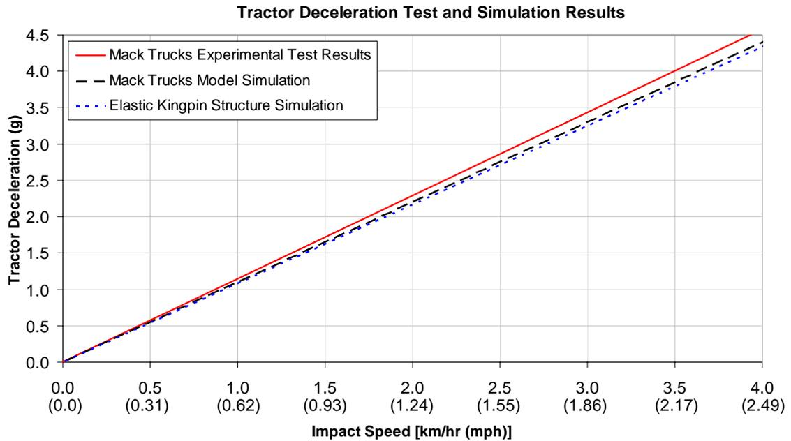
**Figure 5.8: Tractor deceleration vs. impact speed for validation of elastic model**
