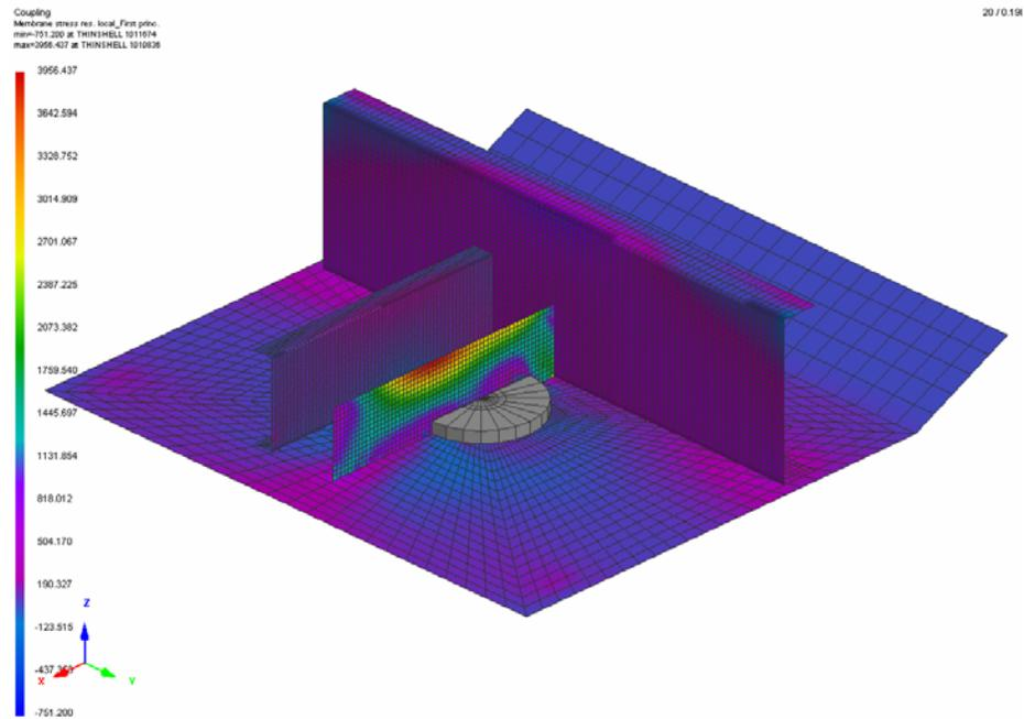
Figure 5.15: Isometric view of Von Mises stress plot from the upward load “E”
