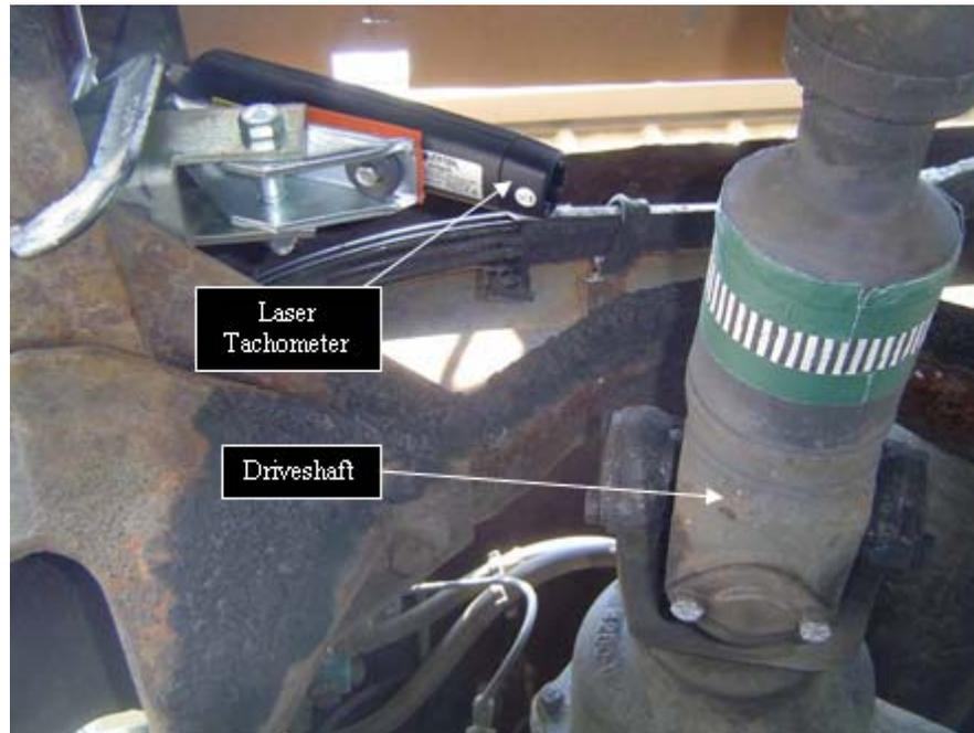
**Figure 3.2: ARL low speed tachometer driveline measurement system**
