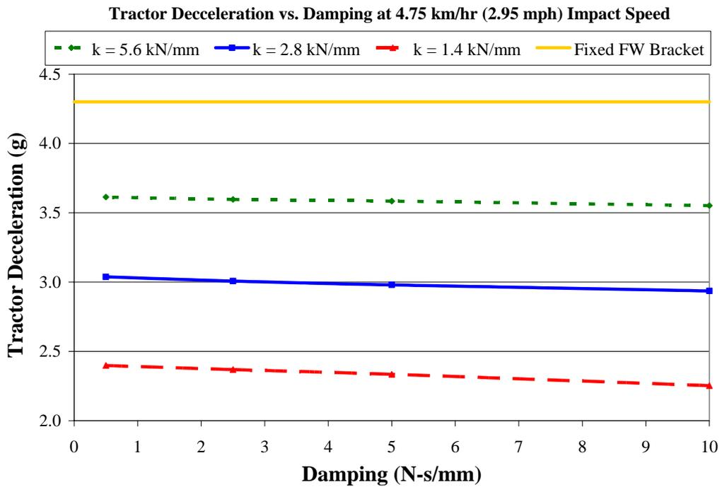
**Figure 3.6: Tractor deceleration of selected damping system parameters**
