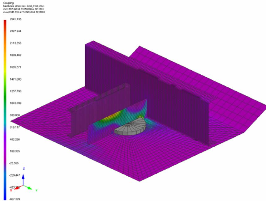
Figure 5.11: Isometric view of corrected SAE J133 load “A” Von Mises stress plot
