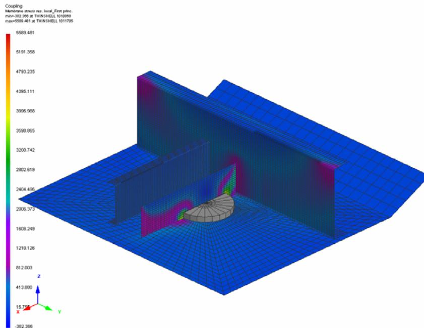
**Figure 5.13: Isometric view of Von Mises stress plot from the downward load “E”**
