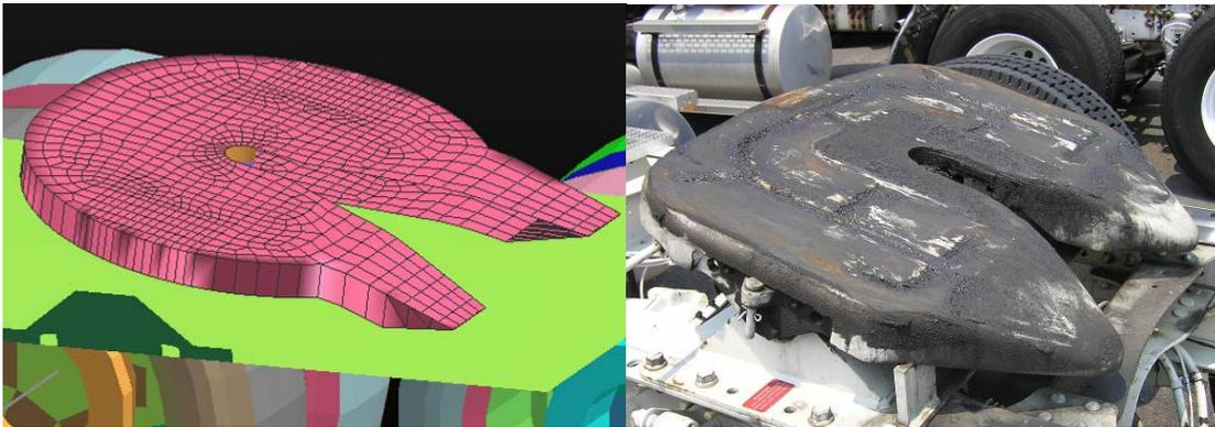
**Figure 2.2: Fifthwheel finite element model and photo**
