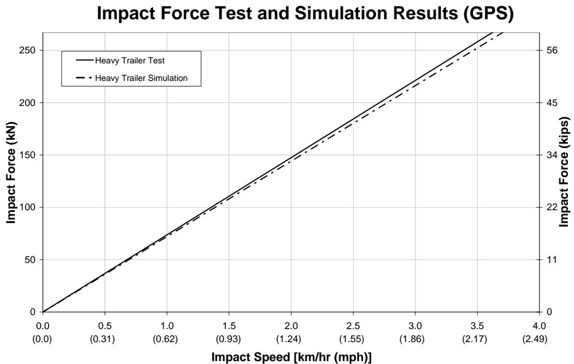
**Figure 4.6: Mack Trucks measured and simulated impact force vs. impact speed**
