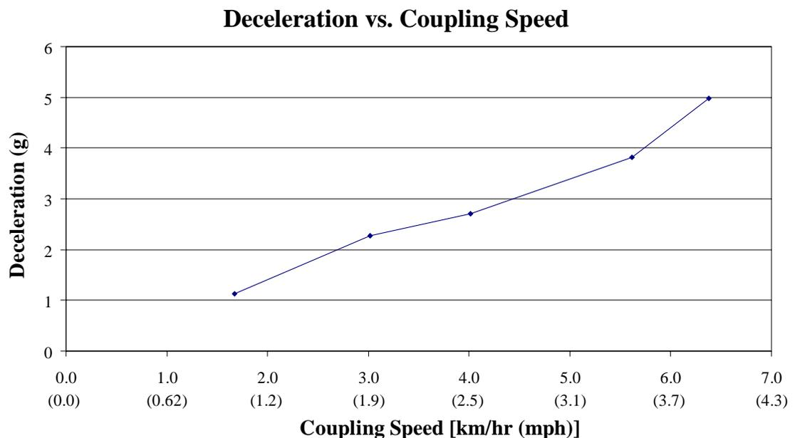
**Figure 1.12: Tractor Deceleration vs. Coupling Impact Speed [1]**
