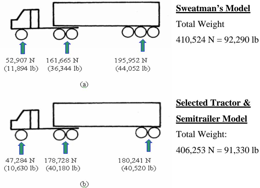
**Figure 1.9: (a) 6-axle tractor-semitrailer [6] and (b) tractor-semitrailer selected for this report**
