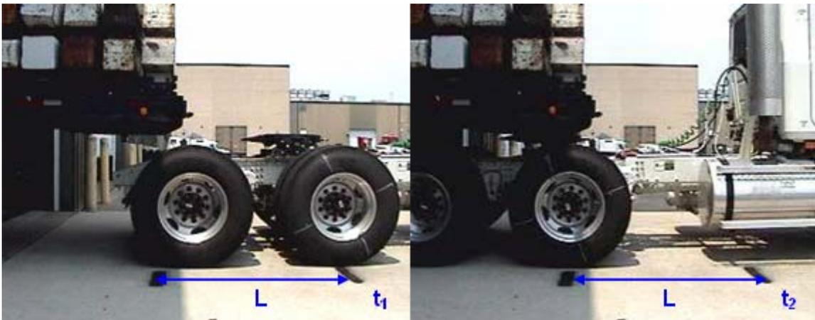
**Figure 4.3: Digital video frames used for impact speed estimation**
