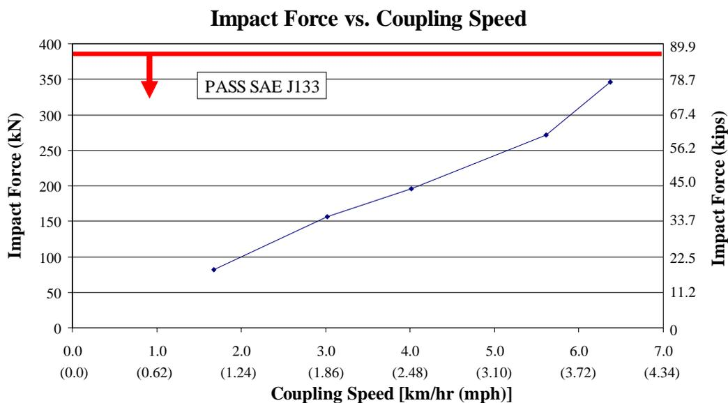
**Figure 1.13: Kingpin Force vs. Coupling Impact Speed [1]**
