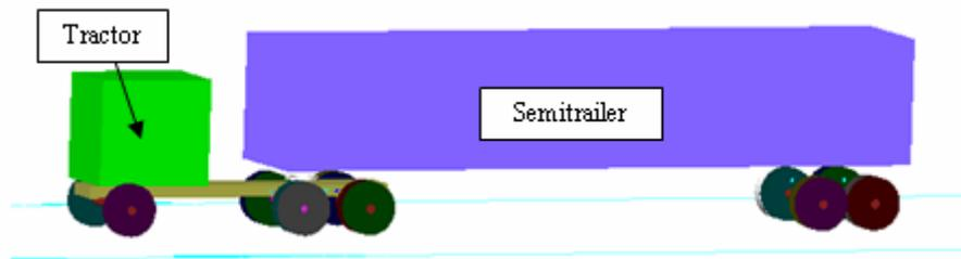
**Figure 1.10: Five-axle tractor-semitrailer DADS<sup>®</sup> model [1]**
