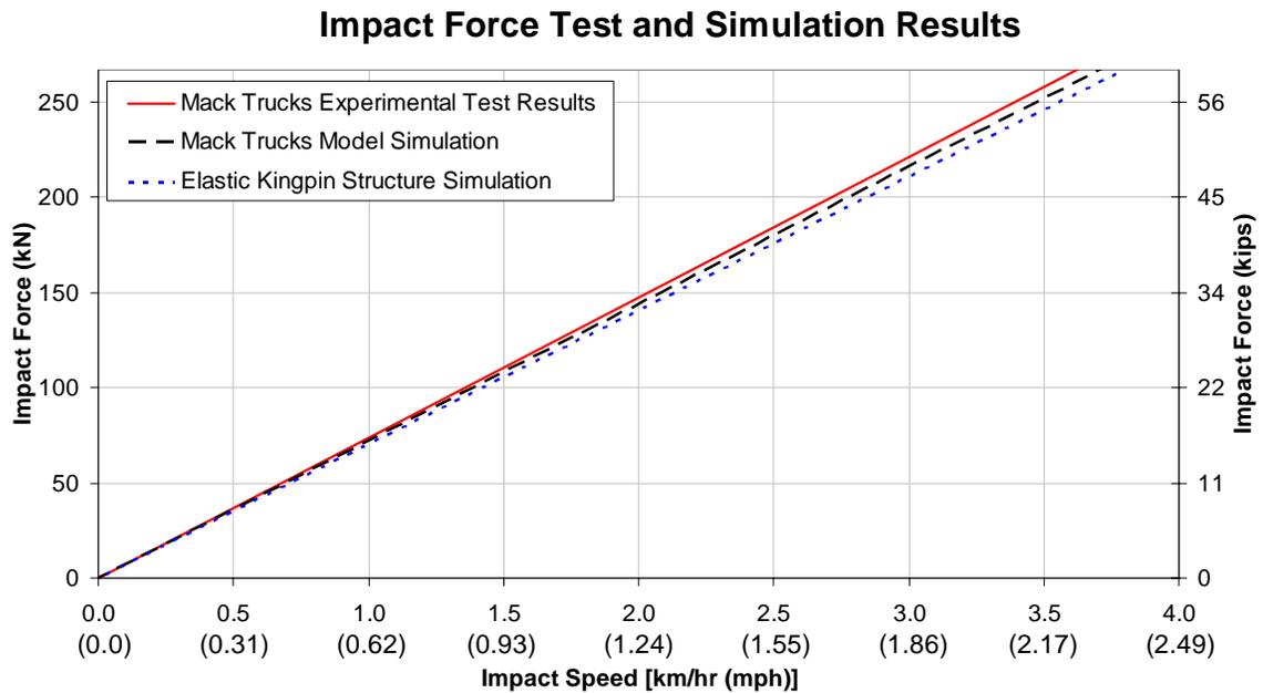
**Figure 5.7: Kingpin impact force vs. impact speed for validation of elastic model**
