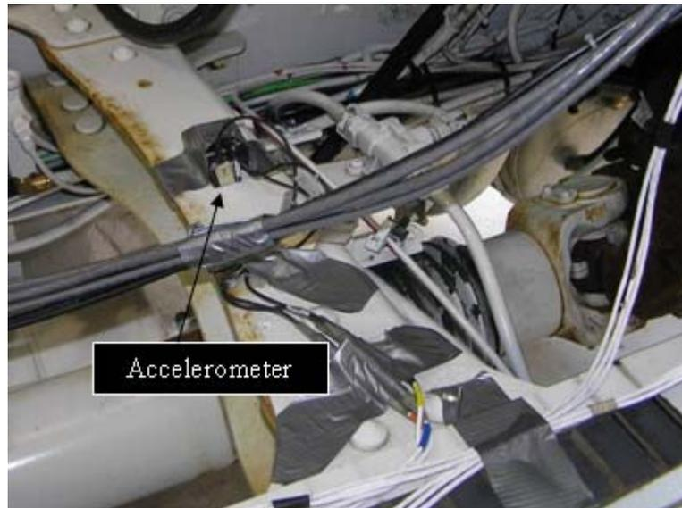
**Figure 4.1: Tractor accelerometer on Mack Trucks' instrumented tractor chassis**
