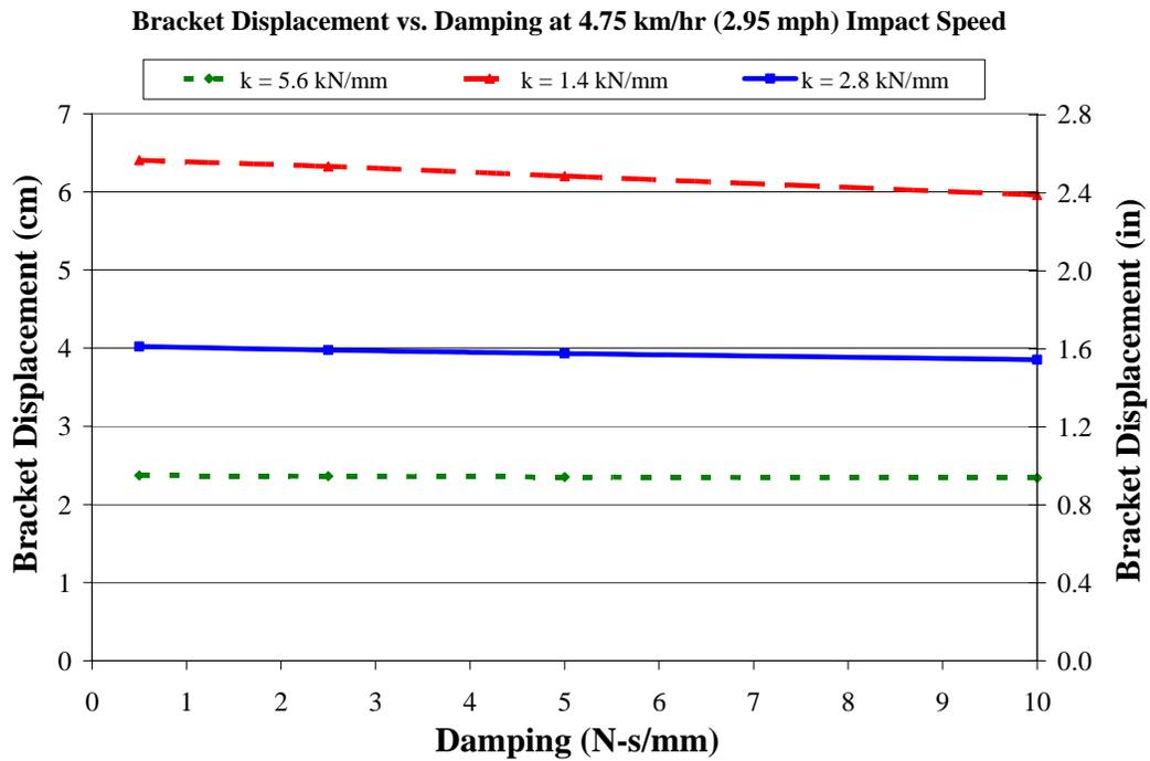
**Figure 3.5: Bracket displacement of selected damping system parameters**
