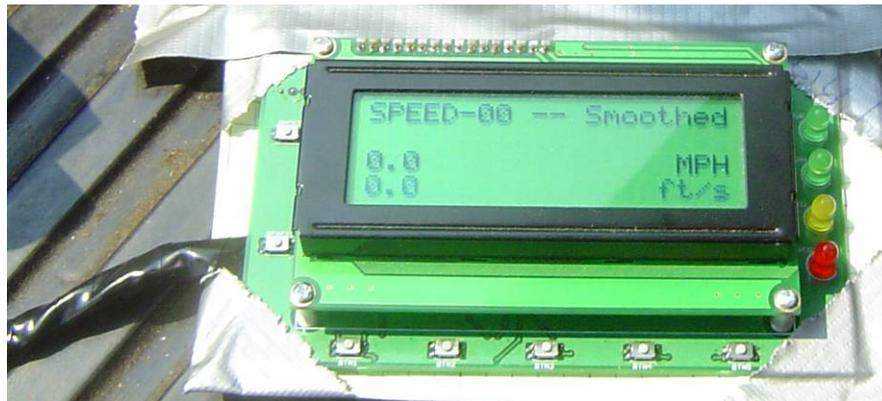
**Figure 3.3: Digital display inside the tractor cab for low speed measurements**
