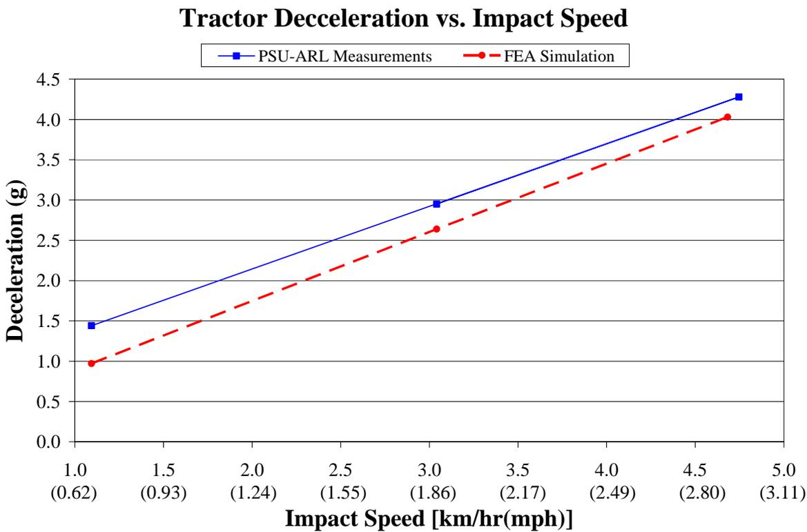
**Figure 3.4: Validation comparison between ARL experimental measurements and FEA simulations**
