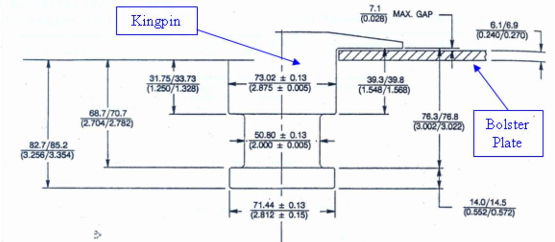
**Figure 1.5: Detailed drawing of an upper coupler kingpin from SAE J700 [4]**
