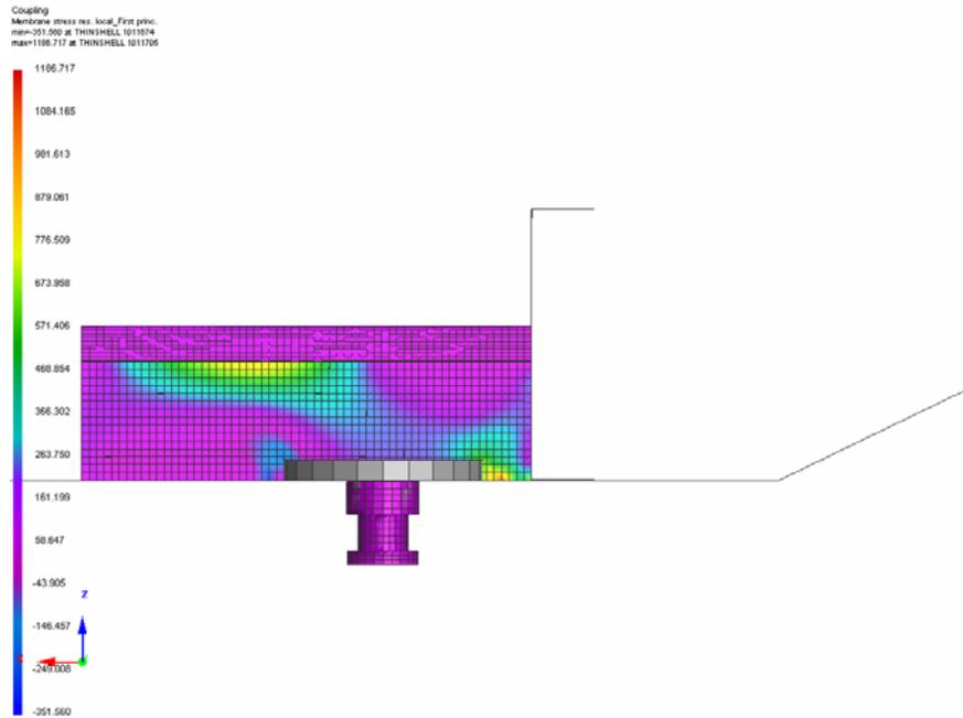
**Figure 5.10: Side view of current SAE J133 Load “A” Von Mises stress plot**
