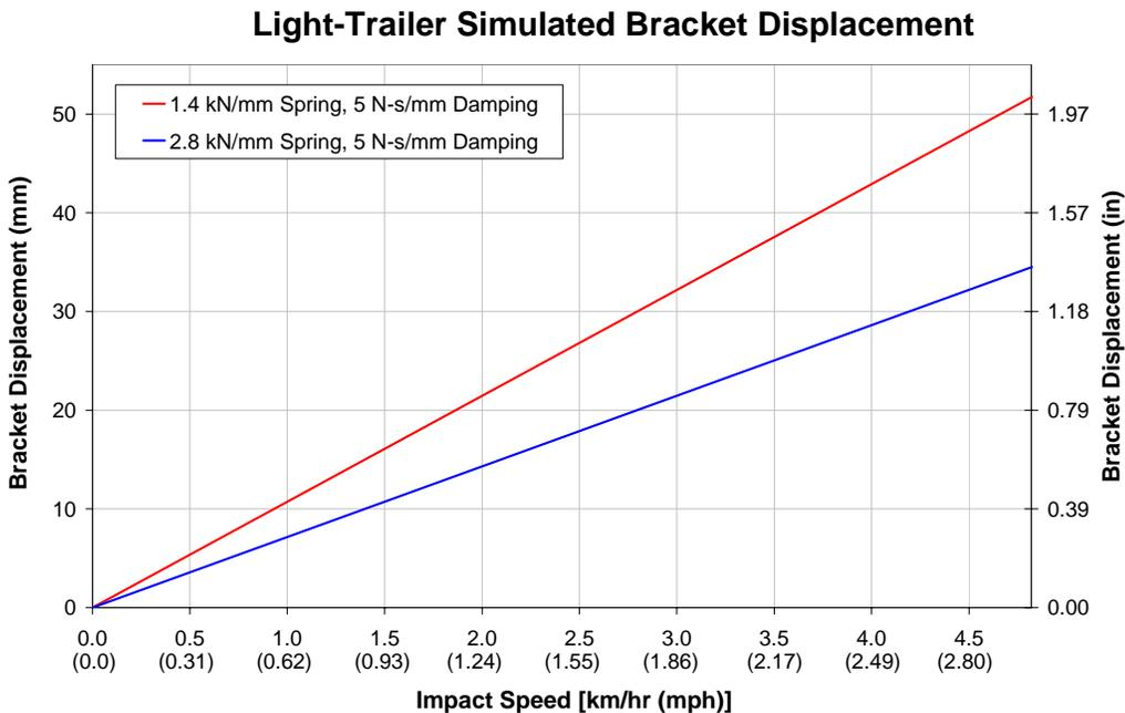
**Figure 4.10: Bracket displacement during lightweight semitrailer coupling**
