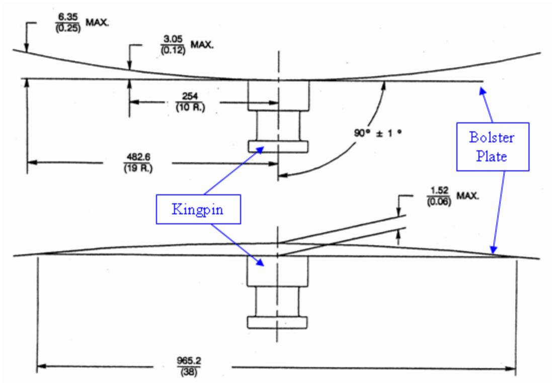
**Figure 1.6: Allowable bowing of kingpin supporting structure plate from [4]**
