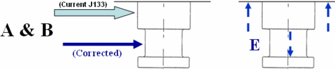
**Figure 1.4: Correct points of application for loads “A”, “B”, and “E” in SAE J133**
