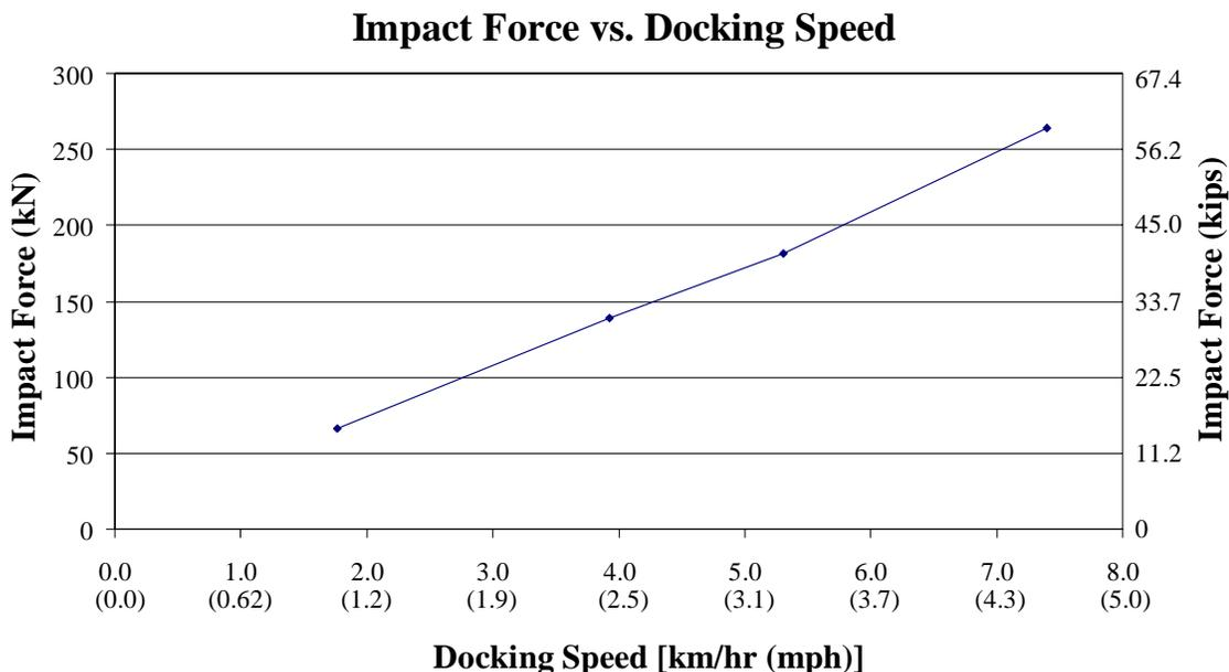
**Figure 1.16: Longitudinal Kingpin Force vs. Docking Speed [1]**
