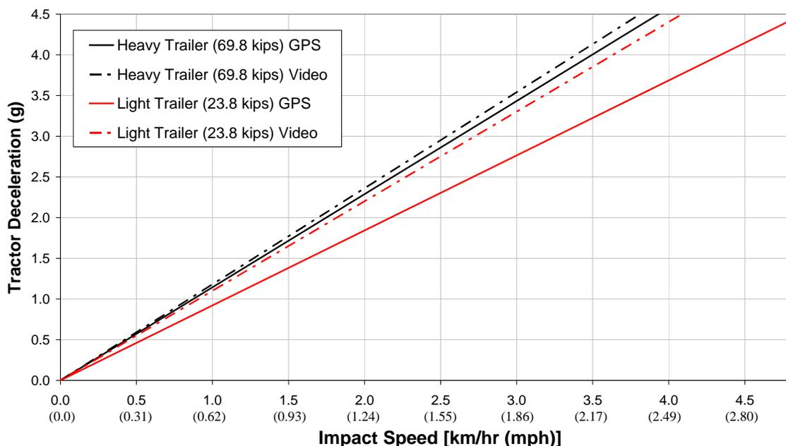
**Figure 4.4: Tractor deceleration vs. impact speed (GPS and digital video) during Mack Trucks' coupling tests**
