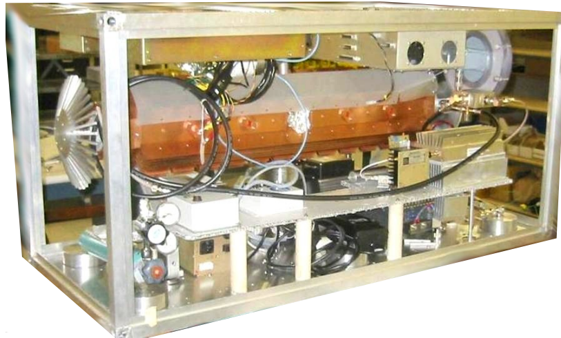
Figure 4.8. The internals of the portable neutron generator used to irradiate the single-phase Ar detector. The generator was designed and built by AccSys, Inc., [134]. Protons are produced by an electron cyclotron resonance (ECR) source and accelerated by a compact radiofrequency quadrupole (RFQ).
