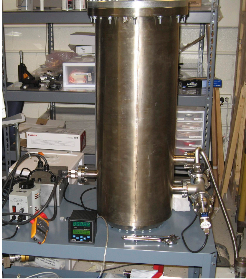
Figure 5.11. The vacuum evaporation system is used for coating both reflectors and windows with TPB to wavelength shift the Ar scintillation light. The chamber is pumped down to a base pressure of \sim 10^{-3} Torr before the crucible is heated to the melting temperature of the TPB.
