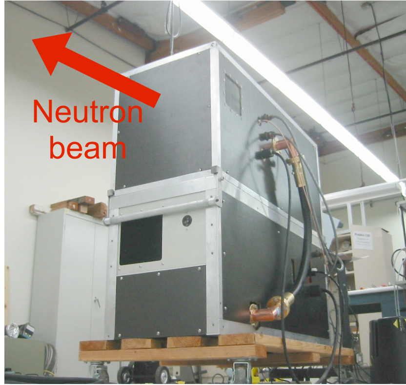
Figure 4.7. The portable neutron generator used to irradiate the single-phase Ar detector for measurement of the nuclear ionization quench factor. The internals of the generator are shown in Figure 4.8.
