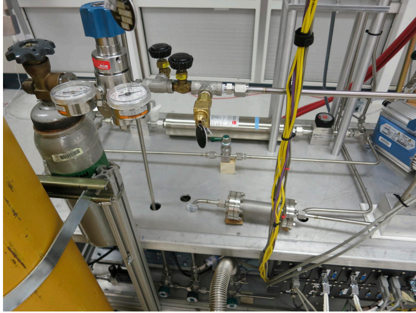
Figure 6.5. ^{37}\text{Ar} was first injected into a calibration volume of \sim 250\text{ cm}^3 , and then pumped through a SAES getter into the detector using the circulation system. As the ^{37}\text{Ar} decayed, the number of calibration volumes injected increased to maintain a nearly constant activity of ^{37}\text{Ar} inside the detector.
