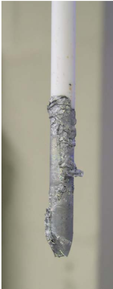
Figure 23. Aluminum coating on alumina loading rod after testing.
