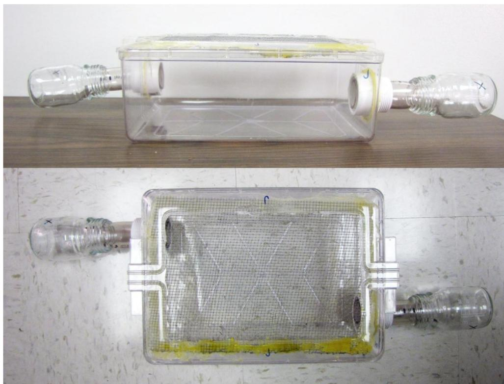
**Figure 2-2. Choice test apparatus.** (above) Side view. (below) Top view of screened lid.
