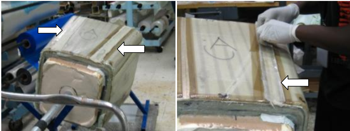
Figure 4-1. GRP strip bridging over caul blocks
