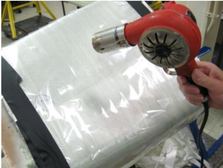
Figure 3-48. Shrink Tape on spar with heat gun.
