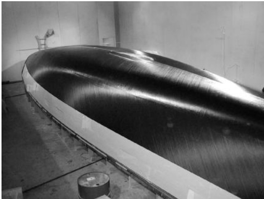
Figure 2-7. Male mold of yacht hull with prepreg applied (Downs-Honey et al, 2003)
