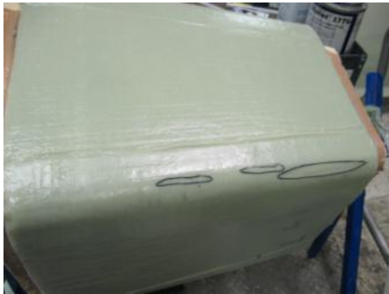
Figure 3-36. Very slight dimpling on spar corner post-cure
