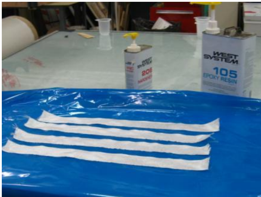
Figure 3-40. 2” Wide GRP strips for caul gap filling
