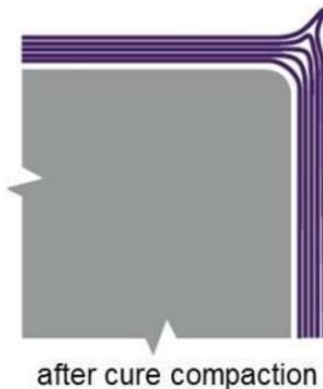
Figure 1-3. Post-vacuum bag compaction of prepreg material (Gurit, 2012)
