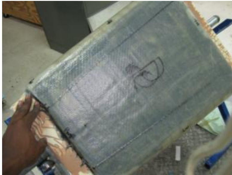
Figure 3-30. Flat and corner caul blocks post-cure (NOT DEMOLDED)
