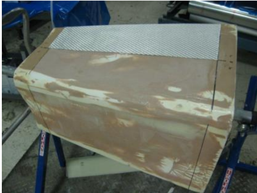
Figure 3-15. First ply lay-up on mandrel
