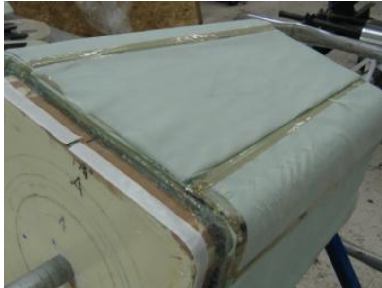
Figure 3-32. Caul block application pre-vacuum
