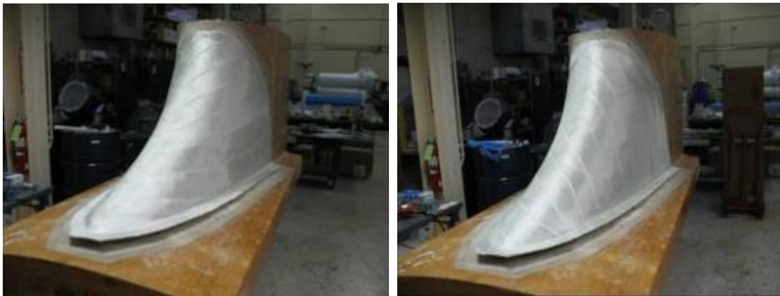
Figure 2-11. Cusp fairing lay-up change in direction of ply lay-up (Juska et al, 2012)
