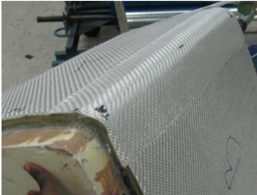
Figure 3-29. Corner caul & Flat caul block lay-up cont.
