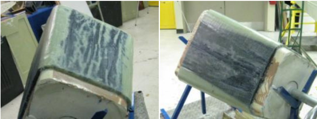
Figure 3-20. Application of blue fairing compound to spar
