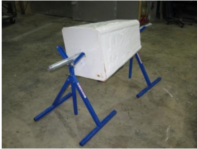
Figure 3-12. Foam core mandrel
