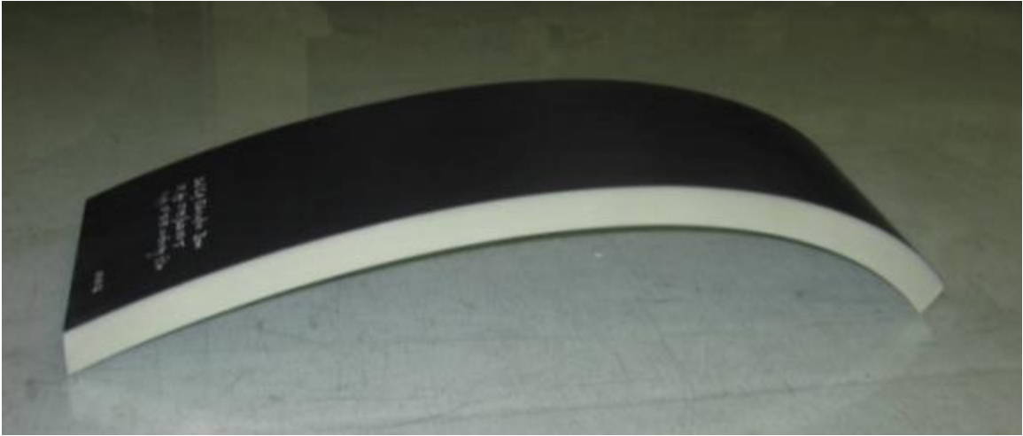
Figure 2-15. Second trial male molded w/ surfacing film (Juska et al, 2012)
