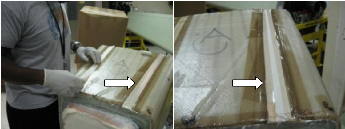
Figure 4-2. Syntho-Glass strip cut into smaller sections - No bridging
