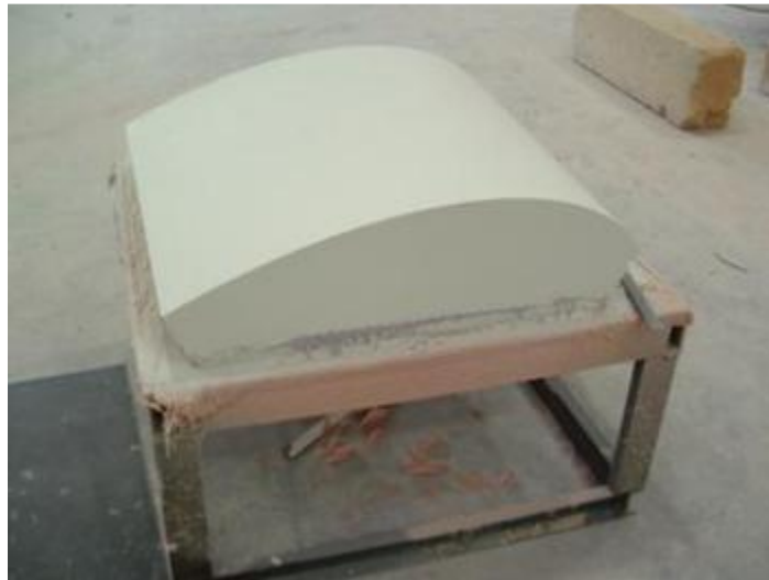
Figure 2-12. Male mold for doubly curved structure (Juska et al, 2012)
