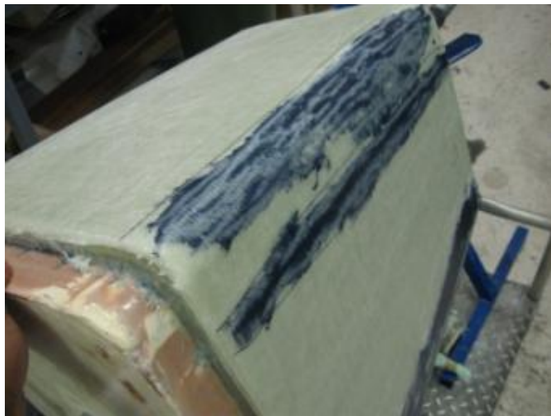
Figure 3-35. Fairing compound applied to corner section of spar
