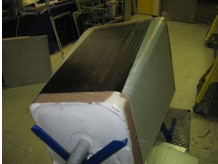
Figure 3-2. Second ply lay-up on mandrel
