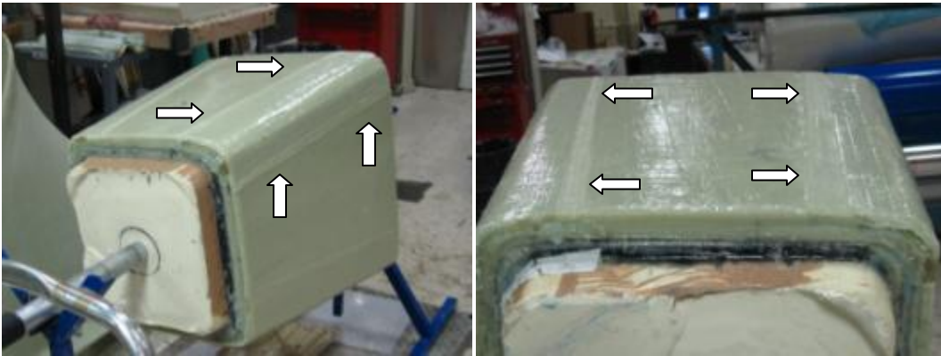
Figure 3-41. Post-Cure of GRP strip stage
