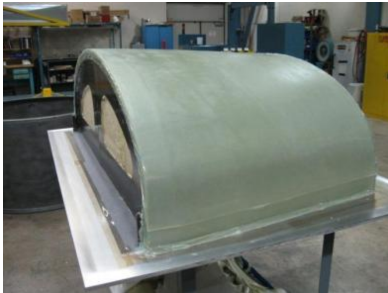
Figure 2-18. Mark off on third trial of doubly curved surface post-cure (Juska et al, 2012)
