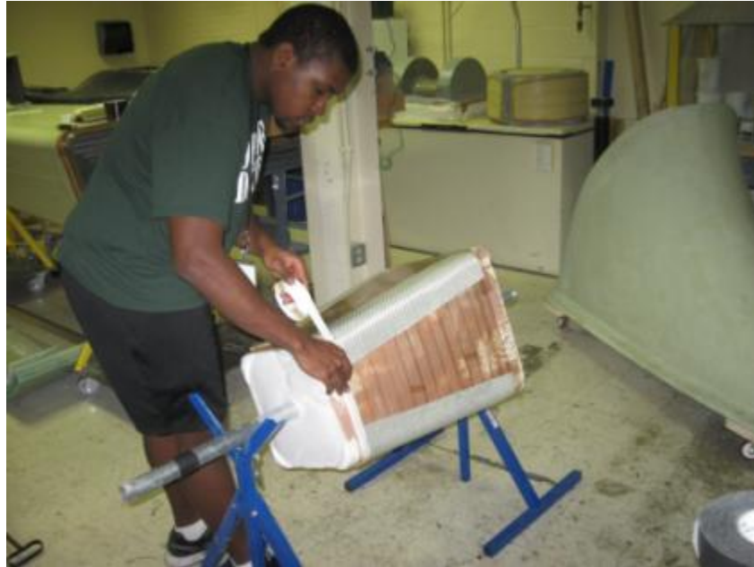
Figure 3-14. Corner caul lay-up cont.
