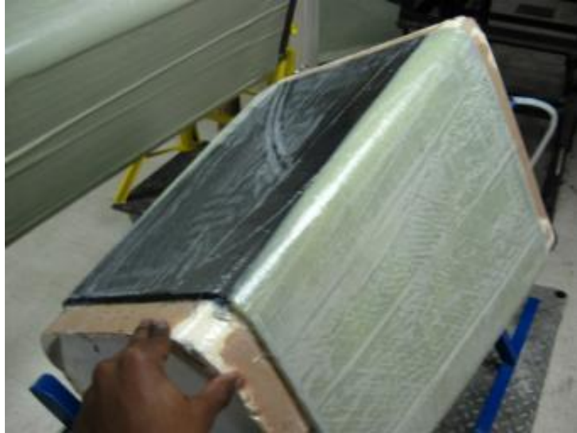
Figure 3-19. Spar post-cure sanding
