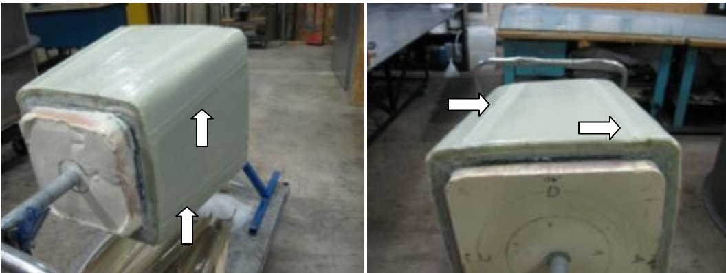
Figure 3-46. Syntho-Glass second trial used as gap filler in conjunction with caul blocks
