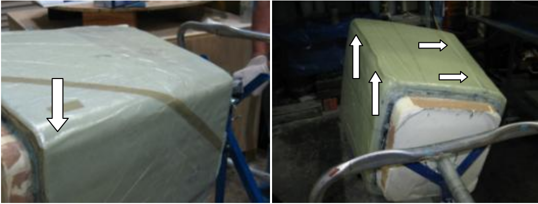
Figure 3-44. Post-Cure first Syntho-Glass trial
