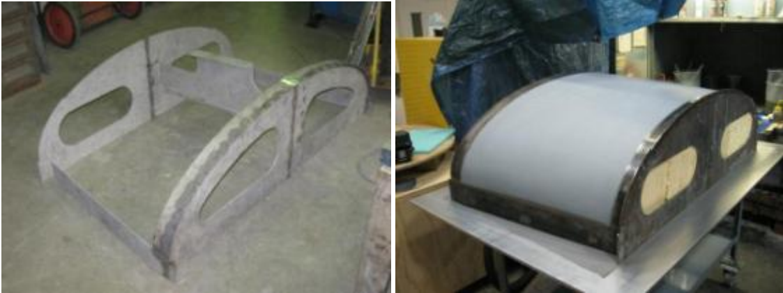
Figure 2-16. Male mold with steel frame for third trial of doubly curved surface (Juska et al, 2012)
