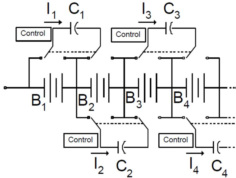
Figure 1.5 Charge Shuttling with Several Cells [4]
