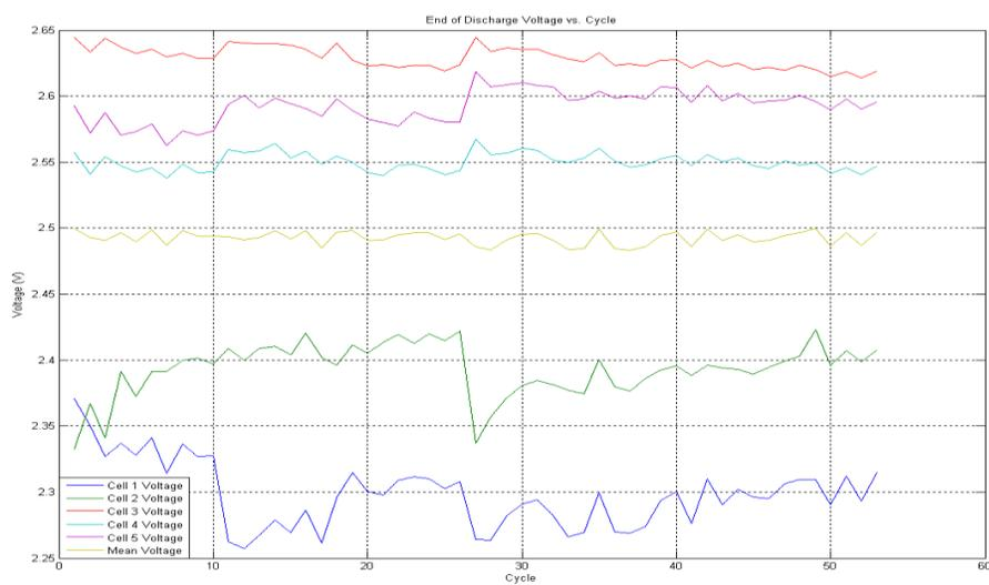
Figure A.2 Cell Voltages at the End of Discharge vs. Cycle (Five Cell Test 1)
