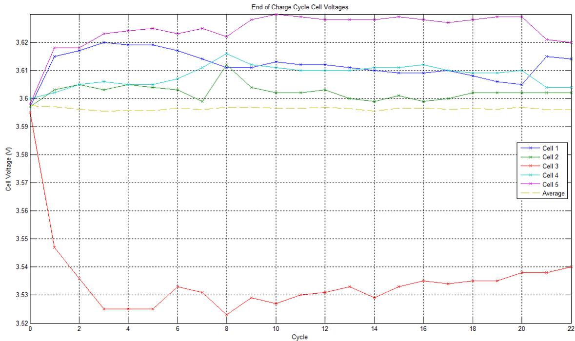
**Figure 5.6 Cell Voltages at the End of the Charge Cycle (Five Cell Test 2)**
