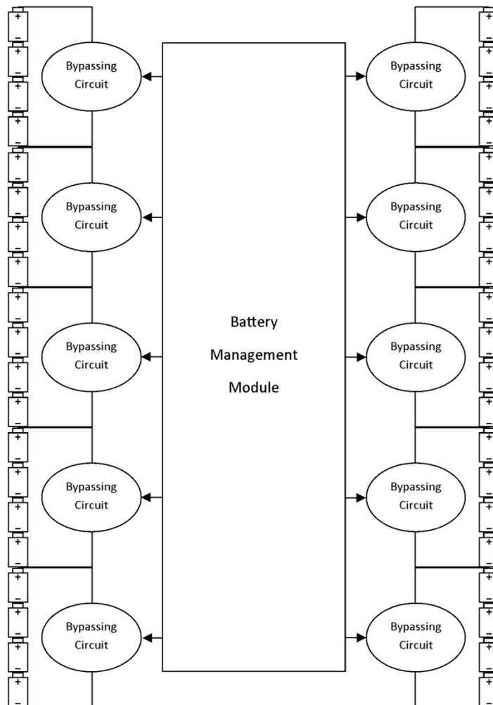
Figure 6.1 Battery Management Module
