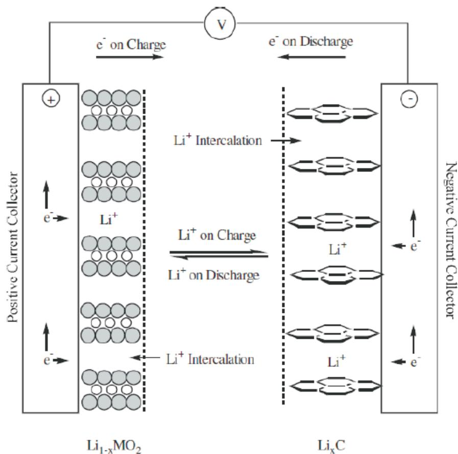
Figure 1.1 Schematic Diagram of a Lithium Ion Cell [6]
