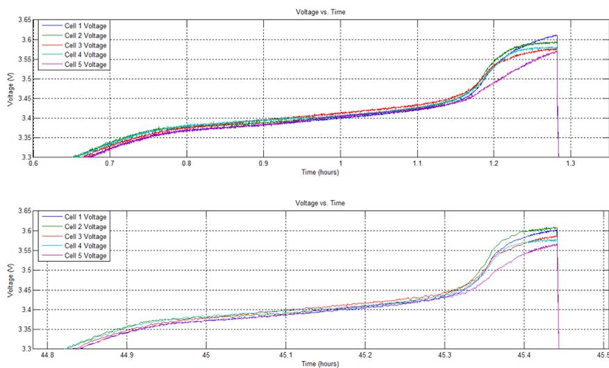
Figure A.1 Cell Voltages at the End of Charge 1 and 53 for the Five Cell Test 1
