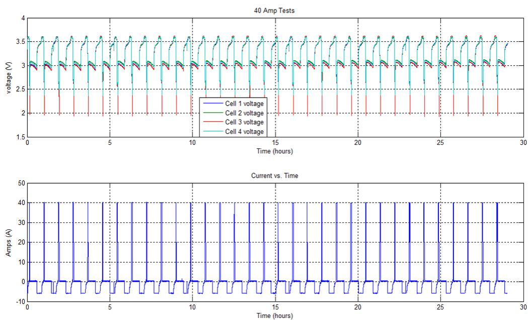
Figure A.3 Cell Voltages at the End of Discharge vs. Cycle (Four Cell Test 40A)
