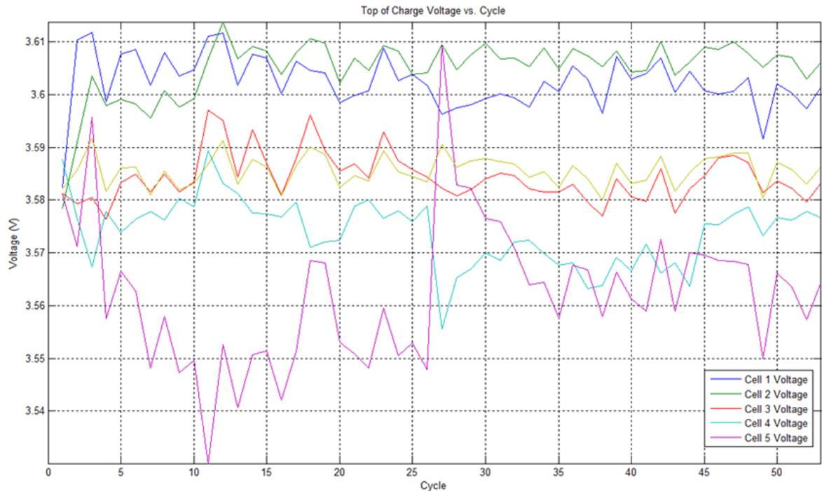
Figure 5.3 Cell Voltage at the End of Each Charge (Five Cell Test 1)
