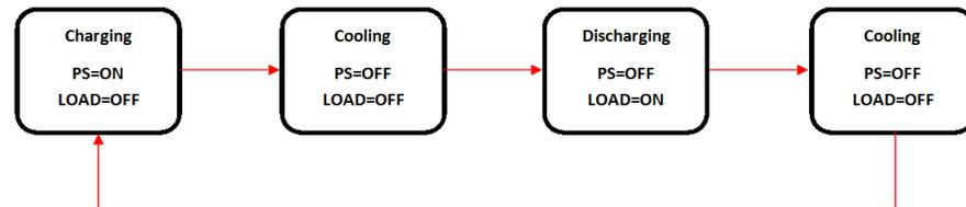
**Figure 3.3 Battery Cycling Program State Diagram**
