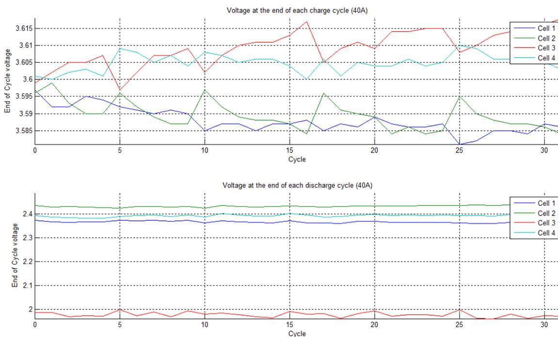
Figure 5.8 Cell Voltages at End of the Charge Cycle (Four Cell Test 40A)
