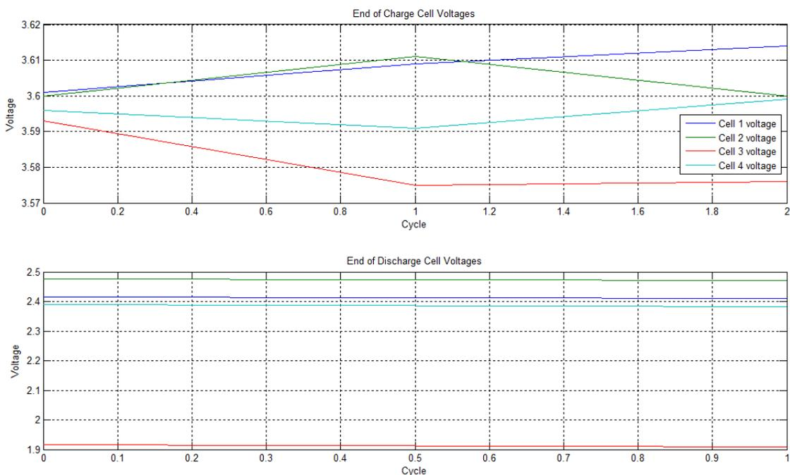
**Figure 5.7 Cell Voltages at the End of the Charge Cycle (Four Cell Test 30A)**
