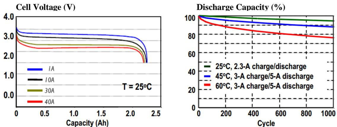
Figure 1.2 Lithium Iron Phosphate Cell Characteristics
