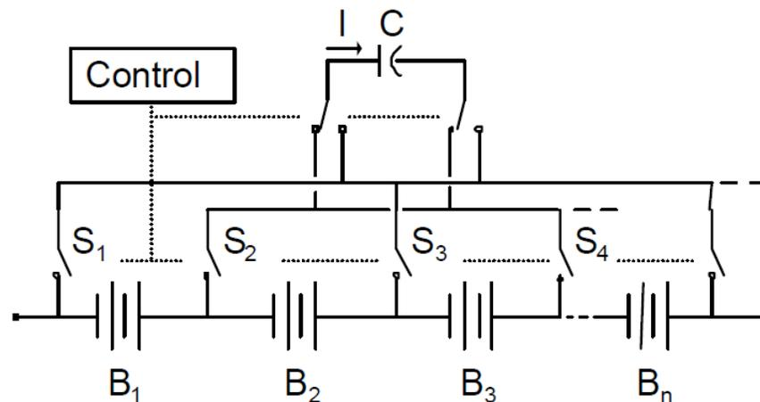
Figure 1.4 Flying Capacitor Charge Shuttling Method [4]
