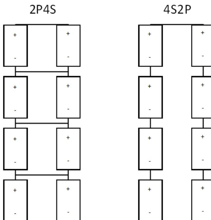
Figure 1.3 Series and Parallel Cells
