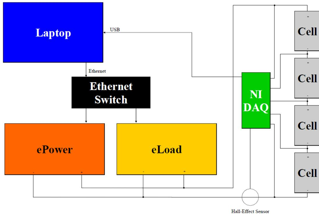
**Figure 3.1 Battery Cycling System Setup**
