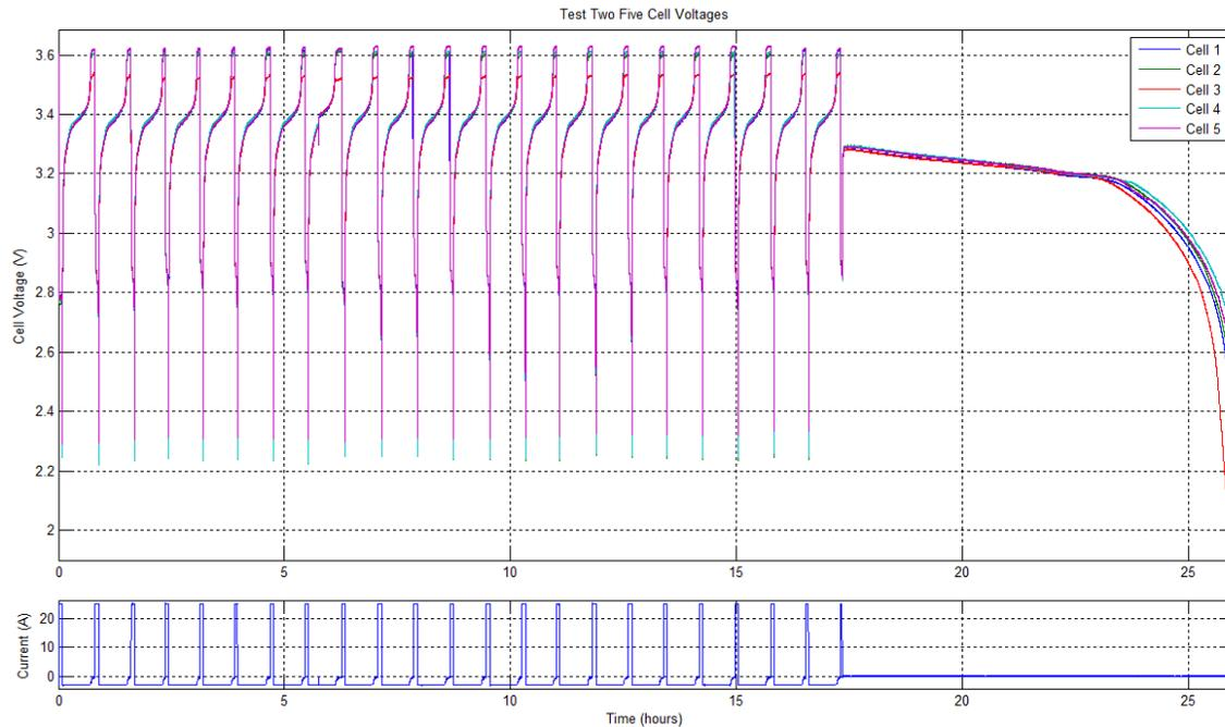
Figure 5.5 Cell Voltages and Current vs. Time (Five Cell Test 2)
