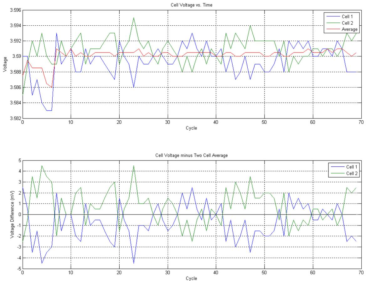
Figure 5.1 Two Cell Cycling Voltages at Top and Bottom of the Charge Cycle
