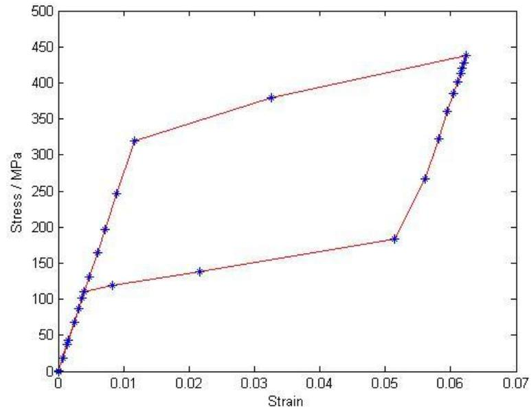
Figure 2-7 Stress-strain hysteresis plot for tension simulation.
