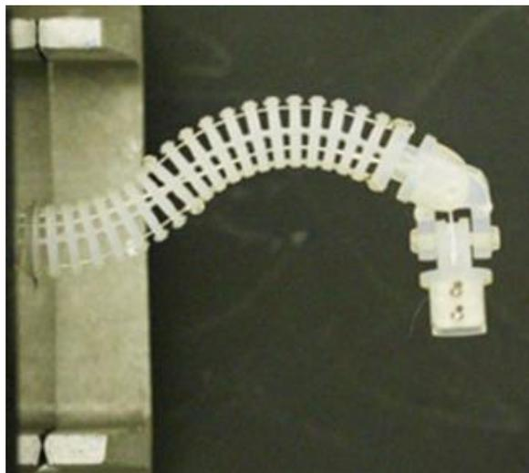
**Figure 1-24 Multi-sector flexible snake driven by four cables [61].**
