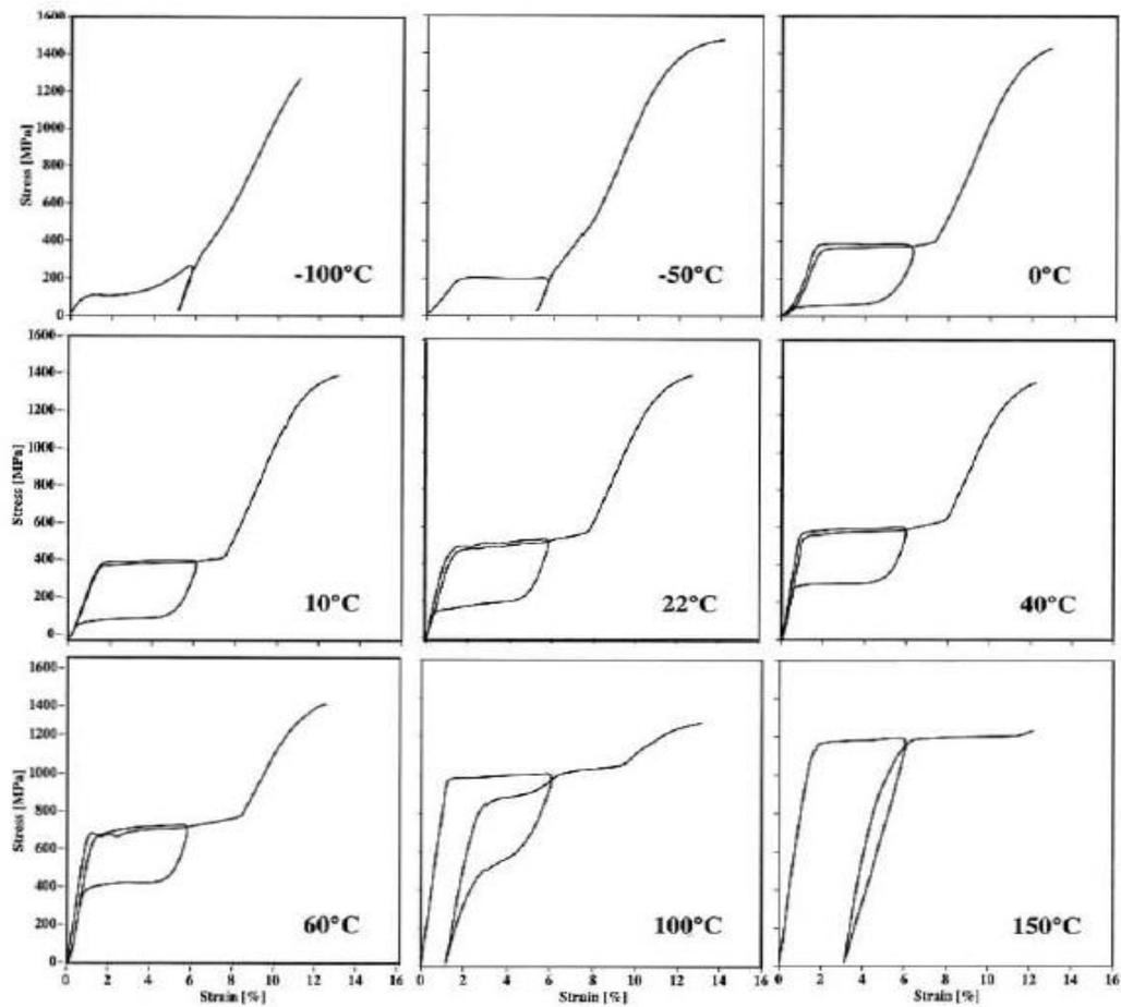
**Figure 1-4 Mechanical behavior of NiTiNOL at different temperature [7].**
