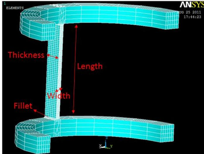
Figure 2-20 Uniform hexahedron meshing on the structure.
