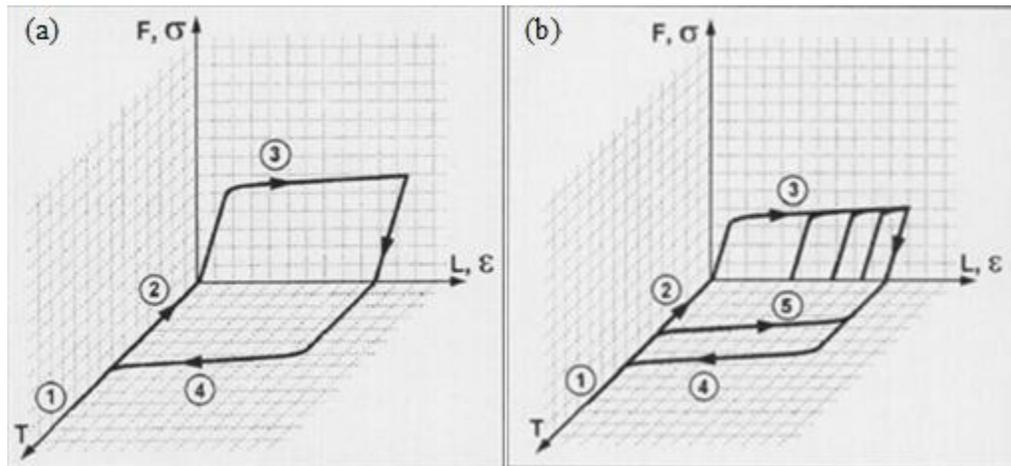
Figure 1-2 (a) One-way shape memory effect; (b) Two-way shape memory effect [3].
