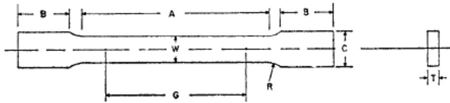
**Figure 2-5 Dog bone tension test specimen [94].**
