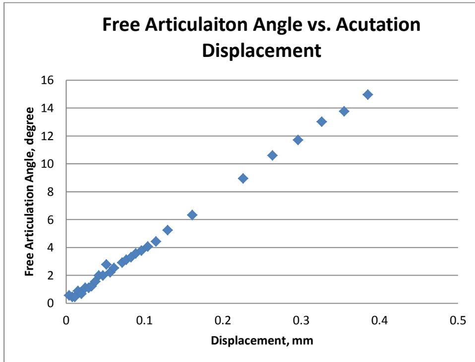
Figure 3-6 Free articulation angle versus tip actuation displacement which is a linear relationship.
