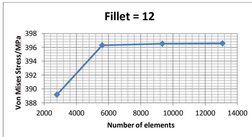
Figure 2-24 Maximum von Mises stress plotted against number of elements when fillet equals 12 and thickness changes from 3 to 16.
