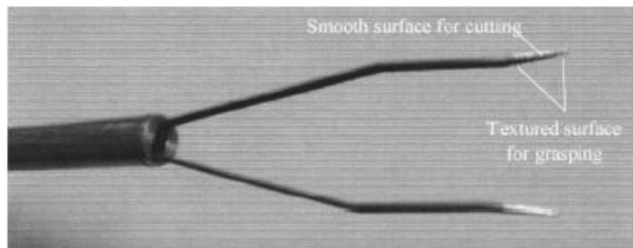
Figure 1-9 Compliant multifunctional scissors-forceps can performing cutting and grasping during surgery [23].
