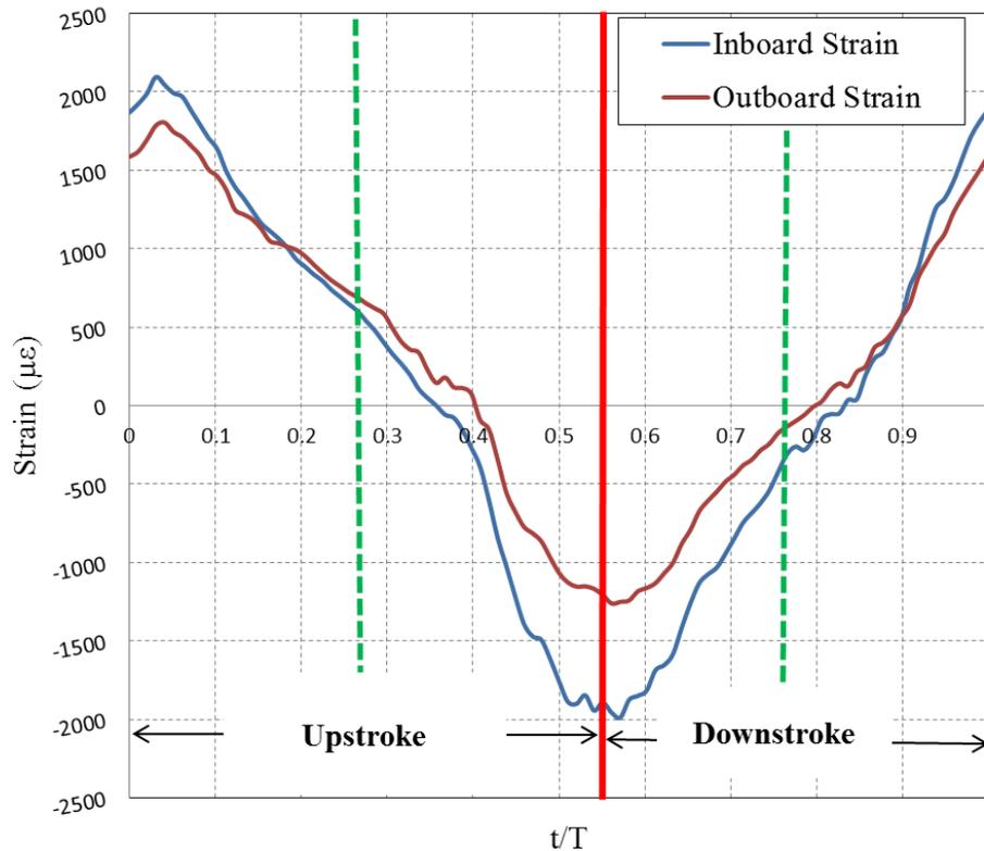
**Figure 4-4 Inboard and outboard strains at the location of the CS root and CS tip [105].**
