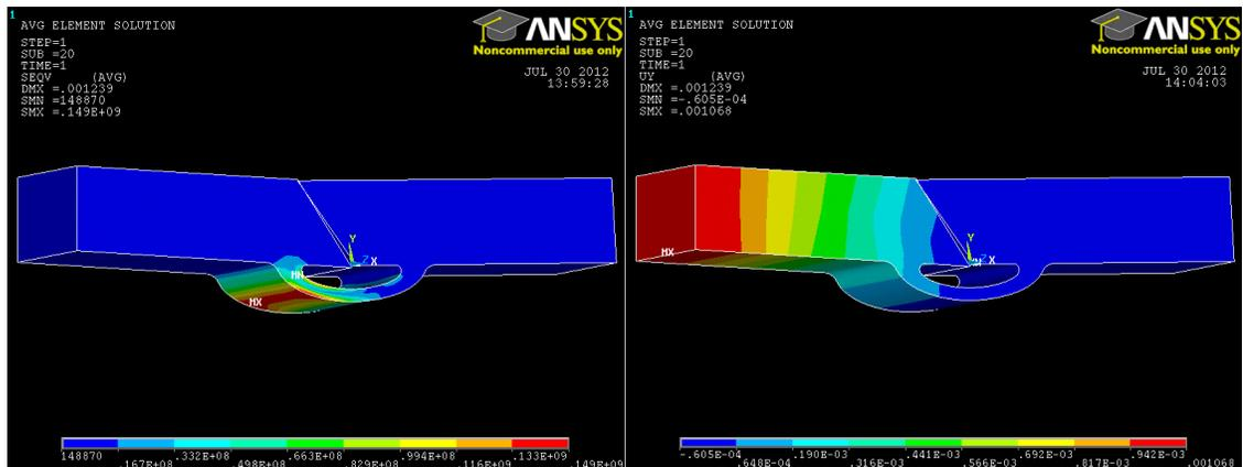
**Figure 4-12 Von Mises stress and Y-displacement plots for downstroke in NiTiNOL design.**
