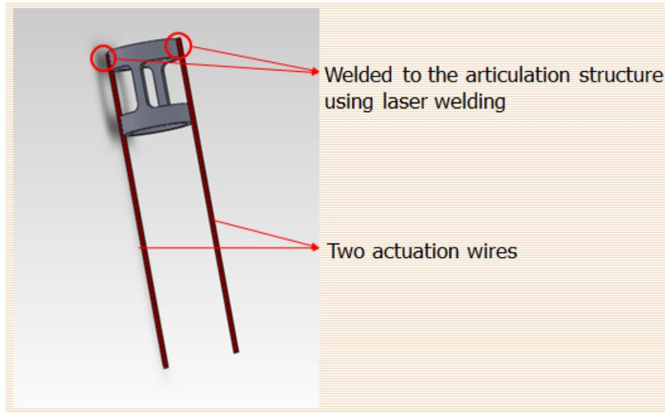
**Figure 5-1 Mechanical actuation for compliant articulation structure using wires.**
