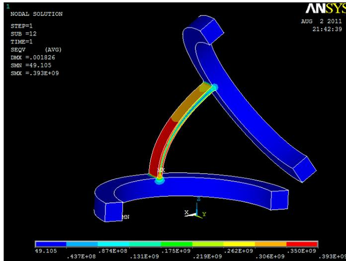
Figure 2-21 Von Mises stress plot of an articulation struture under free articulation.
