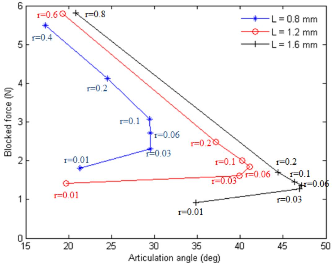
Figure 2-26 Blocked force and deflection angle for designs with three different lengths (represented by three different colors) and varying radius.
