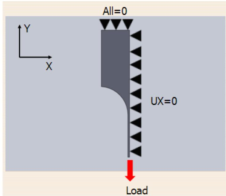
**Figure 2-6 Boundary and loading conditions for tension simulation.**
