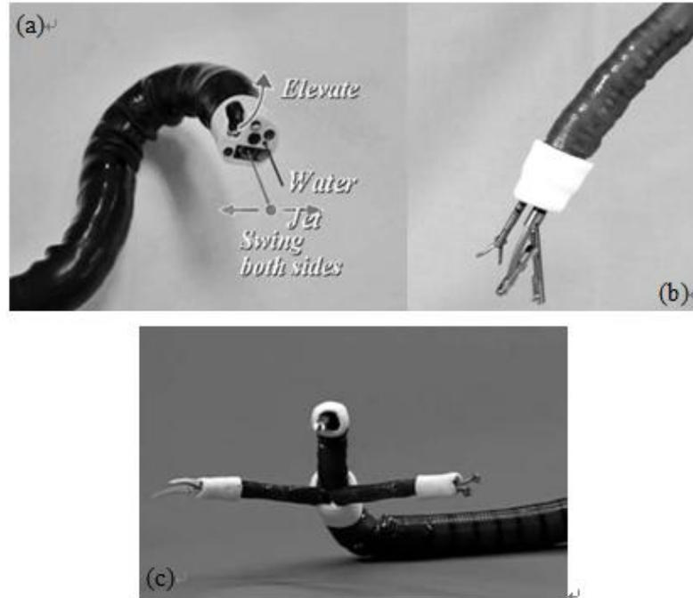
Figure 1-16 (a) The "R" scope from Olympus, Tokyo, Japan; (b) Transport from USGI medical, San Capistrano, CA, USA; (c) The Cobra from USGI medical, San Capistrano, CA, USA [43].
