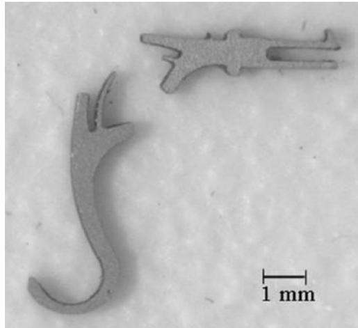
Figure 1-28 NiTiNOL robot leg fabricated using wire EDM [67].
