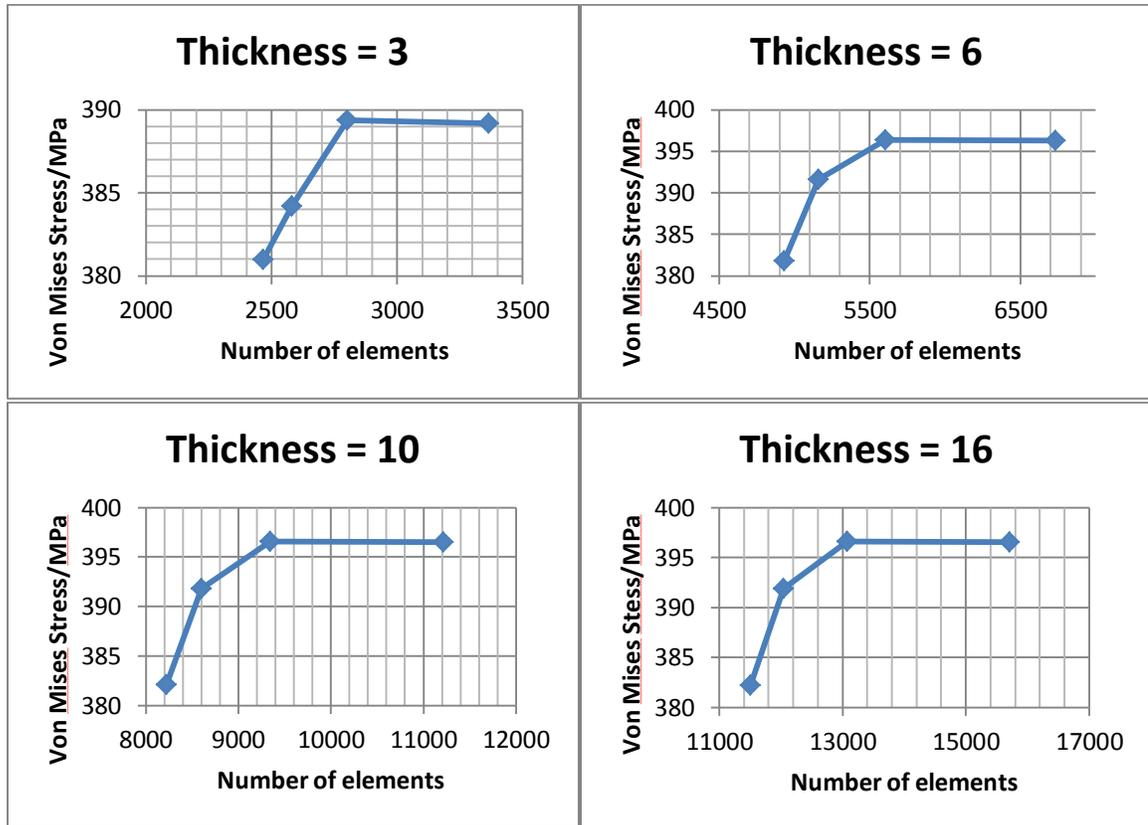
Figure 2-23 Maximum von Mises stress plotted against number of elements when both thickness and fillet are changing.
