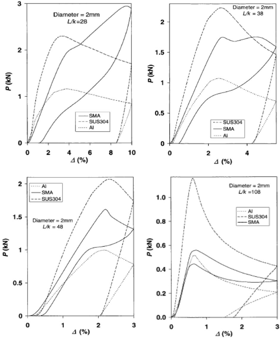
Figure 2-28 Experiment load-strain curve for different materials with different slenderness ratios [97].
