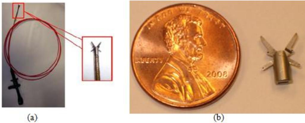
**Figure 1-20 (a) The multifunctional forceps are installed at the end of a endoscopy [48]; (b) The multifunctional forceps can both spread and grasp tissues [56].**
