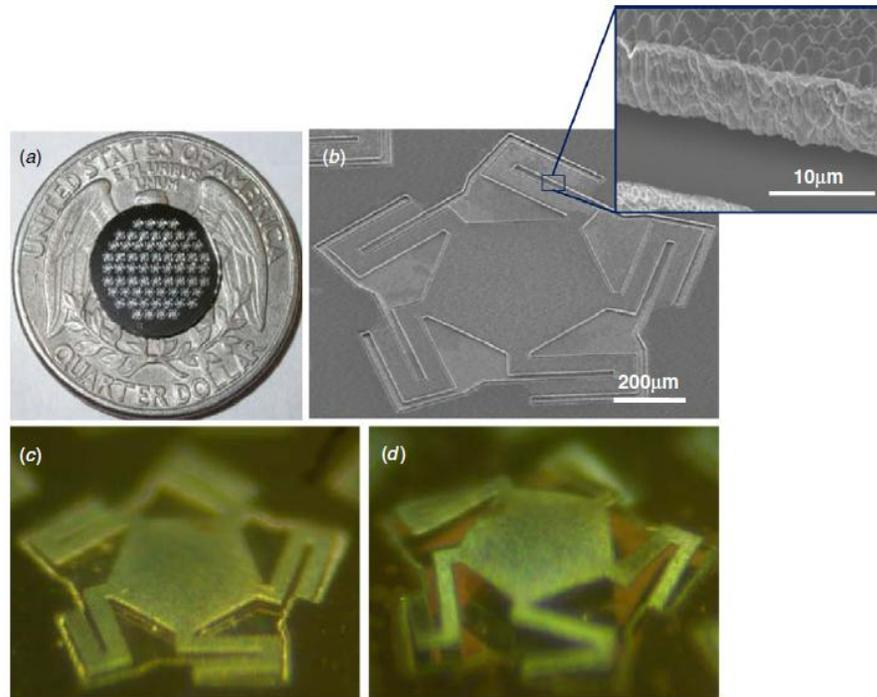
Figure 1-29 Arrays of NiTiNOL MEMS valve fabricated using bi-layer lift-off method [69].
