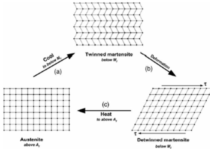
Figure 1-1 Microstructure variation during shape memory effect [4].
