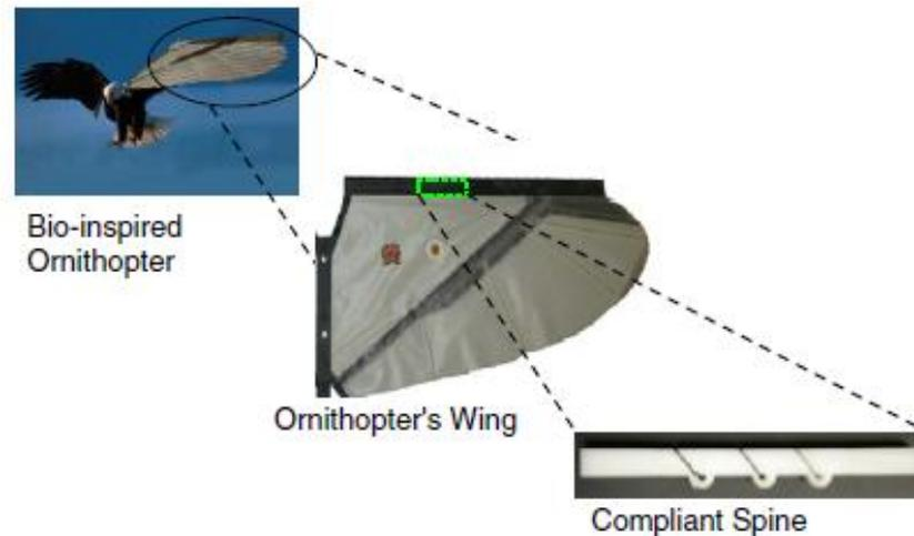
**Figure 1-26** The compliant spine is inserted into the leading edge spar to mimic the function of an avian wrist [65].
