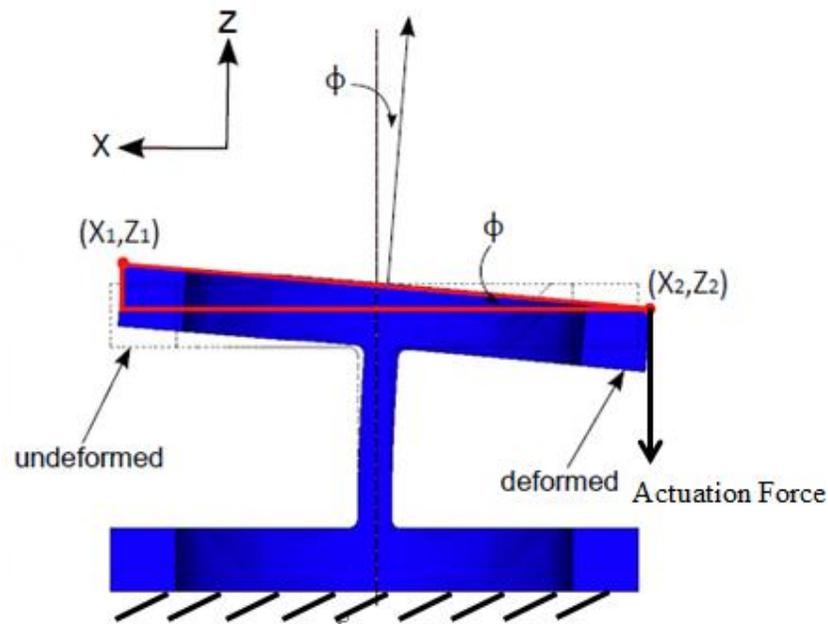
**Figure 2-18 In the half symmetry model, articulation angle ( $\phi$ ) is calculated based on the displacement of two key points in the model.**
