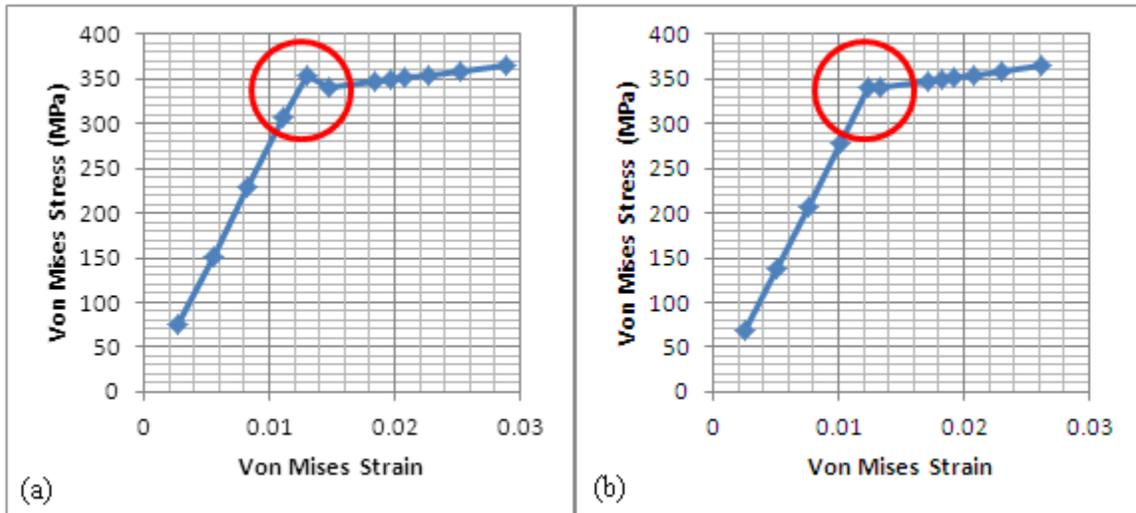
Figure 2-14 (a) Stress-strain curve of a bending cantilever beam with non-convergent response; (b) Stress-strain curve of a bending cantilever beam with convergent response.
