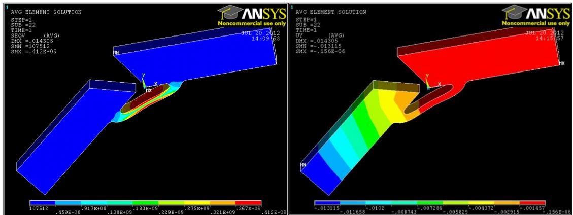
**Figure 4-11 Von Mises stress (left) and strain (right) plot of the one-joint ellipse compliant spine.**
