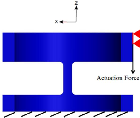
**Figure 2-19 In the half symmetry model, half blocked force is defined as the reaction force at the nodes shown in red.**
