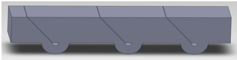
**Figure 4-1 Three-joint contact-aided compliant spine (courtesy: Yashwanth Tummala).**
