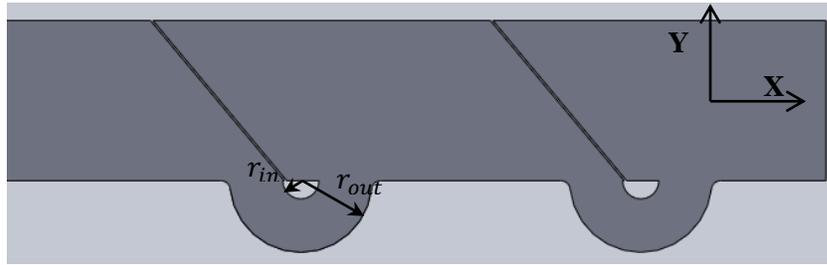
**Figure 4-6 A schematic of two-joint compliant spine.**
