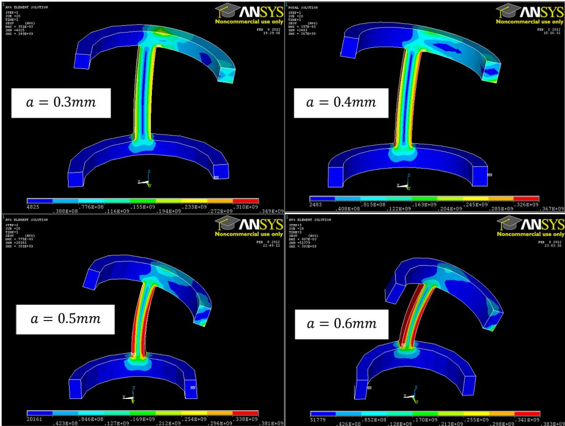
**Figure 2-27 Von Mises stress plot of articulation structures with different ring thickness.**
