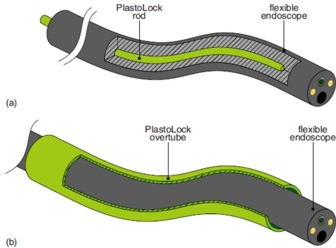
**Figure 1-22 (a) PlastoLock shaft embedded in a flexible endoscope; (b) PlastoLock overtube installed outside a flexible endoscope [59].**
