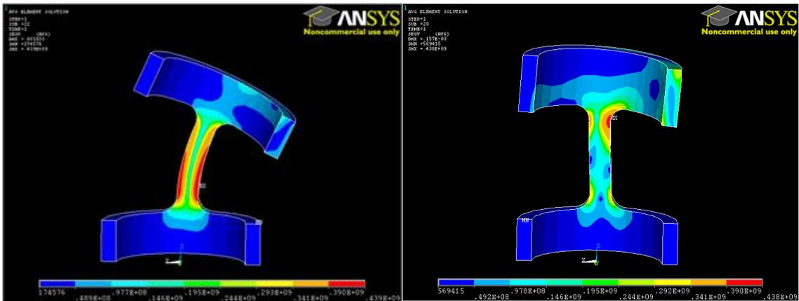
**Figure 2-30 Left: von Mises stress plot of half symmetry model in Free Articulation Angle case; Right: von Mises stress plot of half symmetry model in Blocked Force case.**
