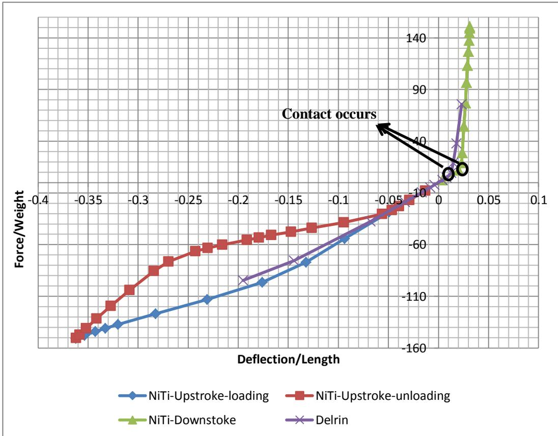
**Figure 4-13 Stiffness plots of both NiTiNOL compliant spine and Delrin compliant spine, showing its non-linear force-deflection curve.**
