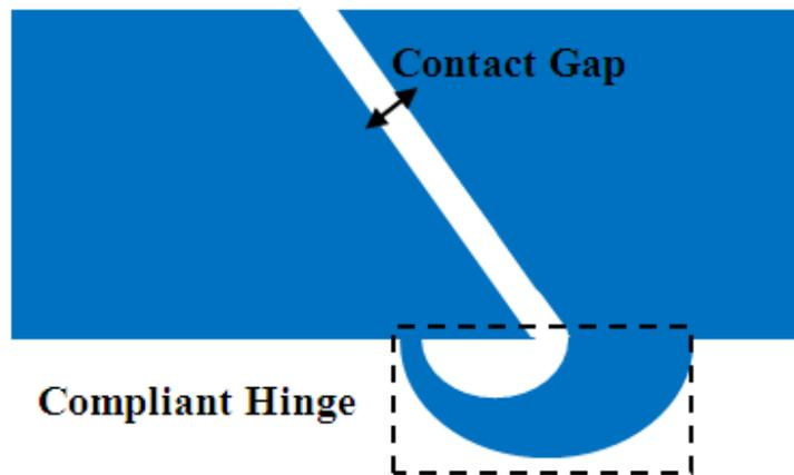
**Figure 1-27** Illustration of single compliant joint consisting of one contact gap and one compliant hinge (Courtesy: Yashwanth Tummala).
