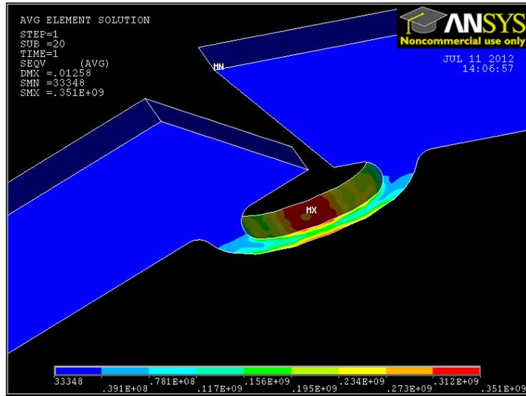
**Figure 4-9 Von Mises stress plot of compliant spine with elliptical joint.**
