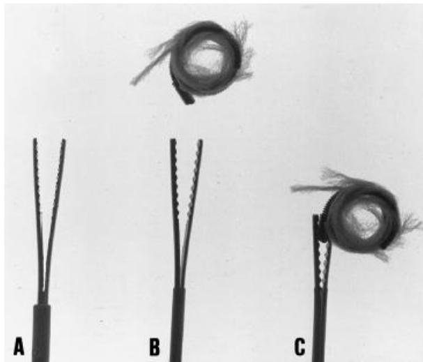
Figure 1-7 NiTiNOL micro-forceps are retrieving objects in experiment [16].
