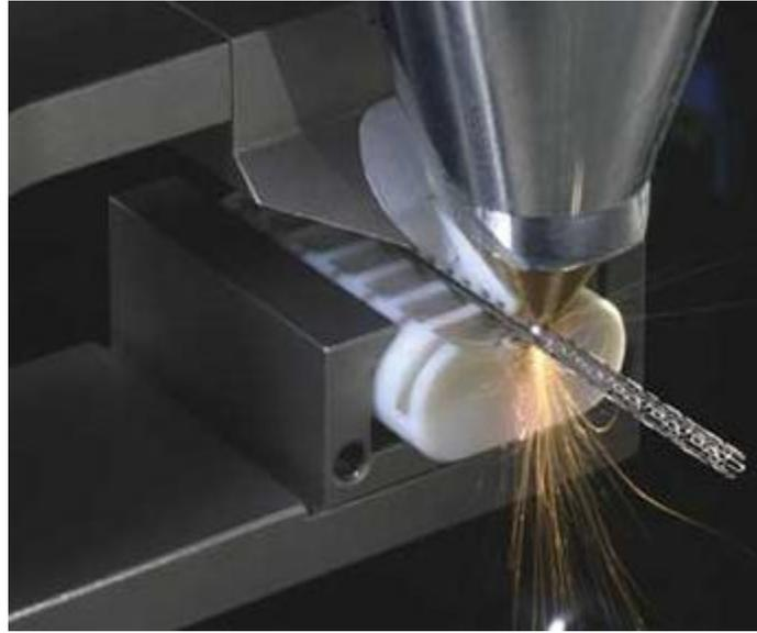
**Figure 1-30 NiTiNOL stent is cut from a tube using high-precision laser processing [71].**
