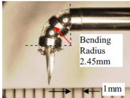
**Figure 1-25 Micro manipulator using ball joint in bending position [62].**
