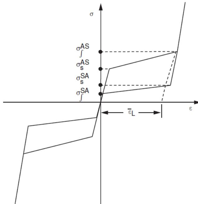
**Figure 2-3 Superelastic Model in ANSYS [90].**
