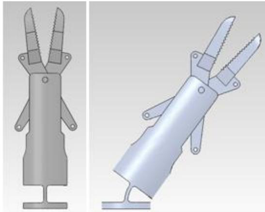
**Figure 2-1 A surgical tool tip mounted on the compliant articulation structure. Articulation increases the functional space and improves dexterity of the surgical instrument.**
