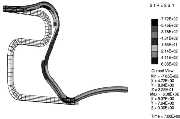
Fig. 7. Orthodontic archwire: deformed mesh in the maximum deformed configuration.
