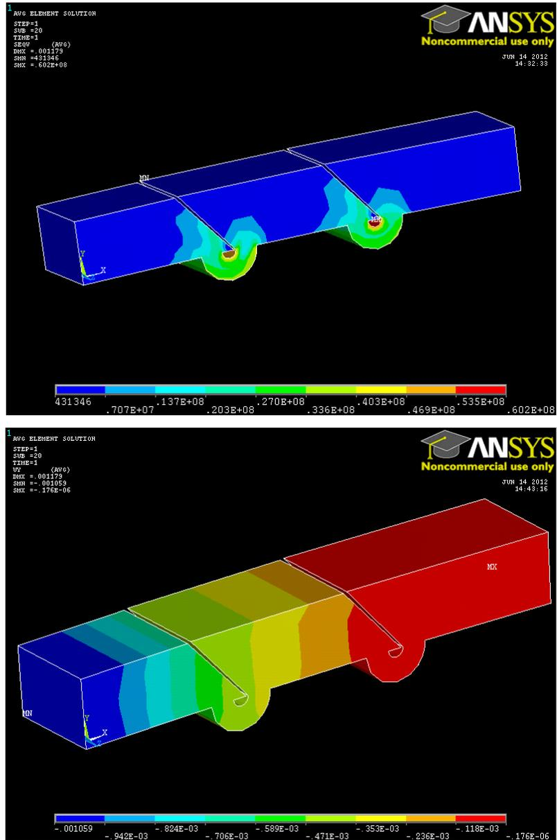
Figure 4-7 Von Mises stress and vertical displacement of compliant spine #1.
