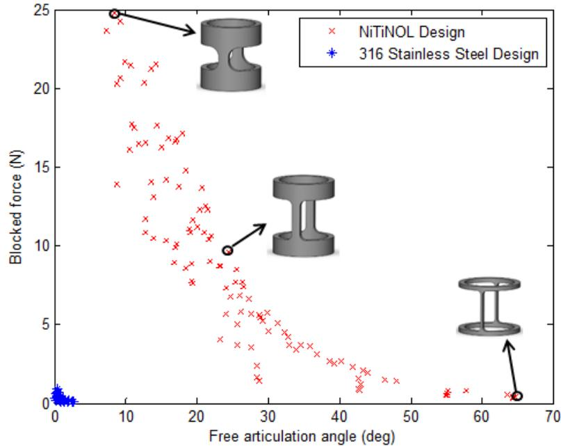
**Figure 2-29 Blocked force and free articulation angle results of the family of designs, with comparison to 316 stainless steel results.**
