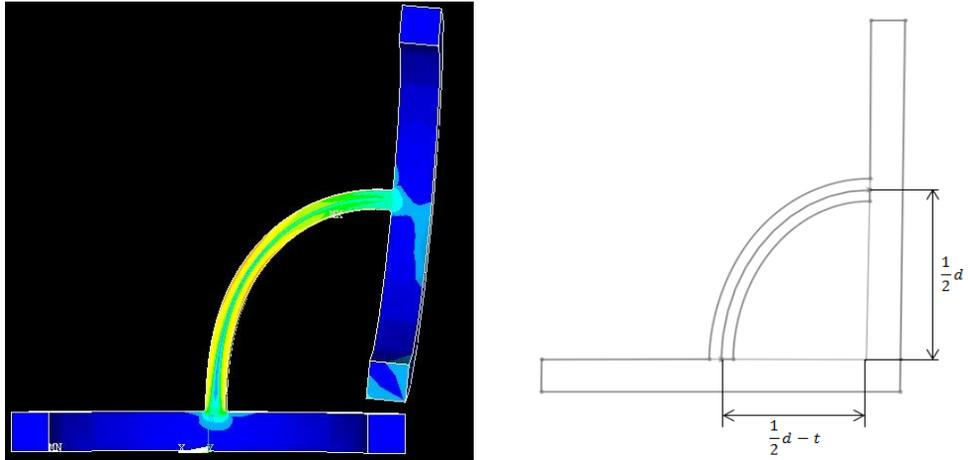
**Figure 2-25 Left: illustration of an articulation structure bending up to 90°; Right: an ellipse model is fitted to calculate the maximum length.**
