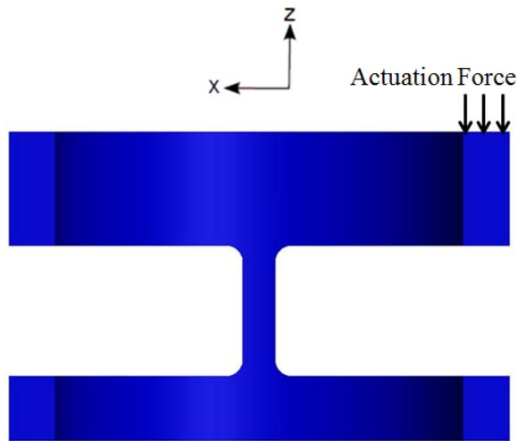
**Figure 3-2 Loading condition in experiment, taken into consideration during modified FEA.**
