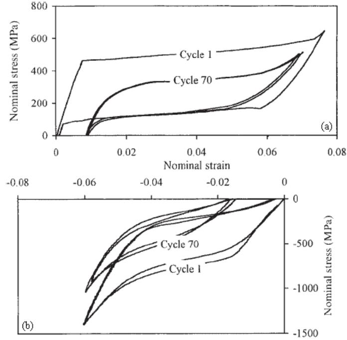
**Figure 2-4 (a) Stress-strain curve at tension test; (b) Stress-strain curve at compression test [93].**
