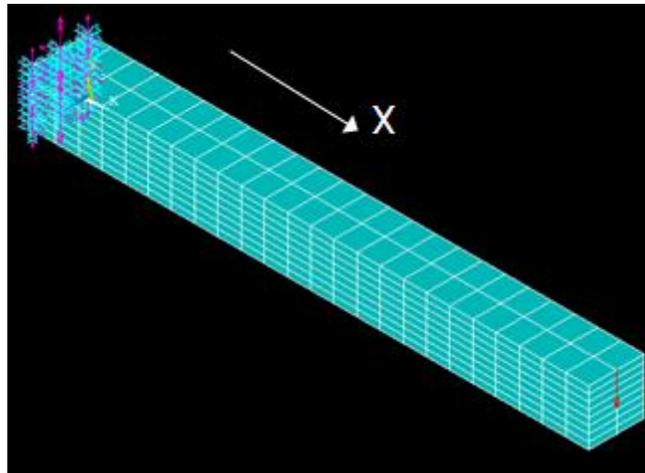
Figure 2-15 A cantilever beam is uniformly meshed in ANSYS.
