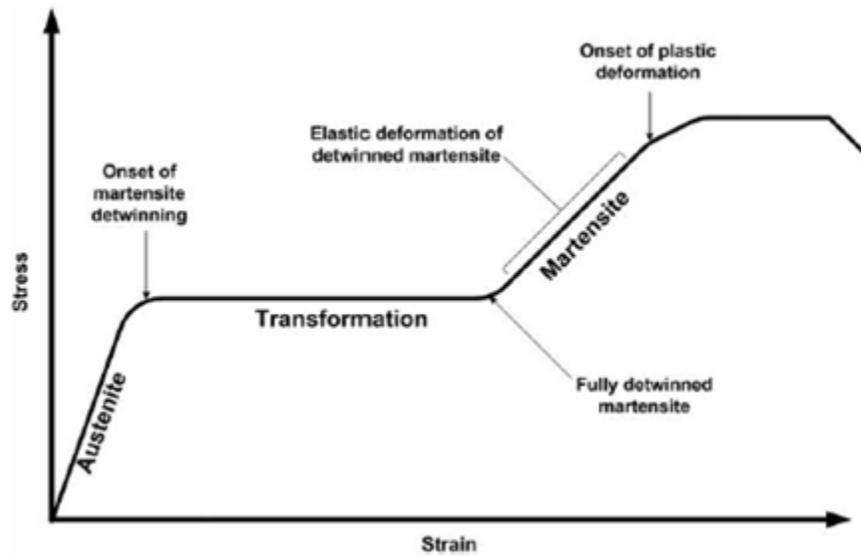
**Figure 1-3 Phase transformation during superelastic effect [4].**
