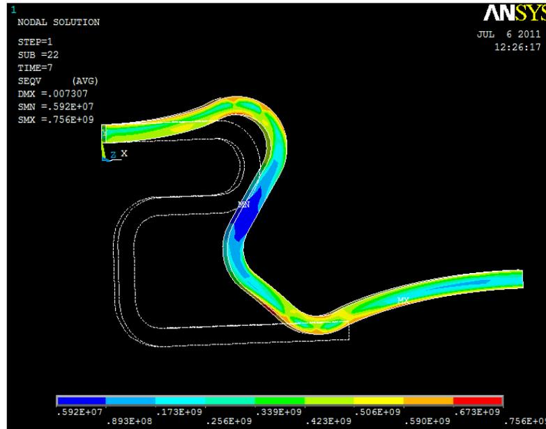
**Figure 2-12 Von Mises stress plot of orthodontic wire simulation.**
