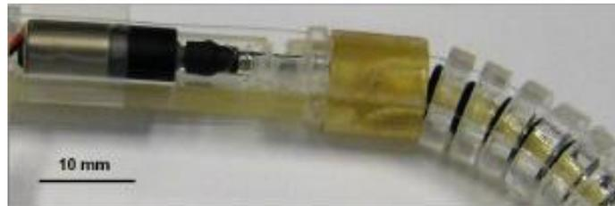
**Figure 1-23 Spine-like articulation system using motor actuation [60].**
