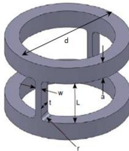
**Figure 2-2 Geometric model of the compliant articulation structure, used to develop families of different designs.**
