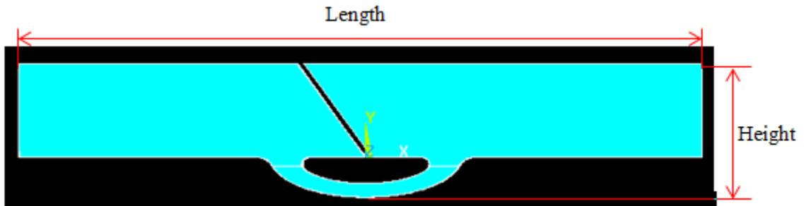
**Figure 4-10 One-joint compliant spine with elliptical hinge.**
