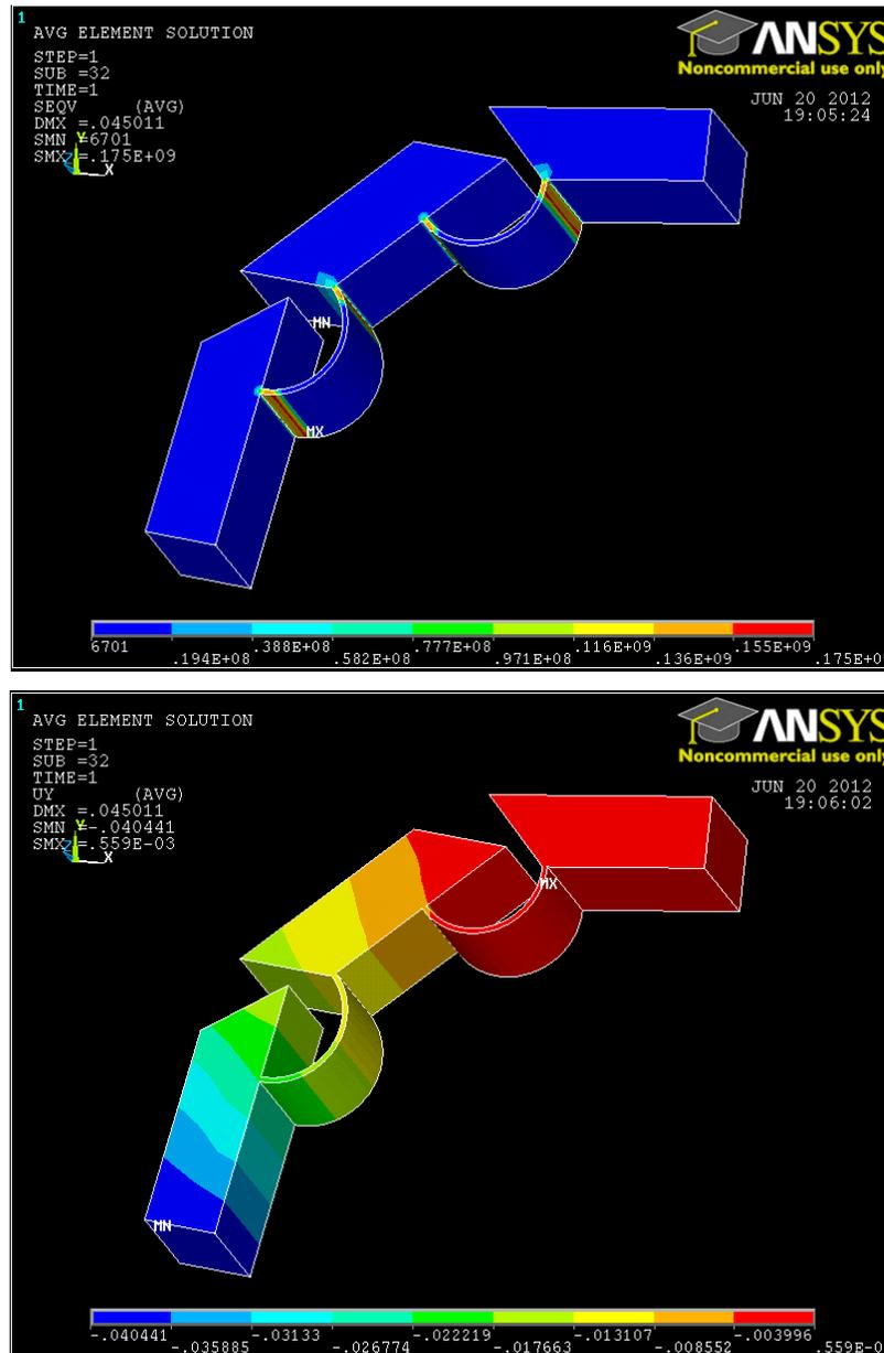
Figure 4-8 Von Mises stress and deflection plot of two-joint compliant spine #2 using superelastic NiTiNOL.
