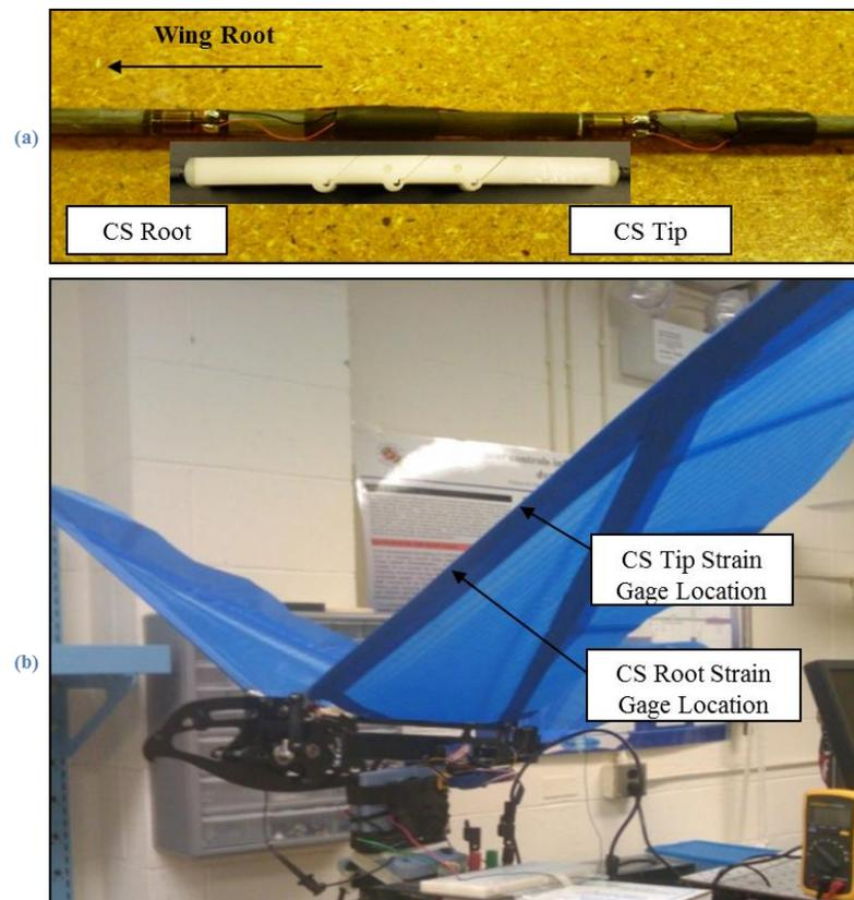
Figure 4-3 (a) Strain gages mounted on the leading edge spar at the locations of the CS root and tip. (b) Experiment setup for measuring the aerodynamic loads on the CS [105].
