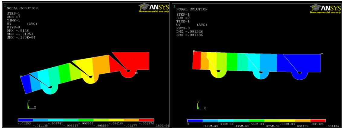
**Figure 4-2 (Left) Compliant spine deformed shape during upstroke; (Right) Compliant spine deformed shape during downstroke.**
