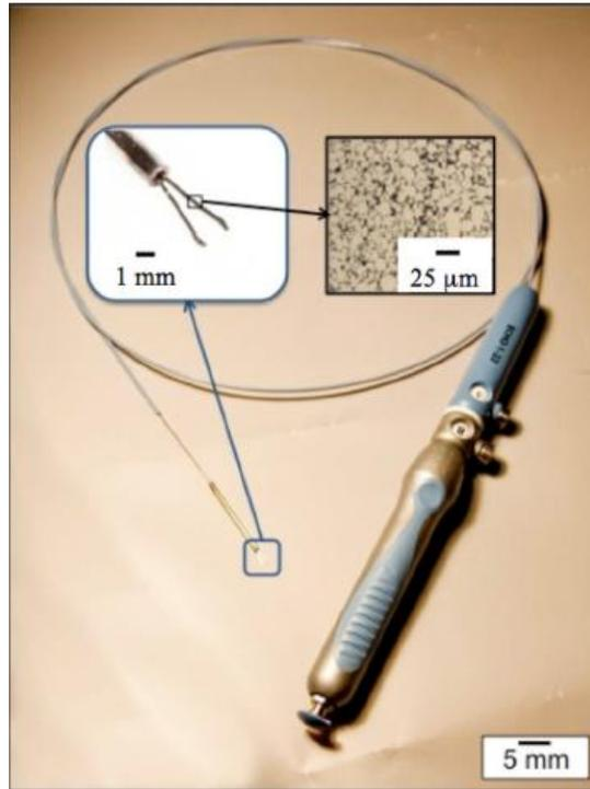
**Figure 1-11 Assembled meso-scale forceps prototype for NOTES [25].**
