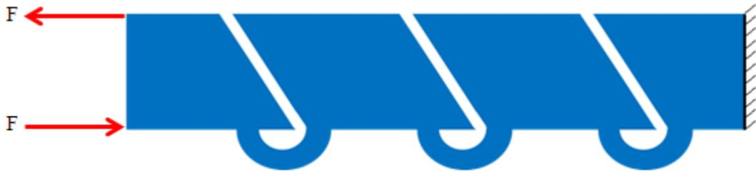
**Figure 4-5 Boundary and loading condition for compliant spine in upstroke.**
