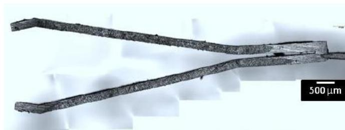
**Figure 1-21 Compliant forceps can fit into 1-mm diameter scope [57].**
