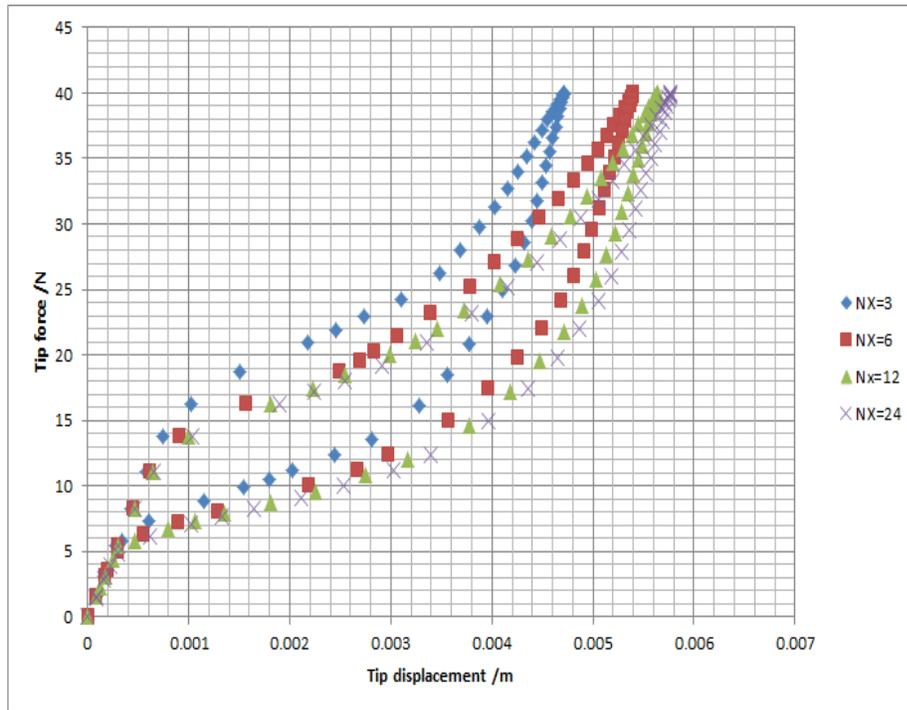
Figure 2-10 Tip force vs. tip displacement results with different number of elements.
