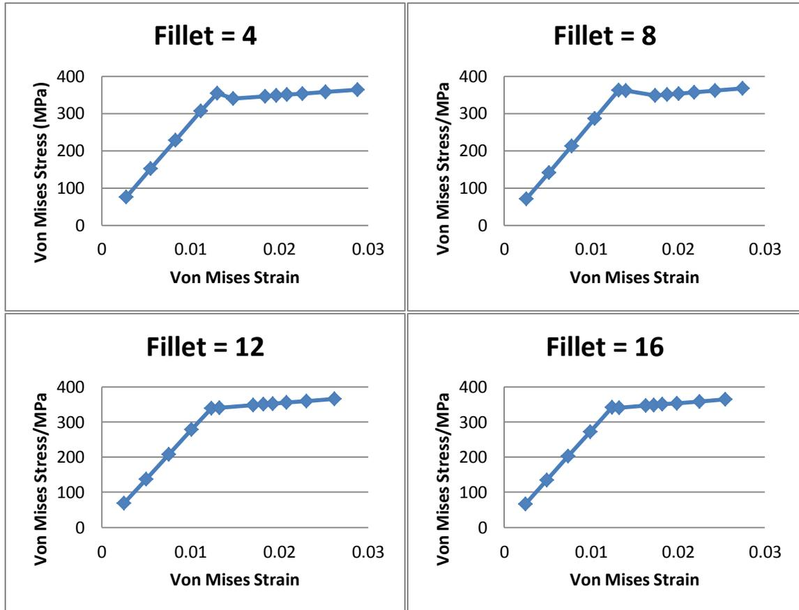
Figure 2-22 Stress-strain plot when the number of elements along fillet is changing.
