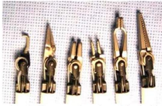
**Figure 1-19 Modified tool tips originally from Laprotek laparoscopic instruments [54].**
