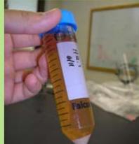
Centrifuge tubes for 15 minutes at ~5,000 rpm to pellet the endospores. Pour off the supernatant.
