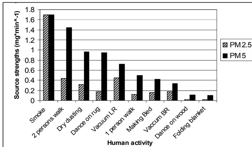
**Figure 2 Source strength of particle resuspension by human activity (Ferro 2002)**
