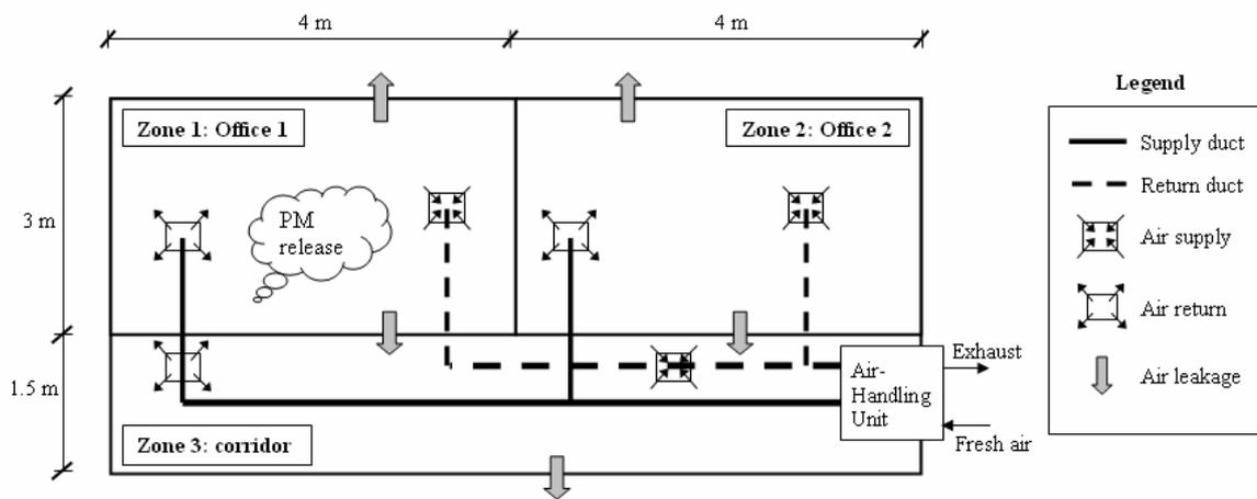
**Figure 59 a three-zone office building equipped with HVAC system**
