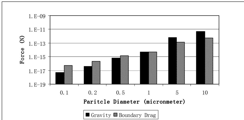
**Figure 9 Comparison of particle gravitational force and boundary drag force**
