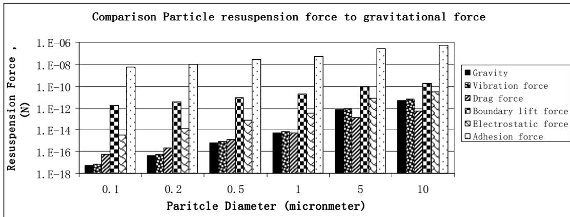
**Figure 17 Comparison of force components acting on surface particles**
