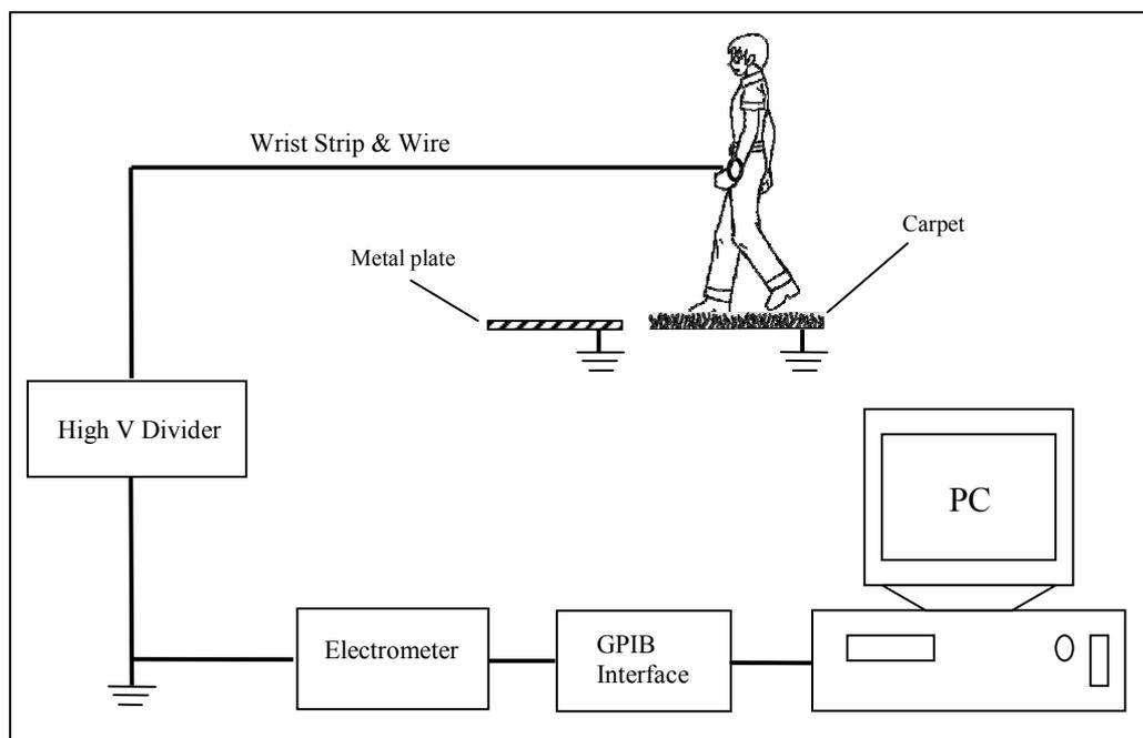
**Figure 38 Measurement system of human body voltage during walking**
