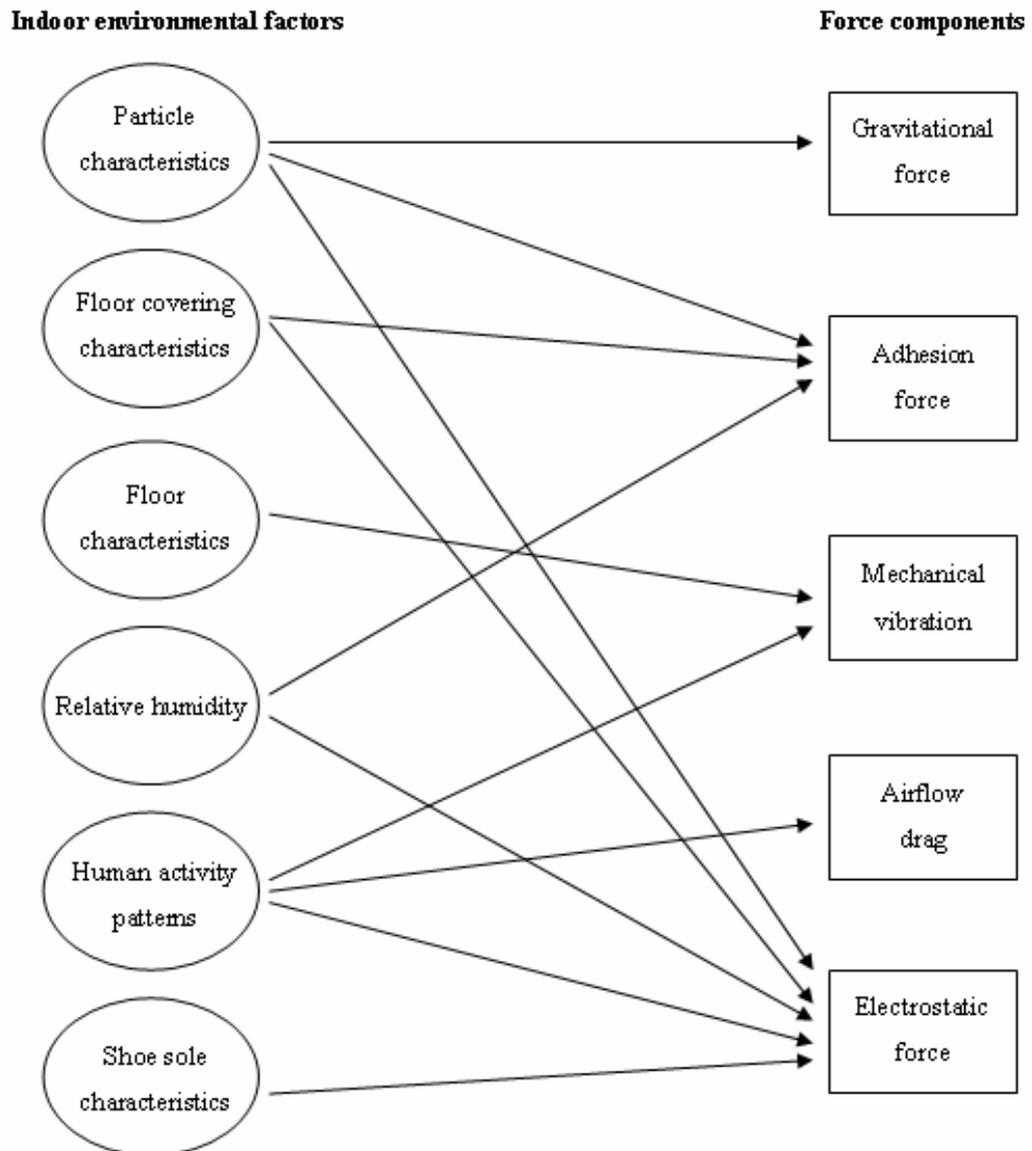
**Figure 4 Factors influencing force components on residing particles**
