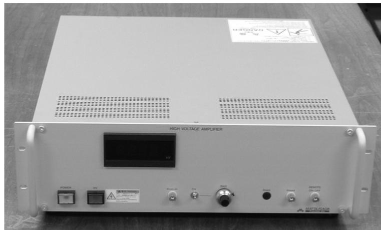
**Figure 49 High voltage amplifier**
