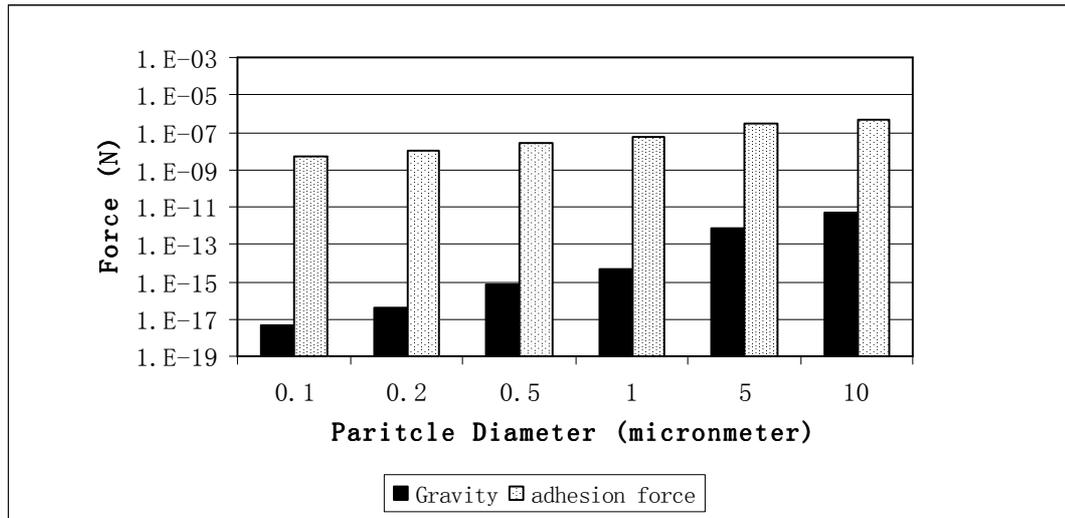
**Figure 5 Comparison between adhesion force and gravitational force**
