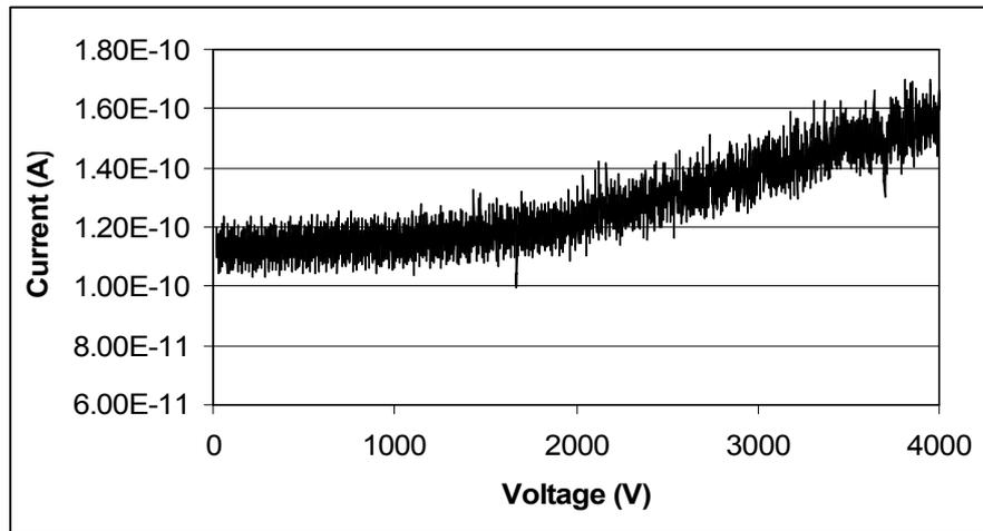
**Figure 20 Measured charging current in Alumina-Vinyl detachment experiment**
