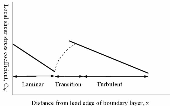
**Figure 8 Influence of location on a flat surface on the local skin friction coefficient**
