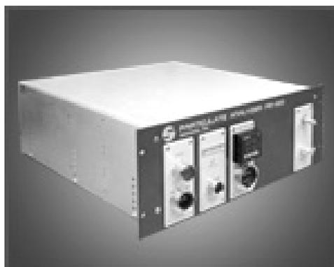
**Figure 46 PM-300 optical particle counter**
