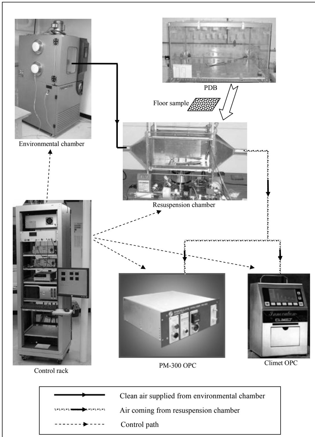
**Figure 50 Operation flow chart of resuspension chamber system**
