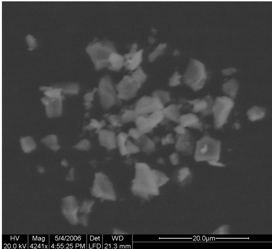
**Figure 26 Surface alumina particles under SEM**
