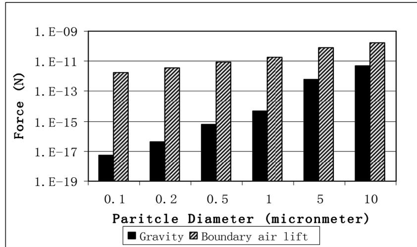
**Figure 10 Comparison of particle gravitational force and boundary lift force**
