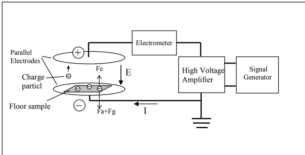
**Figure 19 Electrostatic detachment method for particle adhesion force measurement**
