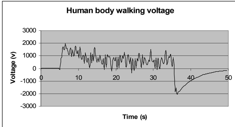
**Figure 39 Body voltage recording for a walking trial**
