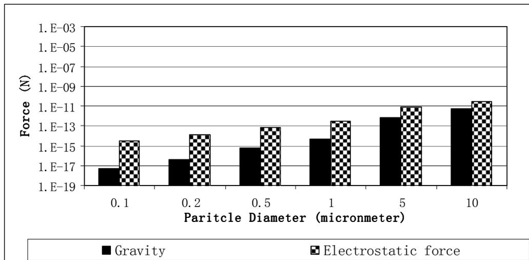
**Figure 15 Comparison of particle gravity and electrostatic force**
