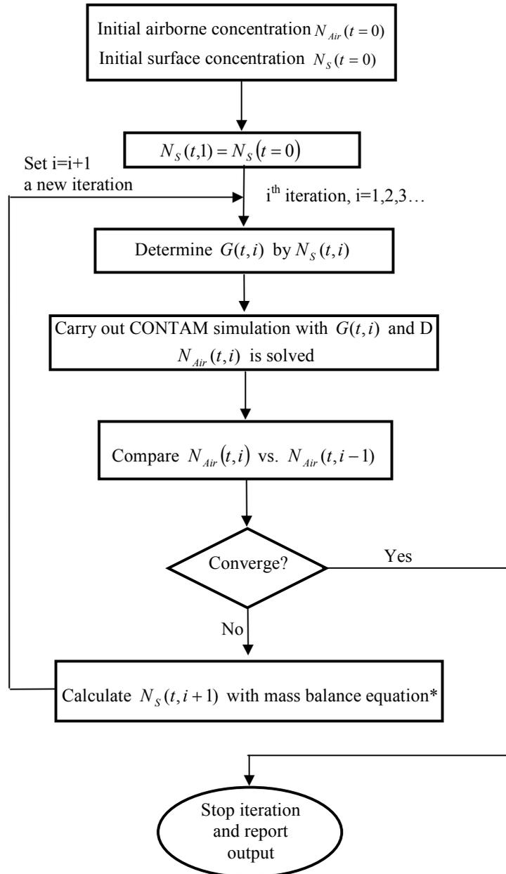
**Figure 58 Algorithm of iteration method for transient simulation**
