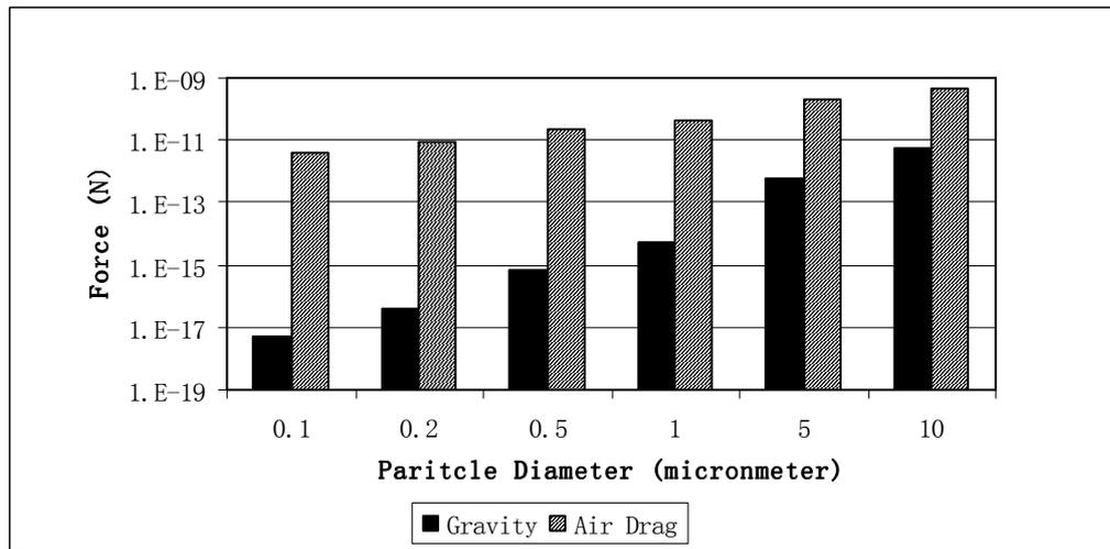
**Figure 7 Comparison of particle gravitational force and air drag force**
