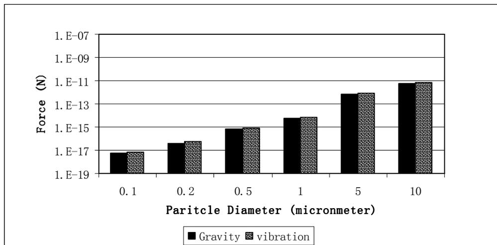
**Figure 6 Comparison between vibration force and gravitational force**
