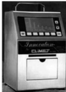
**Figure 47 Spectro .3 particle counter**
