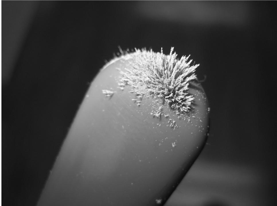
**Figure 16 Roach dusts attaching to the charged plastic spoon handle**
