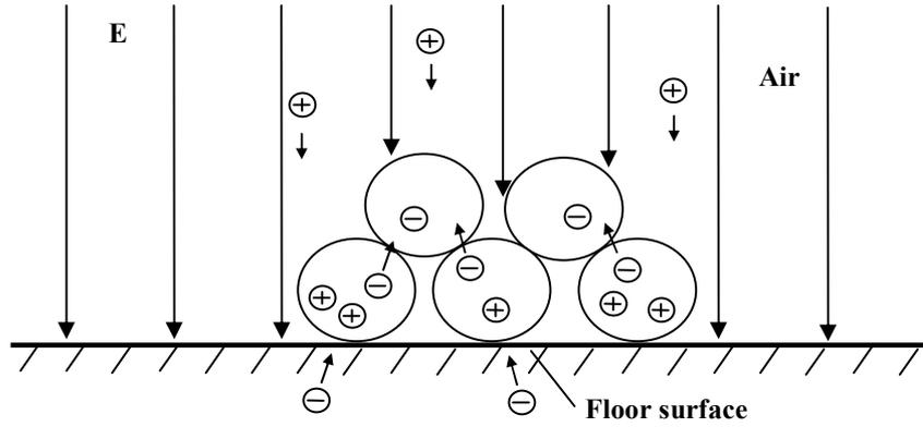
**Figure 13 Induction charges on particles residing on insulating floor**
