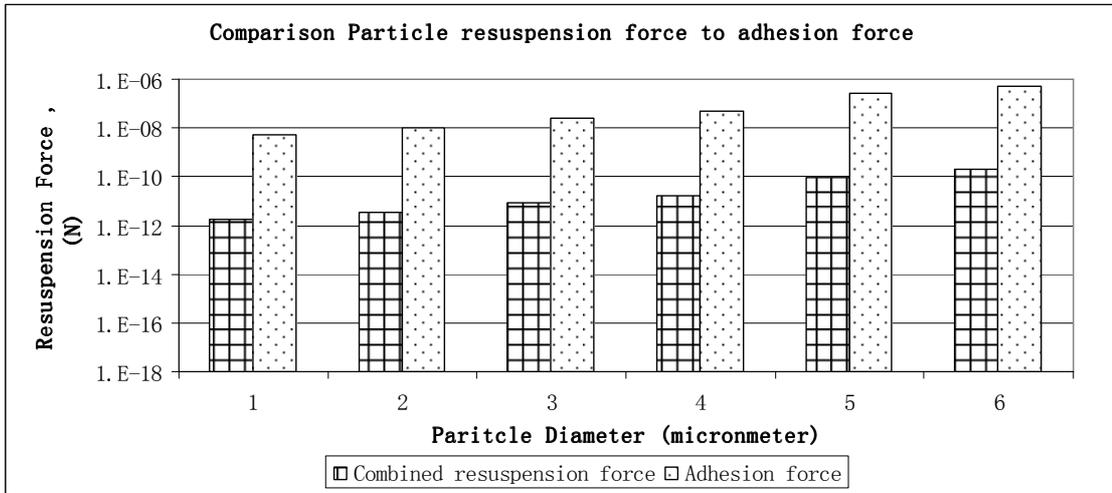
**Figure 18 Comparison particle resuspension force to adhesion force**
