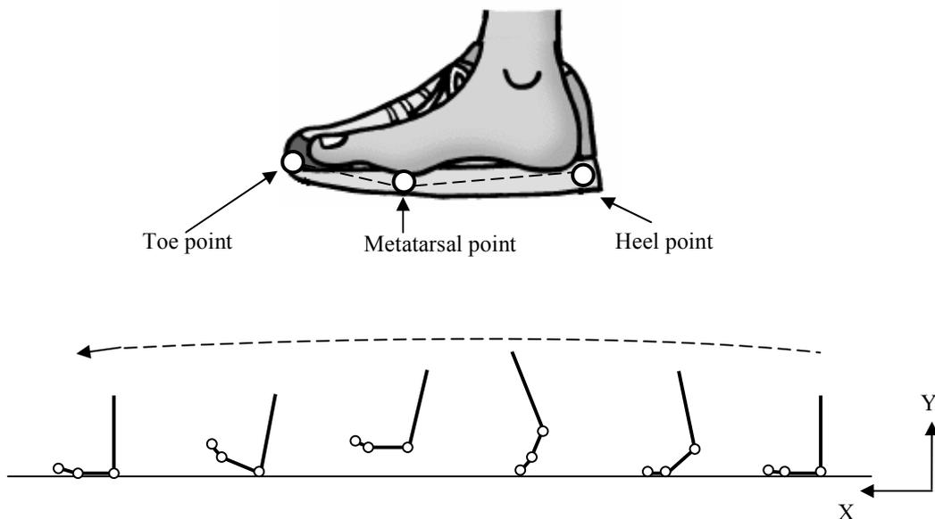
**Figure 32 Three points to measure the shoe bottom position to the floor surface**
