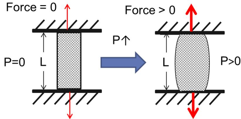
Figure 2-4: Blocked force test diagram.
