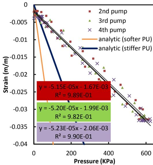
Figure B-5: Small braided tubes 40° free strain test A-3.
