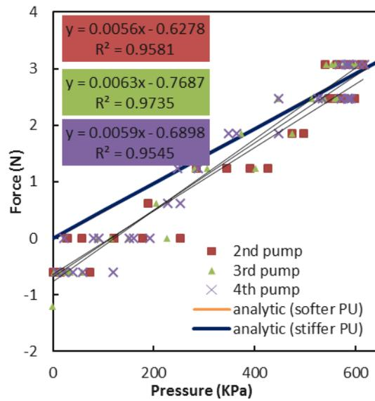
Figure **B-17**: small braided tubes 40° blocked force test A-4.
