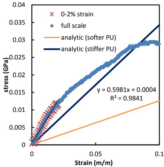
Figure B-21: Small braided tubes 24° axial modulus test A-4.
