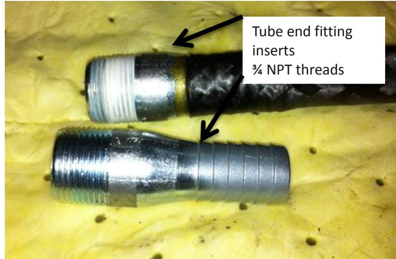
Figure 2-1: Threaded tube fittings.
