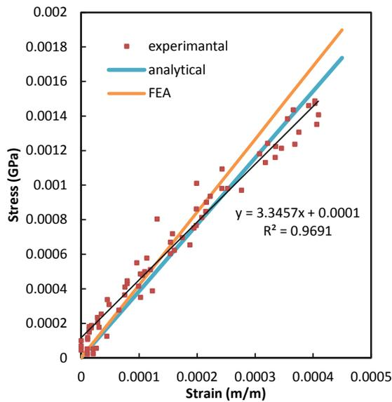
Figure 2-19: 38.3° bi-layer axial modulus.
