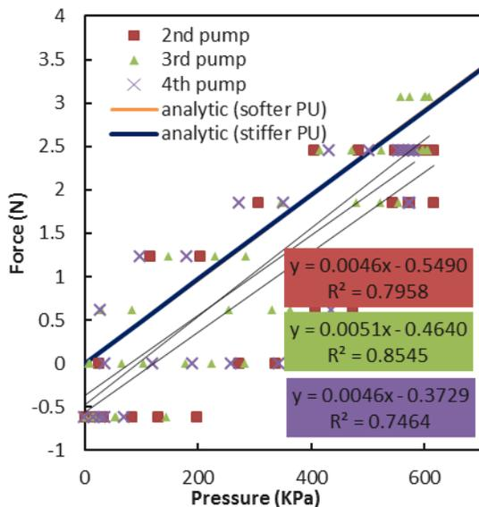
Figure B-15: small braided tubes 40° blocked force test A-2.
