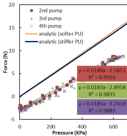
Figure **B-18**: Small braided tubes 24° blocked force test C-1.
