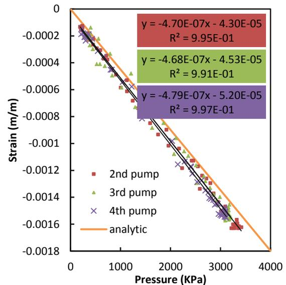
Figure 3-4: Bonded tube free strain test #2.
