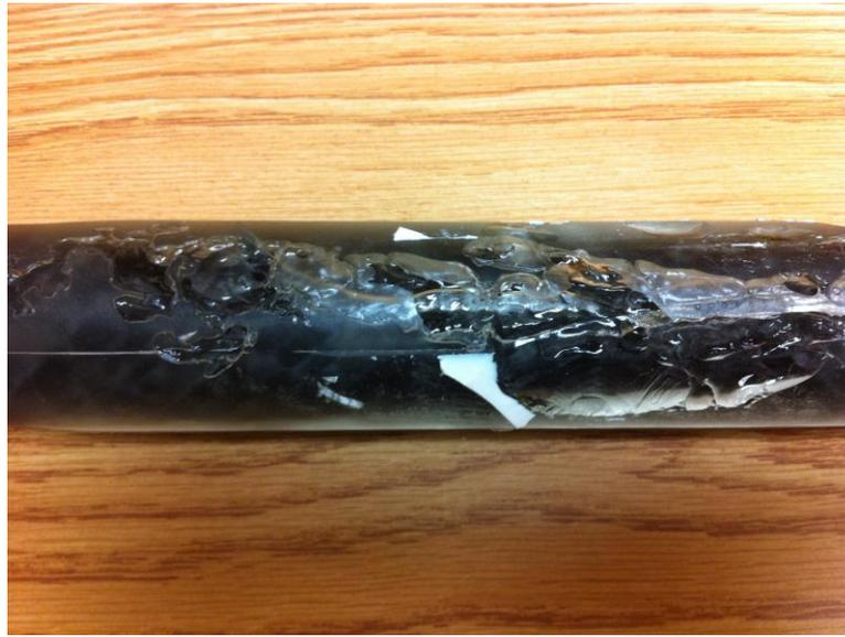
Figure 3-1: Photograph of thick FMC tube cast in epoxy.
