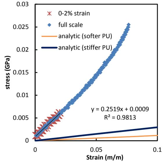
Figure B-23: Small braided tubes 40° axial modulus test A-3.
