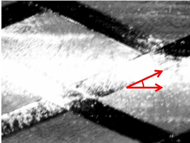
Figure 4-4: Photomicrograph of lower angle braided tube.
