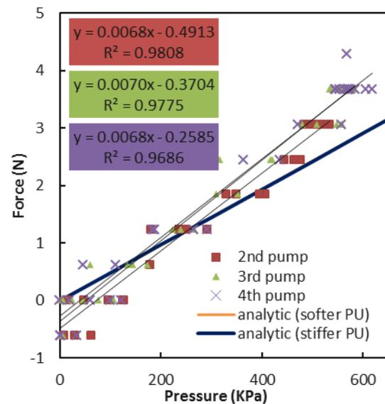
Figure 4-16: Small braided tubes 40° blocked force test A-1.
