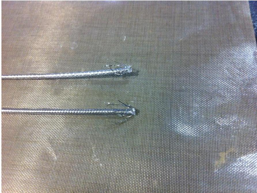
Figure 4-8: Photograph of exposed wire reinforcement prior to attaching end fittings for the third round of braided tube tests.
