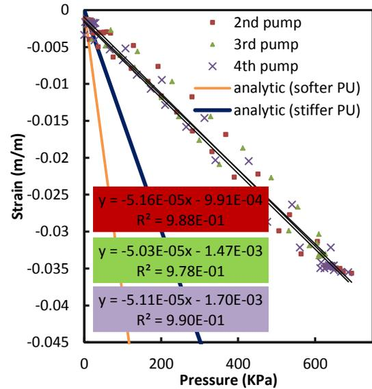
Figure B-9: Small braided tubes 40° free strain test B-2.
