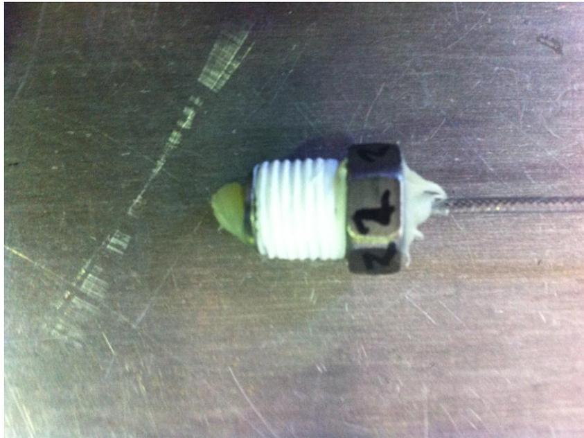
Figure 4-6: Photograph of end fitting bonded to a small braided tube.
