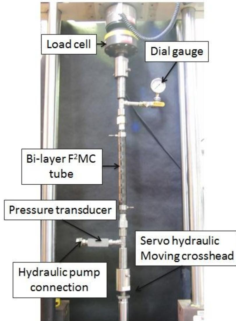
Figure 2-2: Test apparatus for large tubes.
