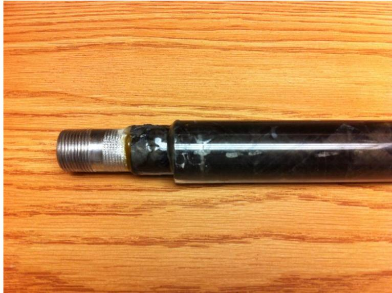
Figure 3-2: FMC tube bonded into a polycarbonate tube, with threaded end fitting in place.
