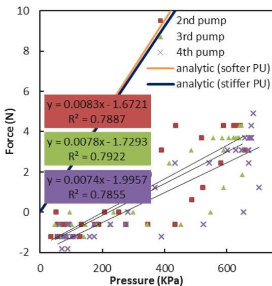
Figure B-13: Small braided tubes 24° blocked force test A-3.
