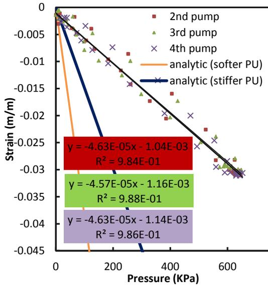
Figure B-8: Small braided tubes 40° free strain test B-1.
