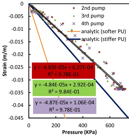
Figure B-6: Small braided tubes 24° free strain test B-1.
