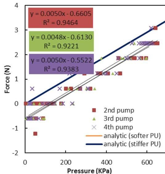
Figure B-16: small braided tubes 40° blocked force test A-3.
