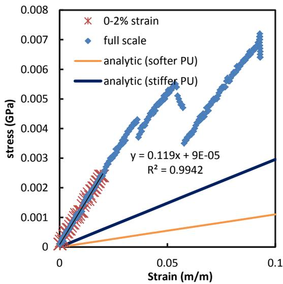
Figure **B-27**: Small braided tubes 40° axial modulus test C-1.
