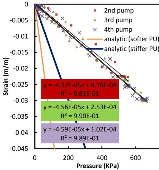
Figure B-11: Small braided tubes 40° free strain test C-1.
