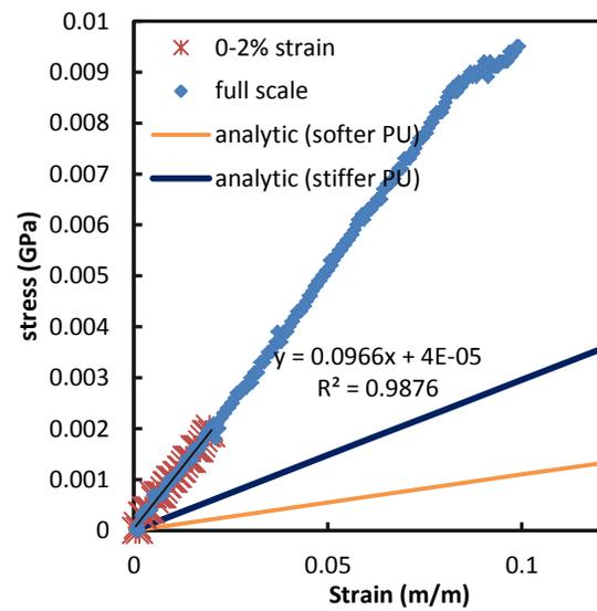
Figure **B-28**: Small braided tubes 40° axial modulus test C-2.
