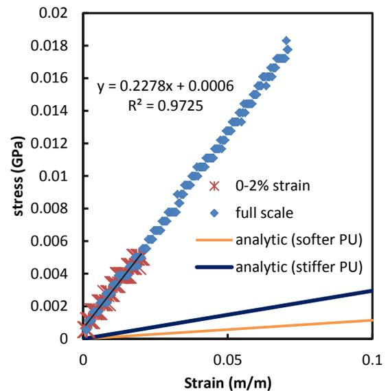
Figure 4-18: small braided tubes 40° axial modulus test A-1.
