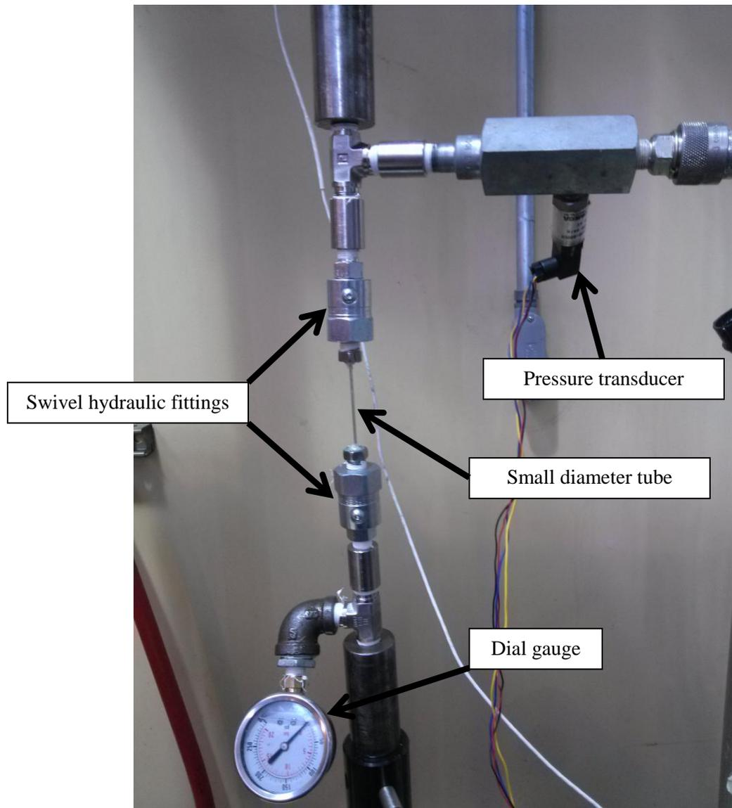
Figure 4-12: Close-up photograph of the blocked force and axial modulus test setups for braided tubes.
