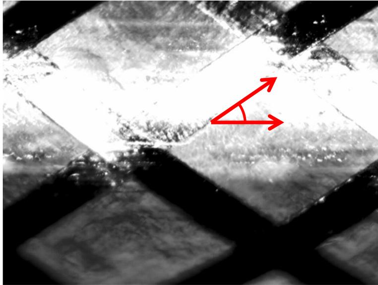
Figure 4-3: Photomicrograph of higher angle braided tube.
