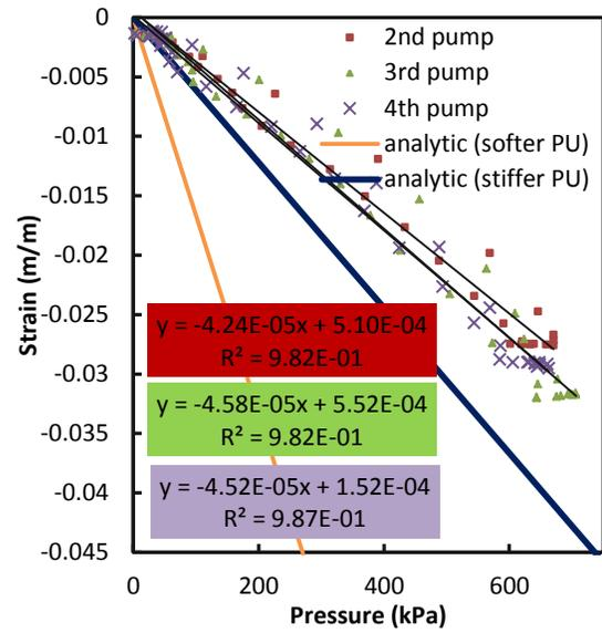
Figure B-7: Small braided tubes 24° free strain test B-2.
