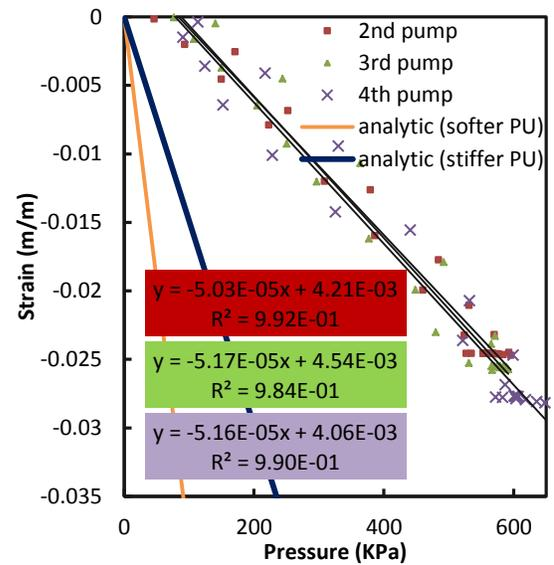
Figure 4-13: Small braided tubes 24° free strain test A-1. Figure 4-14: small braided tubes 40° free strain test A-4.
