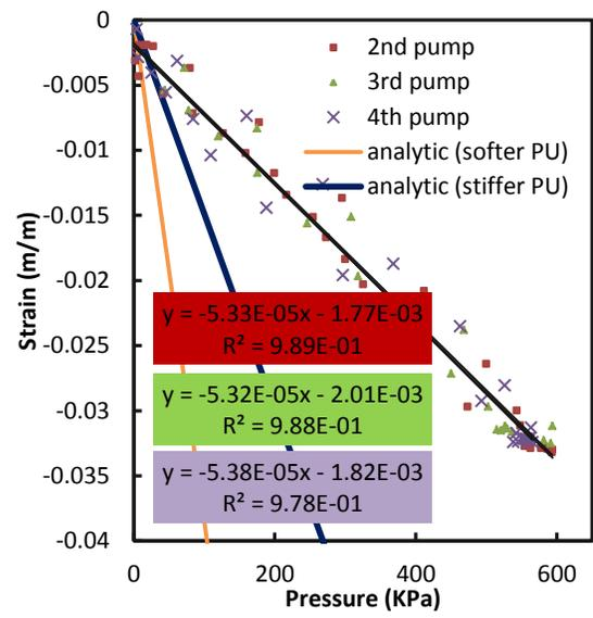
Figure B-4: Small braided tubes 40° free strain test A-2.
