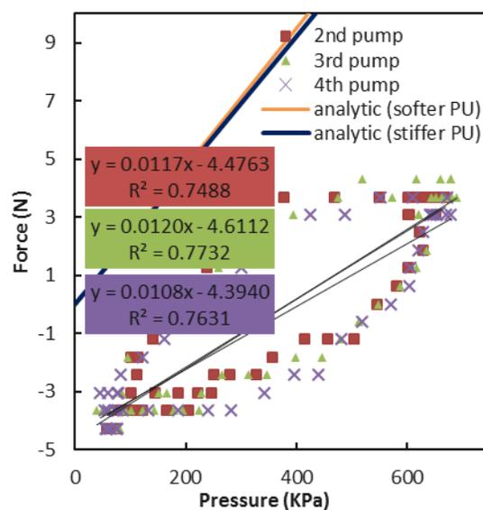
Figure B-14: Small braided tubes 24° blocked force test A-4.
