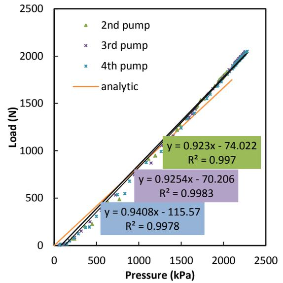
Figure 2-13: 35° thick-walled blocked force.
