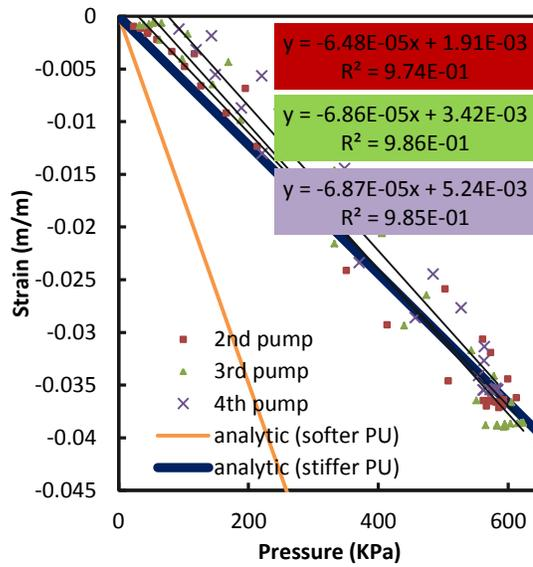
Figure B-1: Small braided tubes 24° Free strain test A-3.
