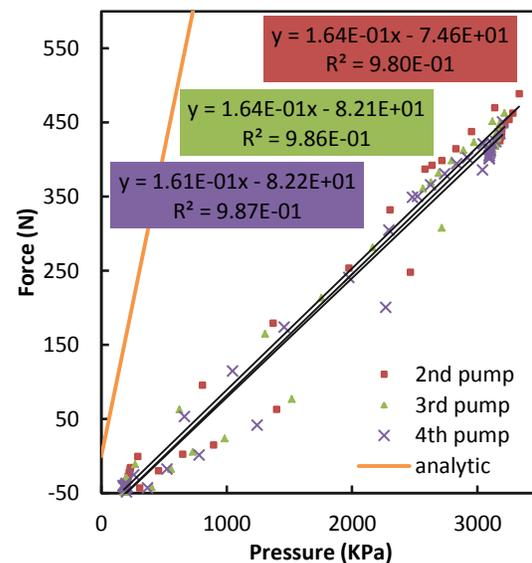
Figure 3-5: Bonded tube blocked force test #2. Figure 3-6: Bonded tube blocked force test #2.
