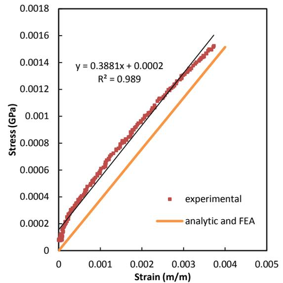
Figure 2-20: 52.5° bi-layer axial modulus.
