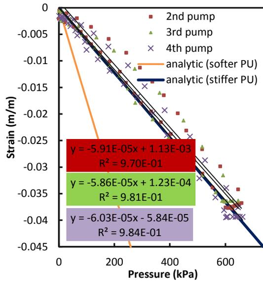
Figure B-10: Small braided tubes 24° free strain test B-1.
