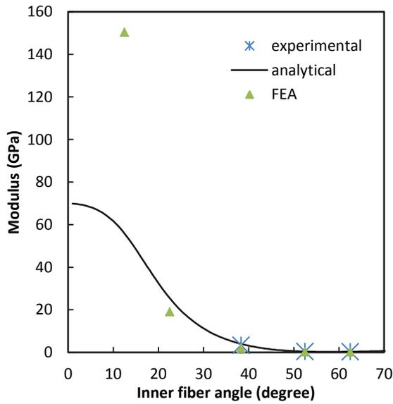
Figure 2-24: Axial modulus results.
