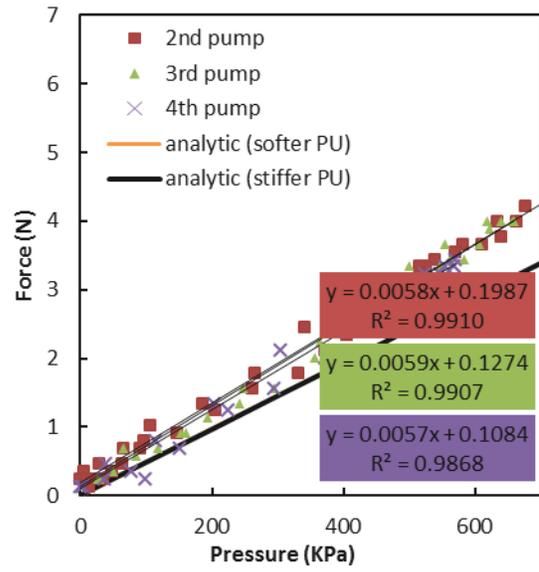
Figure B-20: Small braided tubes 40° blocked force test C-2.
