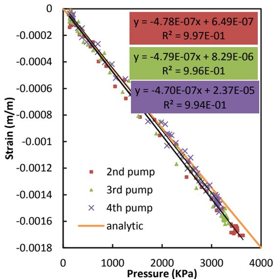
Figure 3-3: Bonded tube free strain test #1.
