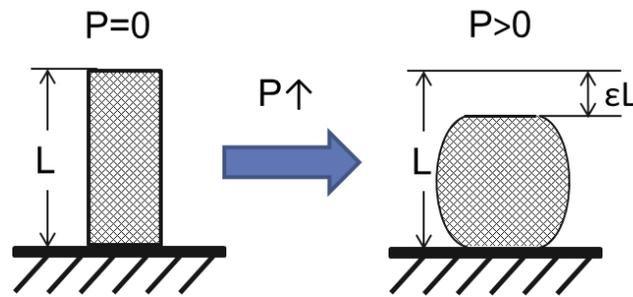
Figure 2-3: Free strain test diagram.
