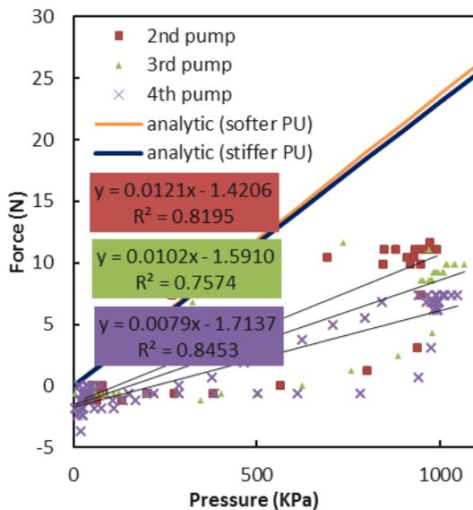
Figure 4-15: Small braided tubes 24° blocked force test A-1.
