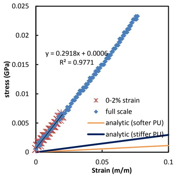
Figure B-24: Small braided tubes 40° axial modulus test A-4.
