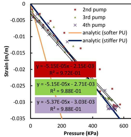
Figure B-2: Small braided tubes 24° Free strain test A-4.
