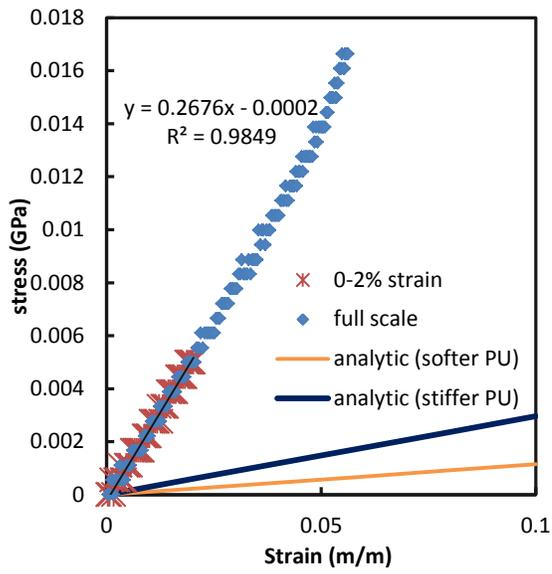
Figure B-22: Small braided tubes 40° axial modulus test A-2.
