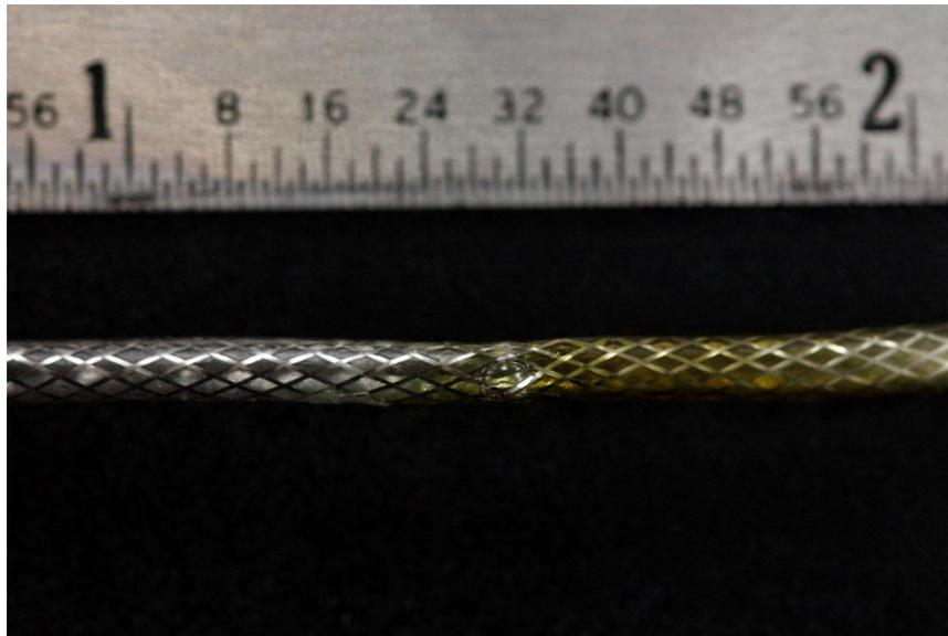
Figure 4-9: Photograph of a blown out braided tube.
