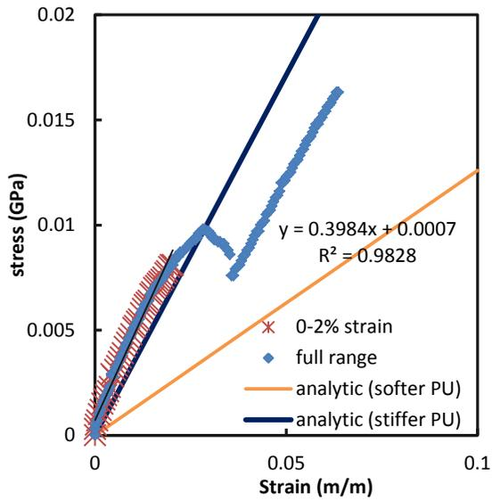
Figure **B-25**: Small braided tubes 24° axial modulus test C-1.
