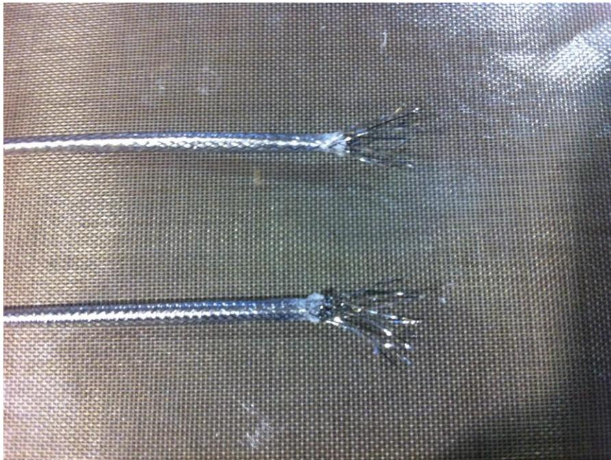
Figure 4-7: Photograph of polyurethane stripped from ends of braided tubes.
