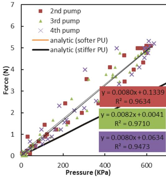
Figure B-19: Small braided tubes 40° blocked force test C-1.
