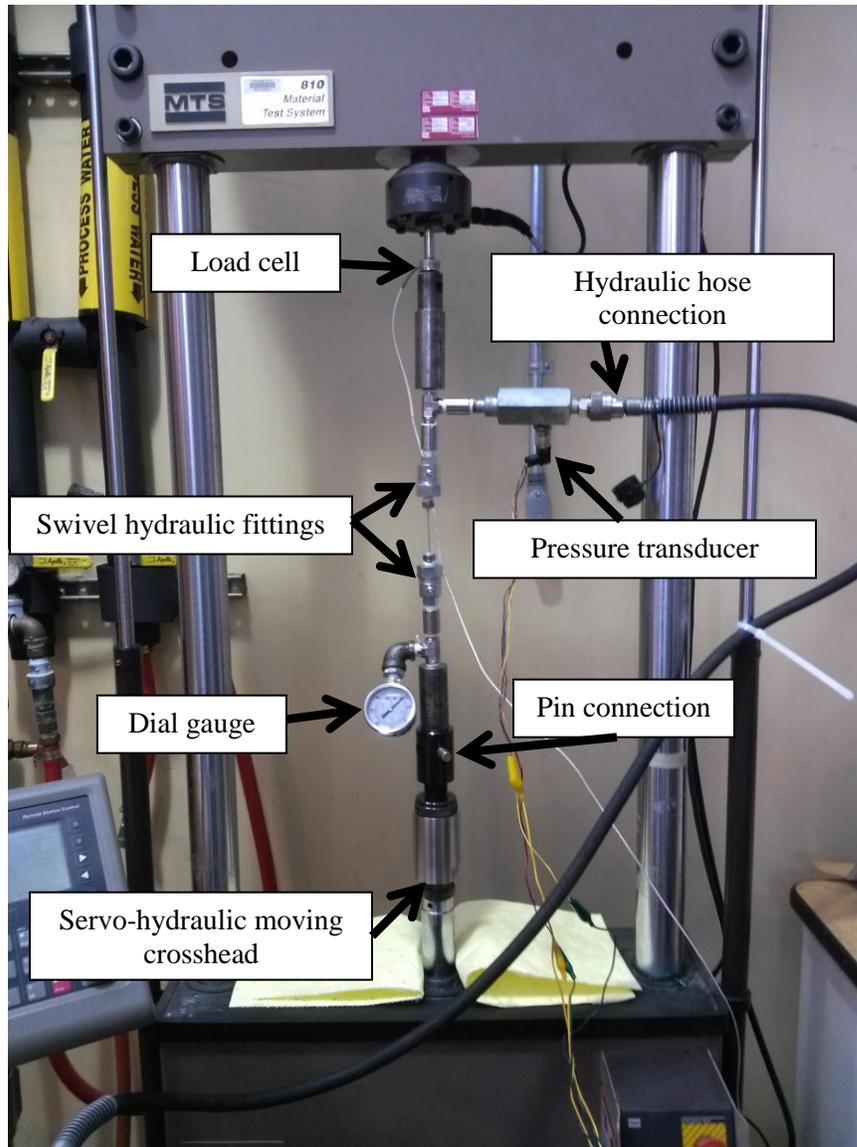
Figure 4-11: Blocked force and axial modulus test setup for braided tubes.
