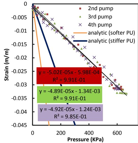
Figure B-12: Small braided tubes 40° free strain test C-2.
