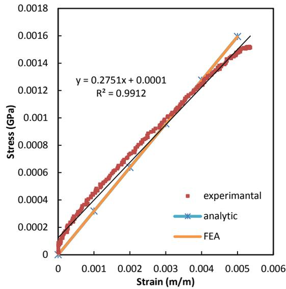
Figure 2-21: 62.5° bi-layer axial modulus.
