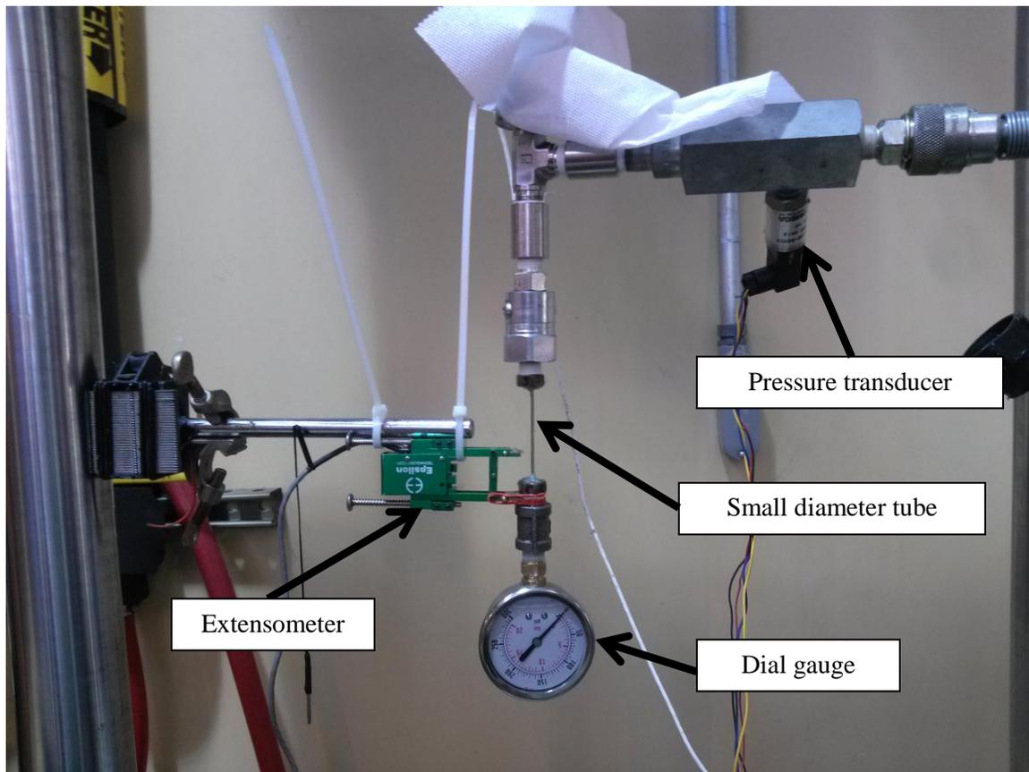
Figure 4-10: Free strain test setup for braided tubes.
