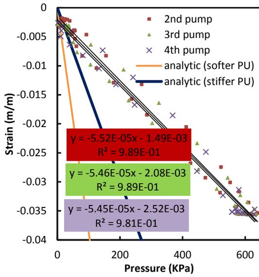
Figure B-3: Small braided tubes 40° free strain test A-1.
