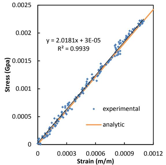
Figure 3-7: Bonded tube axial modulus test #1. Figure 3-8: Bonded tube axial modulus test #2.
