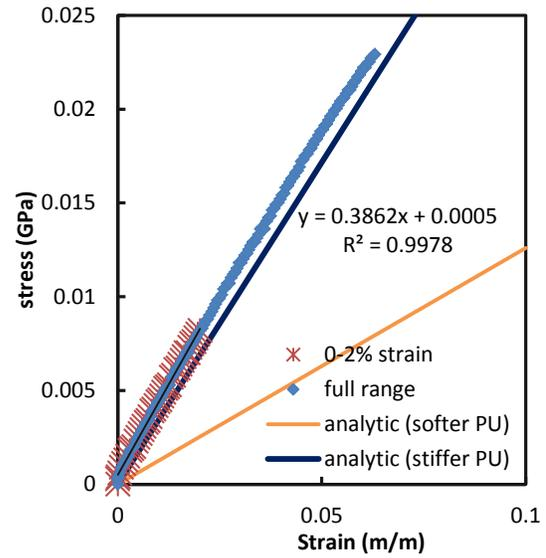
Figure **B-26**: Small braided tubes 24° axial modulus test C-2.
