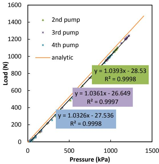
Figure 2-12: 35° thin-walled blocked force.
