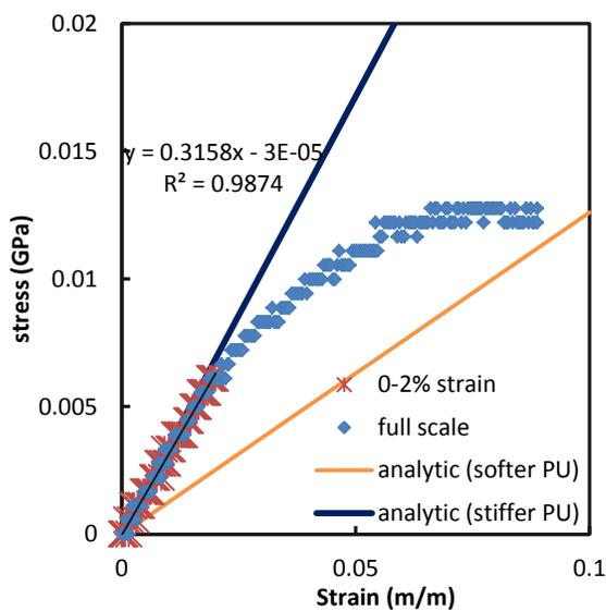
Figure 4-17: small braided tubes 24° axial modulus test A-3.
