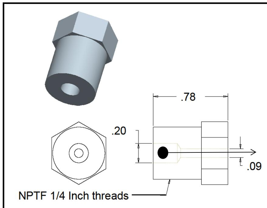
Figure 4-5: Diagram of steel plug used as an end fitting for the braided tubes.
