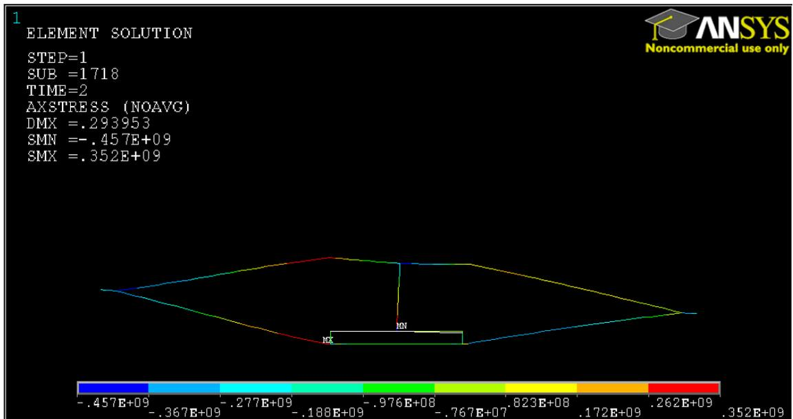
Figure D.6: Stress Distribution for Optimized Cell Deformed Using an Input Velocity of 30 microns/sec for 2 seconds where the Top Wall is not constrained
