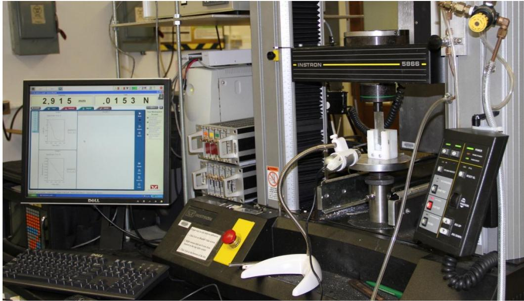
Figure 4.12: The complete test set-up including the test rig and the video camera.
