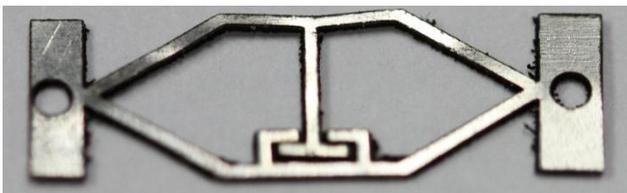
Figure 4.16: Deformed Cell After Compression Testing
