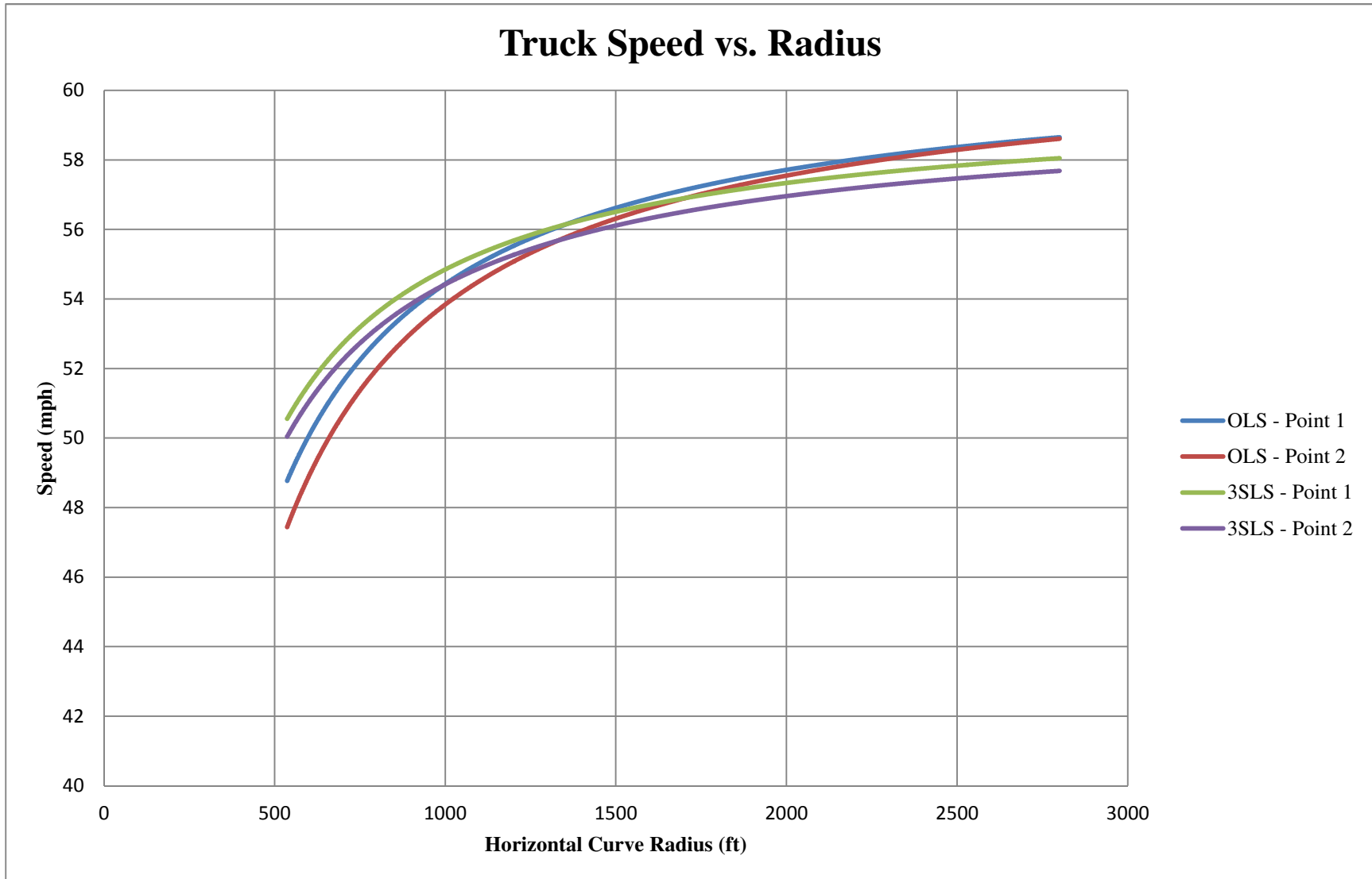
Figure 27 – Truck Speed Profile Plot of Horizontal Curve Radius for OLS and 3SLS models
