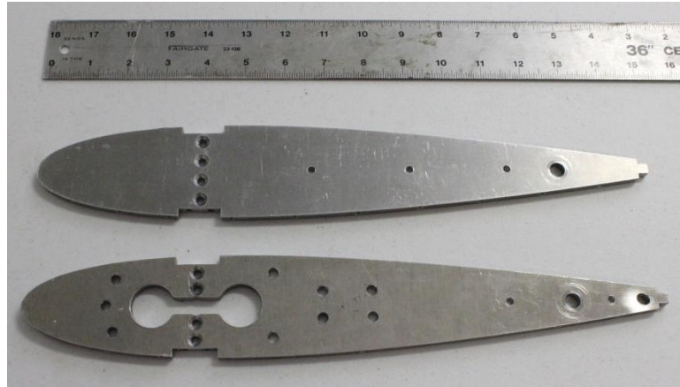
Figure 2-15: Outer (top) and inner (bottom) ribs of extendable chord system.
