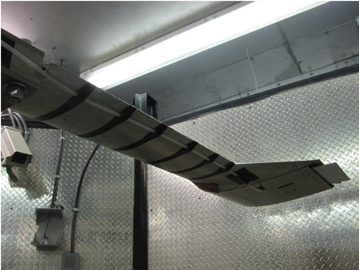
Figure 4-11: Pneumatically actuated extendable chord system installed in AERTS facility.
