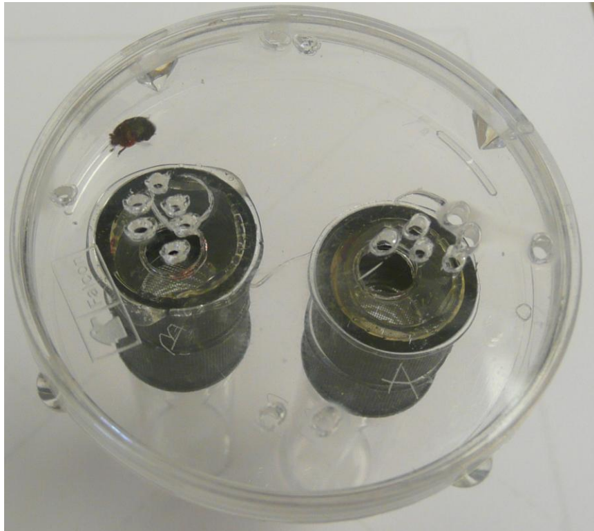
Figure 3-1: Still-air bioassay chamber for assessing adult small hive beetle preferences.
