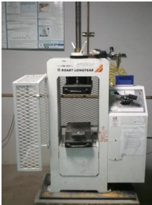
Figure 3-18: Boart Longyear model CM-625 with a CSI Model CS-100-2A Retrofit
