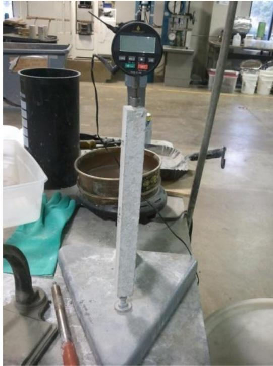
Figure 3-24: Humboldt model BG2600-16001 comparator with specimen loaded for measurement
