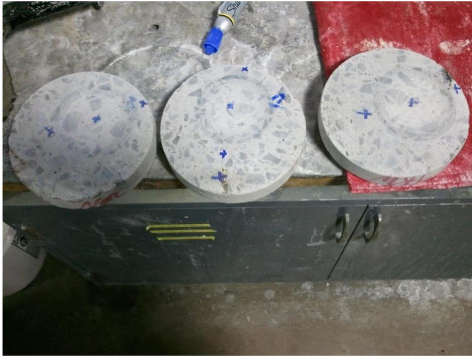
Figure 3-25: Abrasion resistance specimens
