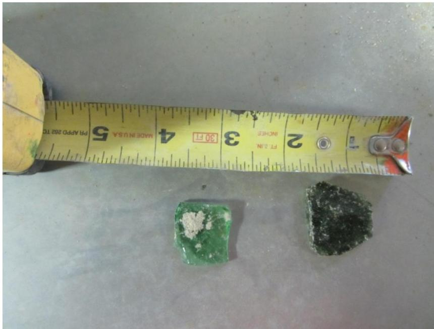
Figure 2-3: Coarse glass aggregate cullet
