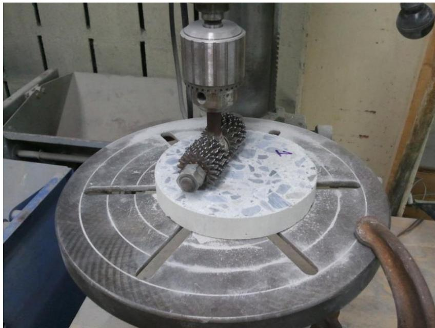
Figure 3-26: ASTM C 944 setup
