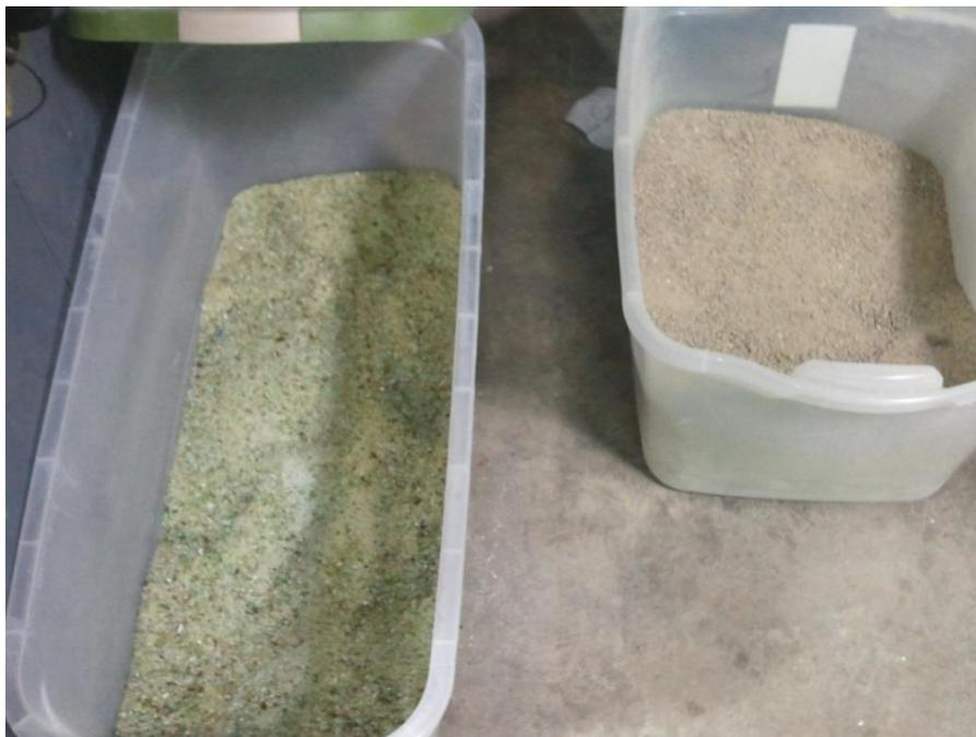
Figure 3-3: 3000 revolution glass sand (left) and natural river sand (right) as used in concrete production
