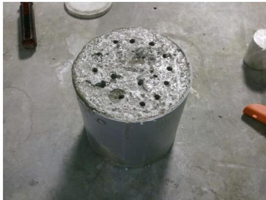
Figure 3-12: Typical mortar time of setting specimen after testing is complete
