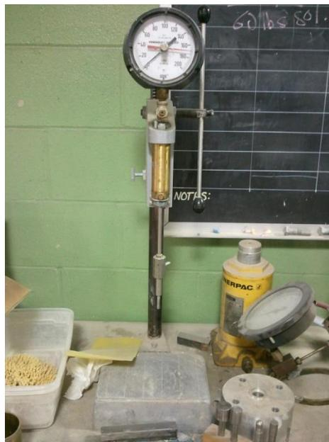
Figure 3-11: Humboldt H/4133 spring-reaction device used for time of setting measurements
