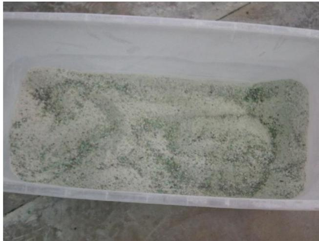
Figure 3-5: 1000 revolution glass sand used in production
