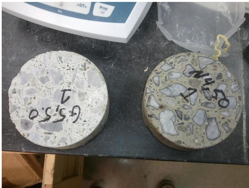
Figure 4-29: Coloration of concrete specimens after sorptivity testing
