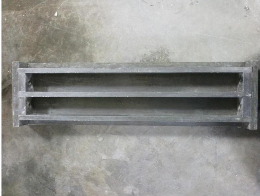
Figure 3-23: Mold used to cast COTE mortar bars
