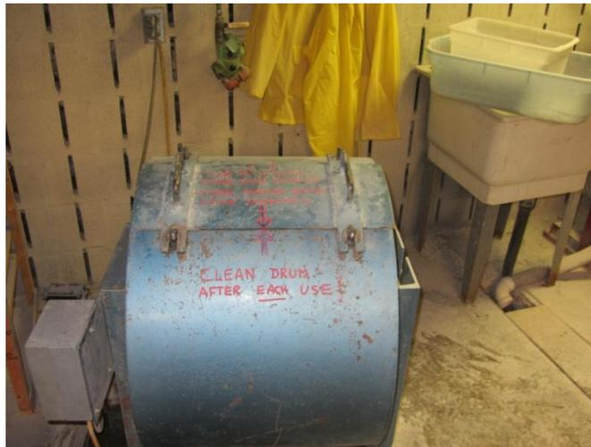
Figure 3-4: LA Abrasion Machine used to crush glass cullet to sand size
