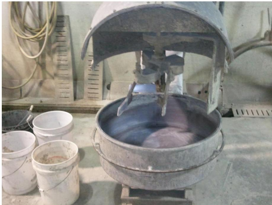
Figure 3-6: Eirich S-1 counter current concrete mixer
