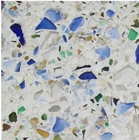
Figure 2-5: Decorative concrete with the top layer of paste removed shown with various waste glass cullet sizes
