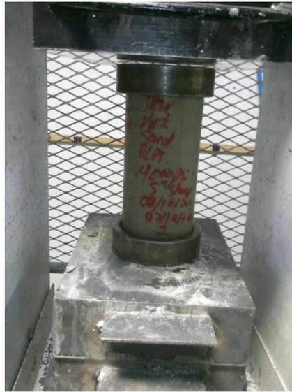
Figure 3-15: Sample concrete specimen prior to compressive strength testing
