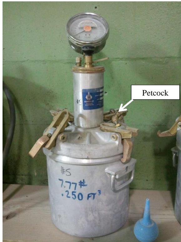
Figure 3-10: Type-B pressure meter used during study
