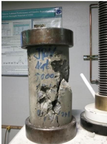
Figure 3-16: Sample concrete specimen post compressive strength testing
