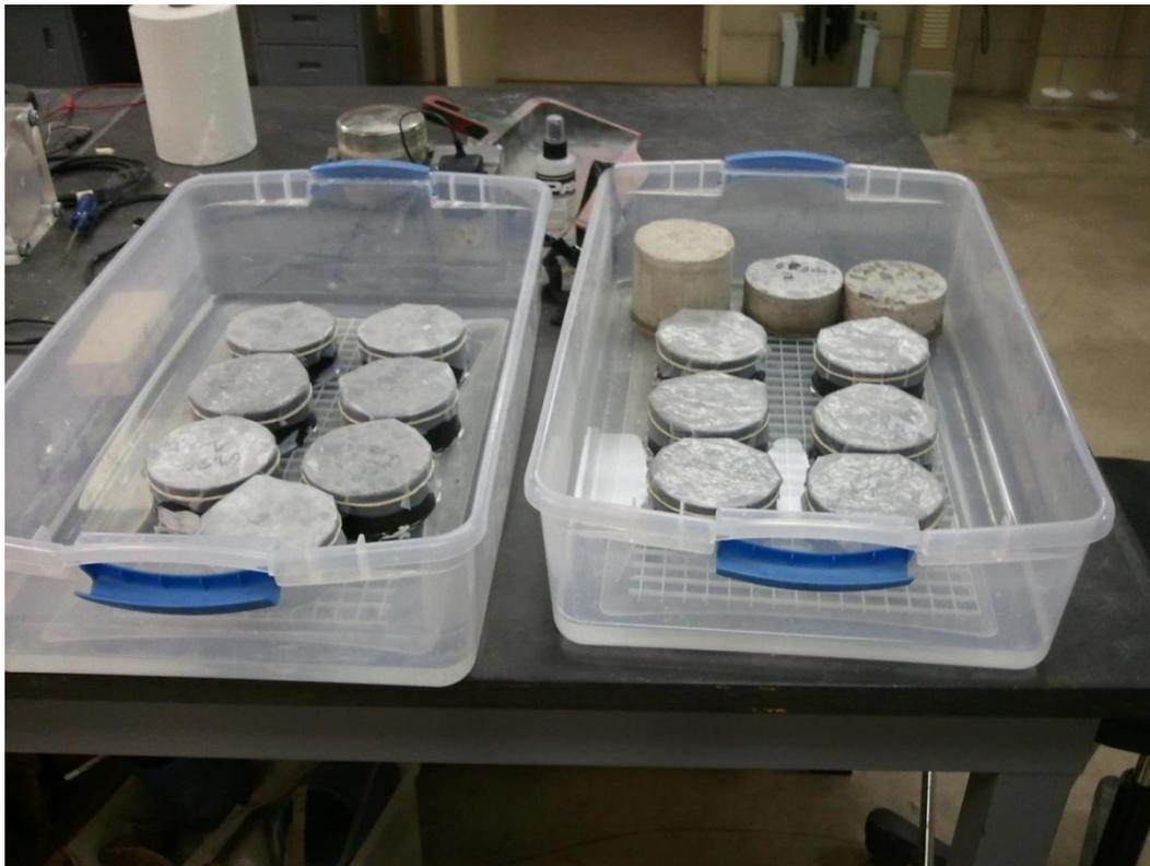
Figure 3-33: ASTM C 1585 water bath setup
