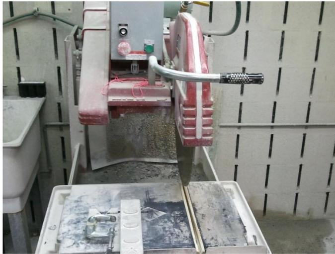
Figure 3-17: Wet saw used to smooth, even, and dimension concrete specimens
