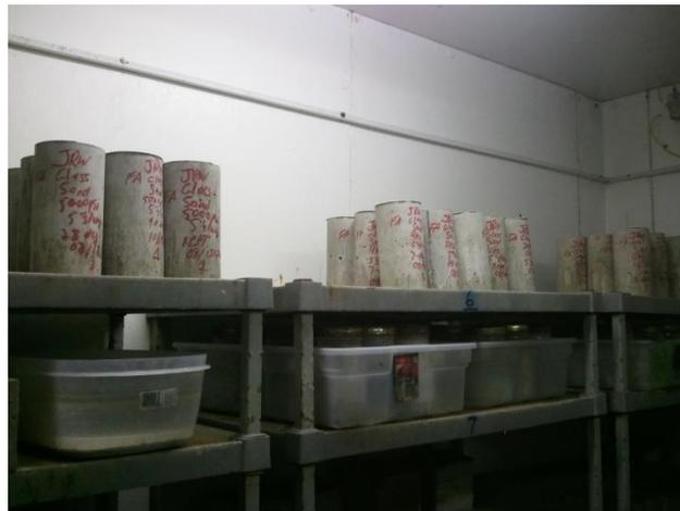
Figure 4-1: Glasscrete and concrete specimens during moist curing
