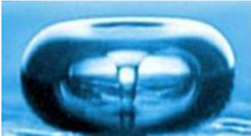
Figure 2-3: Image of implosion of cavitation void showing micro-jetting of fluid through the center of the bubble [25].
