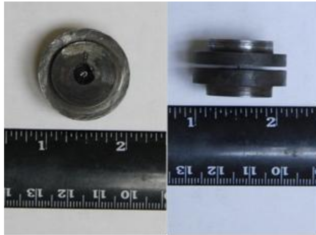
Figure 3-8: Top and side view of torsional DMA specimen bonded to its grips
